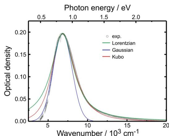
**Fig. S1.** Experimental absorption spectrum of the ammoniated electron (gray symbols) together with fits to difference line-shape functions (curves).
