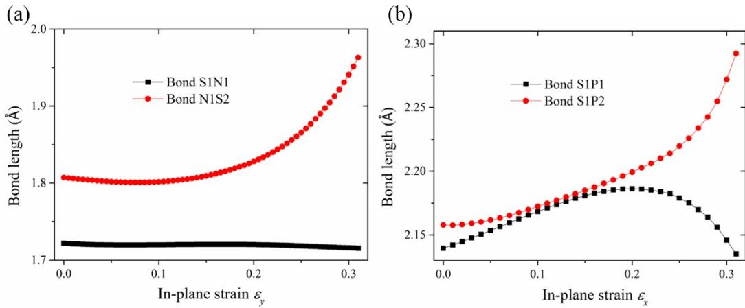
Figure S7 Bond length changes under tension (a) in  $y$  direction for  $\text{S}_3\text{N}_2$  and (b) in  $x$  direction for  $\text{S}_3\text{P}_2$ .
