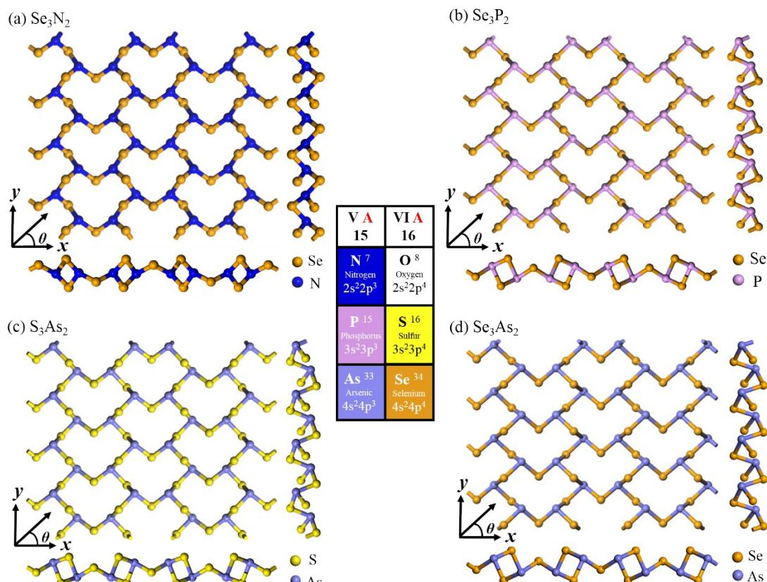
Figure S1 Atomic model of (a)  $Se_3N_2$  (b)  $Se_3P_2$  (c)  $S_3As_2$  and (d)  $Se_3As_2$ . The inset shows group V and VI elements considered in this study (colored).  $\theta$  defines the orientation relative to  $x$  axis.
