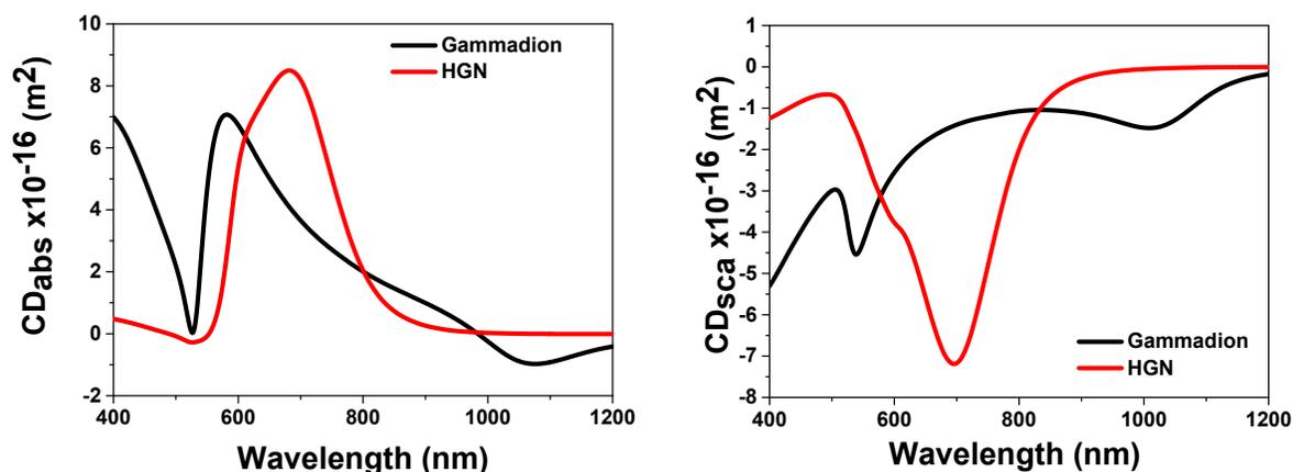
**Figure S7.** Comparison between the CD spectra obtained for a chiral HGN and gold gammadion; left:  $CD_{abs}$ , and right:  $CD_{sca}$ .
