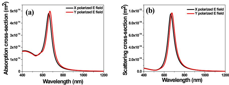
**Figure S2.** (a) Absorption spectra and (b) scattering spectra of free-standing HGN ( $L=150$  nm,  $T=40$  nm and cavity diameter 28 nm) excited by a plane wave having electric field along X (black lines) and Y (red lines) direction.
