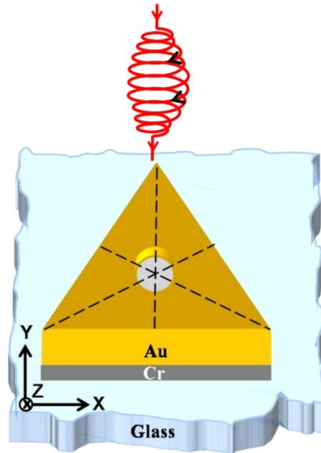
**Figure S1.** Schematic representation of the numerical simulation set up. An HGN, having 150 nm edge length, 40 nm thickness and 28nm cavity diameter is placed on a 4 nm thick Cr substrate which is already placed on a 20 nm thick glass. The whole system is excited either by linearly polarized (X or Y) or circularly polarized (LCP or RCP) light coming from the +ve Z-direction.
