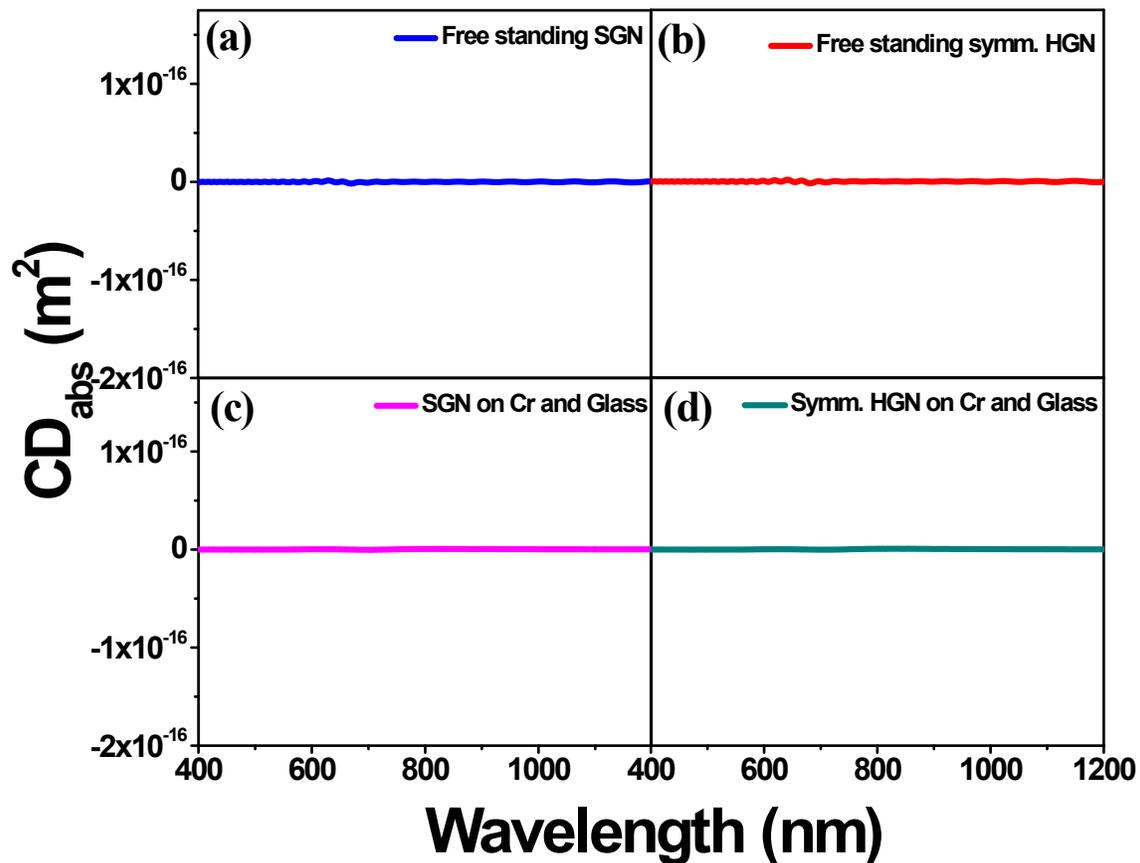
**Figure S3.**  $CD_{abs}$  spectra for (a) free-standing SGN, (b) free-standing symmetrical HGN, (c) SGN on glass and Cr and (d) symmetrical HGN on glass and Cr. Both the SGN and HGN have same edge length (150 nm) and thickness (40 nm). The symmetrical HGN has a cavity (diameter 28nm) at its centroid.
