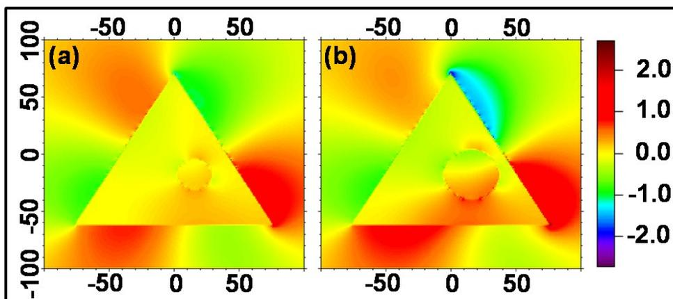
**Figure S5.** Differential electric field distribution ( $|E_{RCP}| - |E_{LCP}|$ ) of a chiral HGN ( $L = 150\text{nm}$ ,  $T = 40\text{nm}$  and  $16\text{nm}$  offset) of having cavity of (a)  $28\text{nm}$  and (b)  $44\text{nm}$  diameter.
