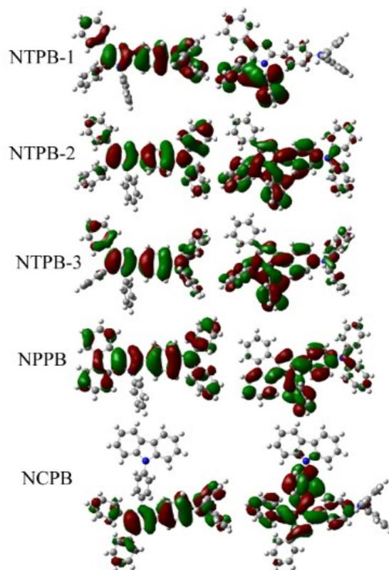
Figure S20. Molecular orbital plots of the HUMOs and LUMOs of NTPB, NPPB and NCPB.
