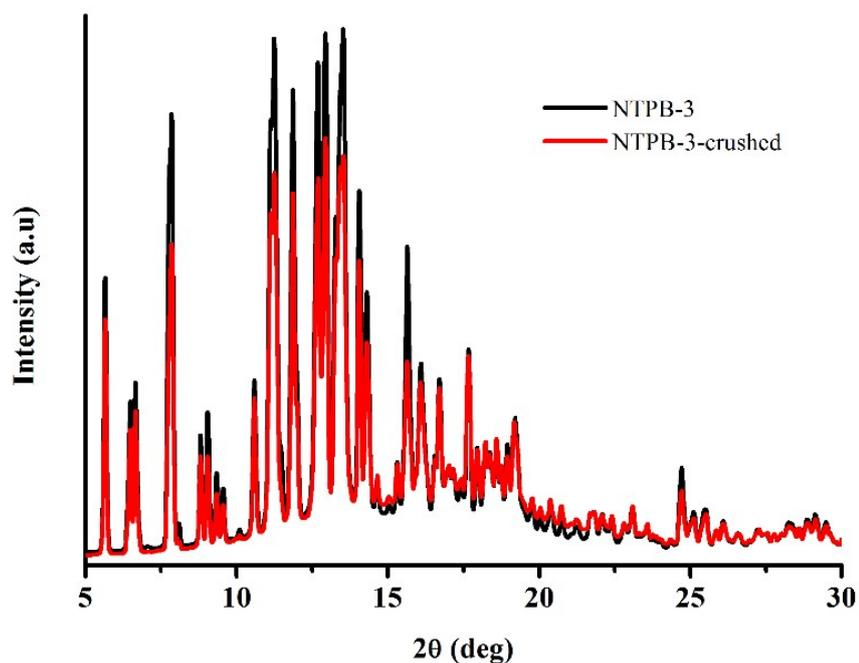
Figure S19. PXRD pattern of NTPB-3 before and after crushing.
