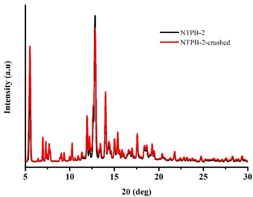
Figure S18. PXRD pattern of NTPB-2 before and after crushing.
