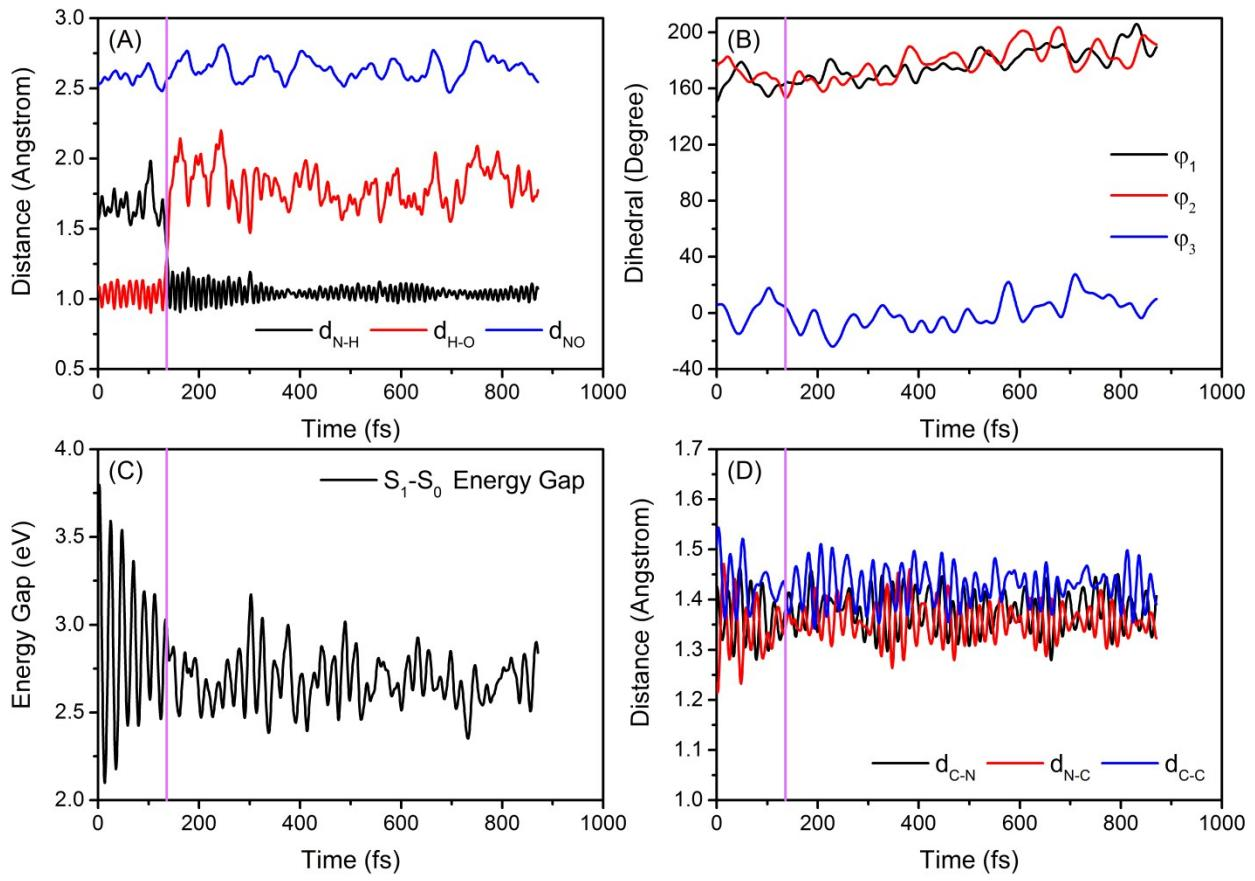
**Fig. S4.** Different properties vs. simulation time of a typical trajectory for (IIA)S<sub>1</sub> in acetonitrile solution. a) N–H, O–H and NO distances, b)  $\varphi_1$ ,  $\varphi_2$  and  $\varphi_3$  dihedral angles, c) S<sub>1</sub>/S<sub>0</sub> energy gap and d) C<sub>1</sub>–N, N–C<sub>3</sub> and C<sub>3</sub>–C<sub>4</sub> distances. The vertical lines indicate the ESIPT event.
