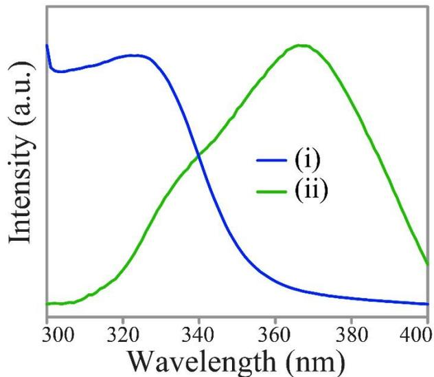
**Figure S7.** Photoluminescence excitation spectra of (i) as synthesized ZnS Qdots ( $\lambda_{em}= 440$  nm) in aqueous solution and (ii) QDC ( $\lambda_{em}= 500$  nm) in DMSO.
