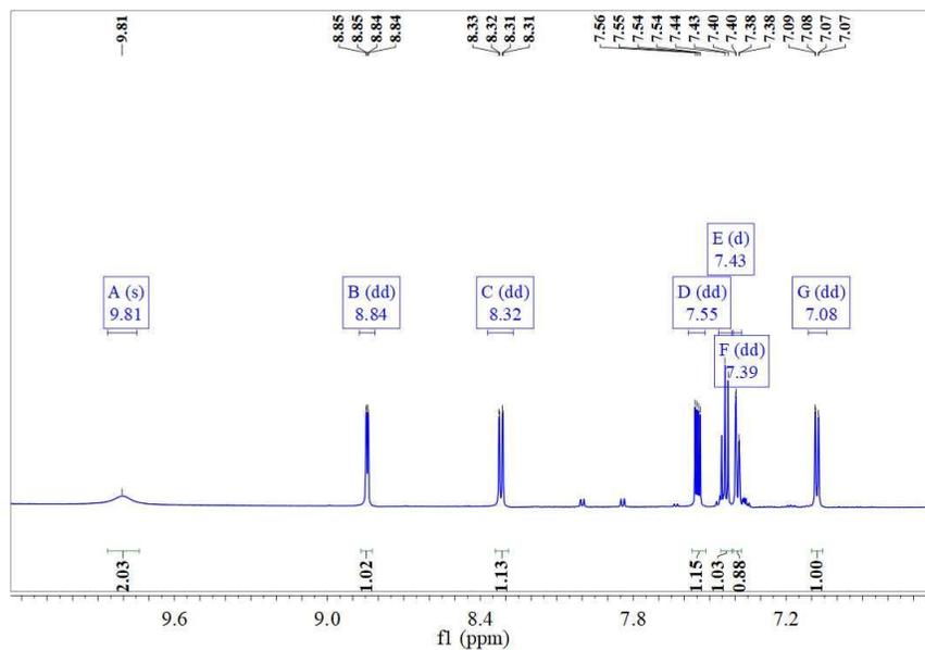
**Figure S9.** Proton NMR spectrum of 8-hydroxyquinoline (HQ).  $^1\text{H}$  NMR (600 MHz, DMSO)  $\delta$  9.81 (s, 1H), 8.84 (dd,  $J = 4.1, 1.6$  Hz, 1H), 8.32 (dd,  $J = 8.3, 1.6$  Hz, 1H), 7.55 (dd,  $J = 8.3, 4.1$  Hz, 1H), 7.43 (d,  $J = 7.6$  Hz, 1H), 7.39 (dd,  $J = 8.2, 1.2$  Hz, 1H), 7.08 (dd,  $J = 7.5, 1.3$  Hz, 1H).
