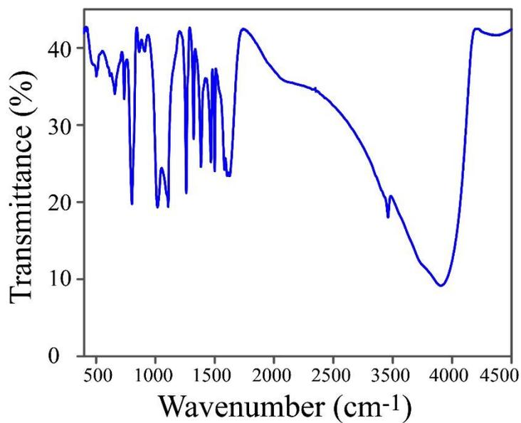
**Figure S8.** Fourier transform infrared (FTIR) spectrum of the solid sample (KBr pellet) of ZnS-Q QDC.
