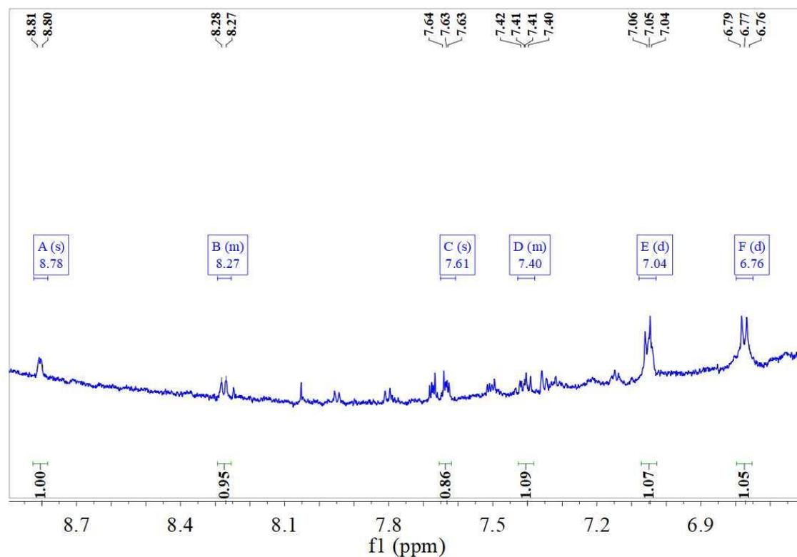
**Figure S11.** Proton NMR spectrum of supernatant obtained after centrifugation of as prepared ZnS-HQ QDC.  $^1\text{H}$  NMR (600 MHz, DMSO)  $\delta$  8.78 (s, 1H), 8.29 – 8.25 (m, 1H), 7.61 (s, 1H), 7.43 – 7.38 (m, 1H), 7.04 (d,  $J$  = 15.2 Hz, 1H), 6.76 (d,  $J$  = 13.5 Hz, 1H).
