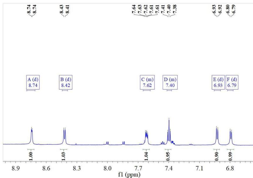
**Figure S10.** Proton NMR spectrum of  $\text{ZnQ}_2$ .  $^1\text{H}$  NMR (600 MHz, DMSO)  $\delta$  8.74 (d,  $J = 3.7$  Hz, 1H), 8.42 (d,  $J = 8.1$  Hz, 1H), 7.65 – 7.58 (m, 1H), 7.42 – 7.37 (m, 1H), 6.93 (d,  $J = 7.9$  Hz, 1H), 6.79 (d,  $J = 7.7$  Hz, 1H).
