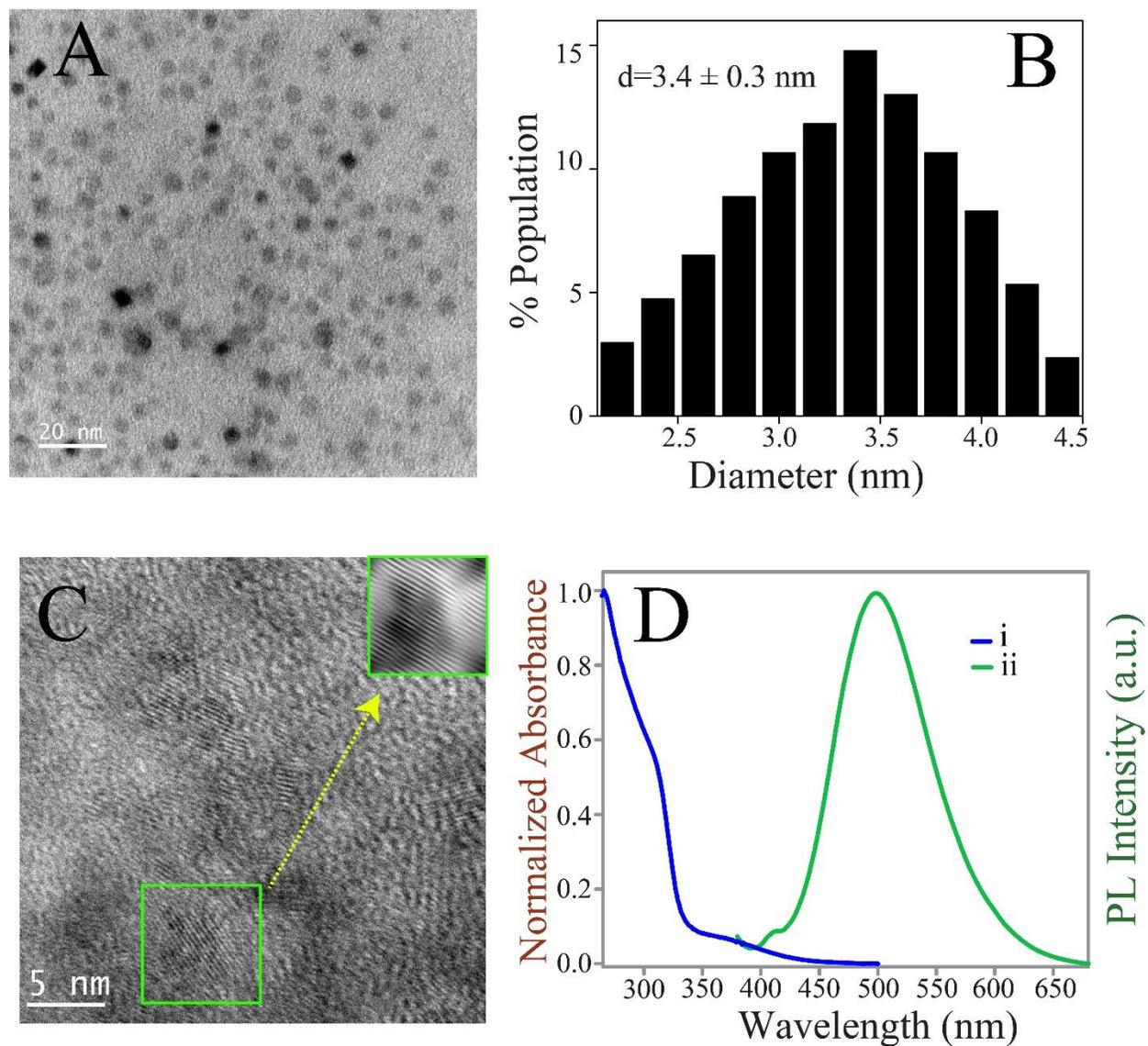
**Figure S6.** (A) Transmission electron microscopic (TEM) image (scale bar- 10 nm) and (B) corresponding particle size distribution, (C) high resolution TEM image (scale bar - 5 nm) and corresponding inverse fast Fourier transform (IFFT) image (inset) and (D) UV-vis and emission spectrum ( $\lambda_{\text{ex}}$ -365 nm) of QDC (in DMSO).
