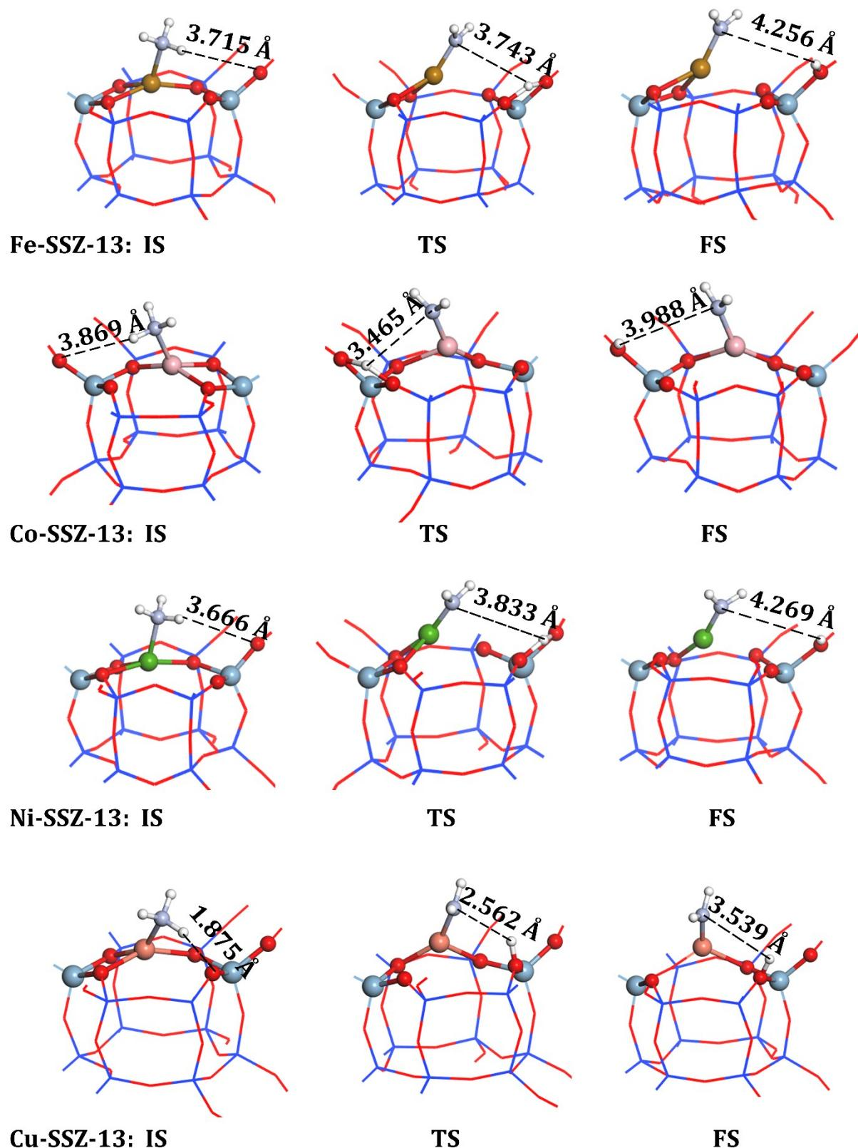
**Fig. S7** Calculated structures of the initial, final, and transition states for  $\text{NH}_3$  activation in Fe, Co, Ni, Cu-SSZ-13.
