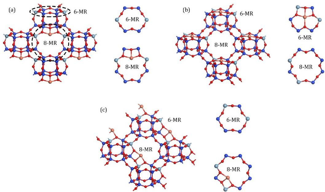
**Fig. S1** The structure schematic diagrams and corresponding 2-dimensional views of 6-MR and 8-MR (a) TM-pAl2-8MR (b) TM-mAl2-6MR (c) TM-mAl2-8MR
