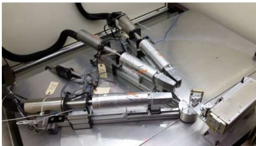
Fig. S1 – Photograph of the last prototype of EDXD diffractometer, with three detectors placed at three fixed angles
