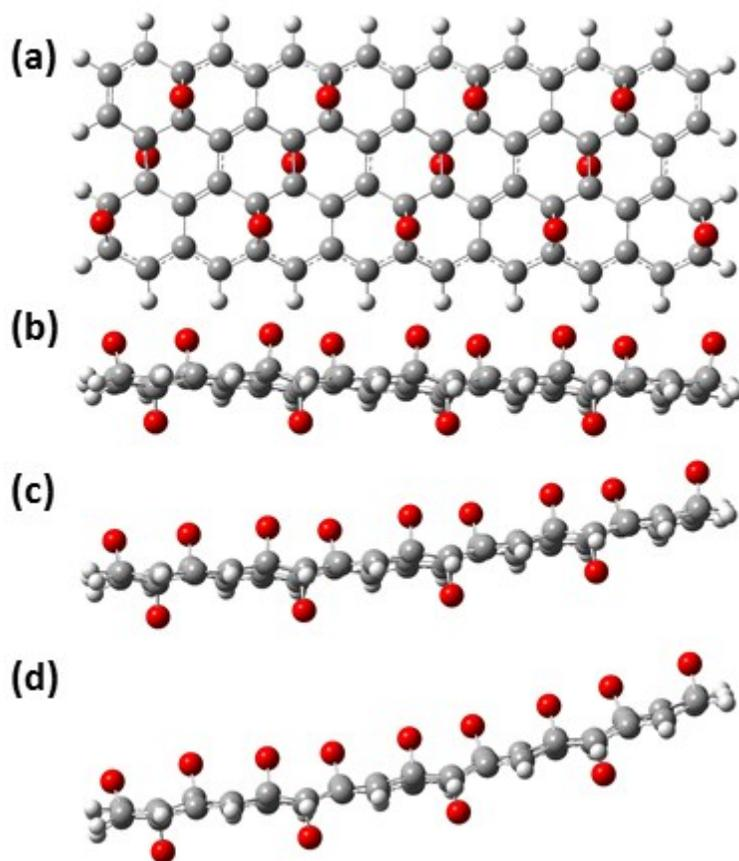
**Figure S2:** Top (a) and side (b) views of optimized GO nanoribbon with zigzag edge and 50% epoxy coverage, as well as side views of its constrained optimization results with bent right edge to accommodate one (c) and two (d) water molecules.
