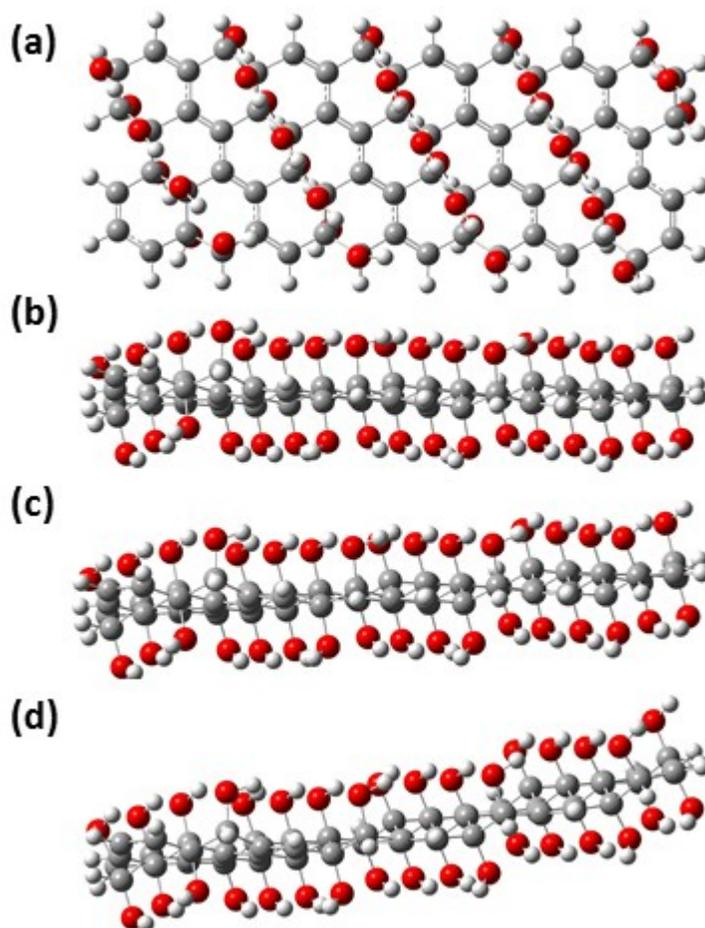
**Figure S3:** Top (a) and side (b) views of optimized GO nanoribbon with zigzag edge and 50% hydroxyl coverage, as well as side views of its constrained optimization results with bent right edge to accommodate one (c) and two (d) water molecules.
