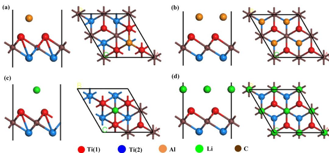
**Fig. S9** The structure of a single atom or a layer of atoms adsorbed on the surface of Ti<sub>2</sub>C surface.
