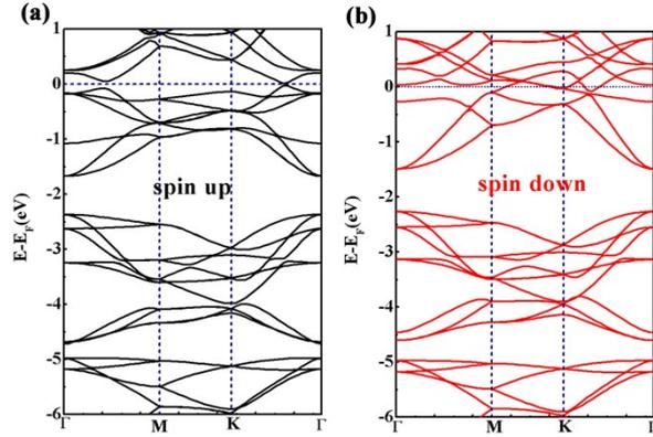
**Fig. S5** The band-structure of  $\text{Ti}_2\text{C-OH}$  monolayer. (a) spin up; (b) spin down.
