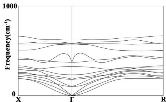
**Fig. S8** Phonon dispersion curves of the asymmetrically Li-Ti<sub>2</sub>C-O monolayer.
