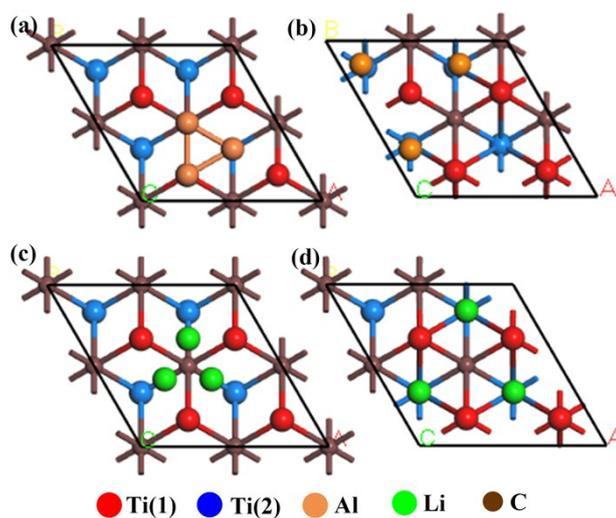
**Fig. S10** The structures before and after optimization of the metal clusters on the surface of Ti<sub>2</sub>C monolayer. (a)unrelaxed (b)relaxed structures of Ti<sub>2</sub>C-Al clusters; (c)unrelaxed (d)relaxed structures of Ti<sub>2</sub>C-Li clusters.
