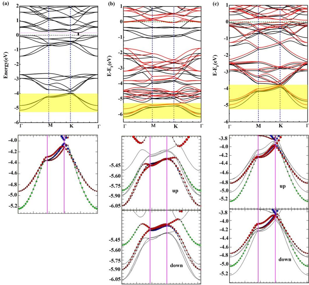
**Fig. S3** The band structure for  $\text{Ti}_2\text{C}$ (a),  $\text{Ti}_2\text{CO}$ (b),  $\text{Ti}_2\text{CLi}$ (c), where the red, blue and green circle represent the band composed of  $3d_{xy}$ ,  $3d_{x^2-y^2}$ ,  $3d_{xz}$ ,  $3d_{yz}$  and  $3d_z^2$ .
