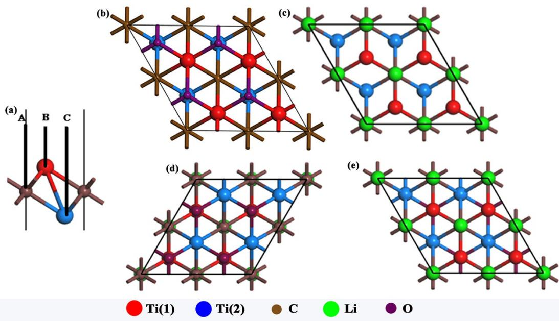
**Fig. S1** The structure of pristine Ti<sub>2</sub>C monolayer and functional Ti<sub>2</sub>C monolayer. (a) side view of the unitcell of Ti<sub>2</sub>C monolayer, where A, B, C represent the possible adsorption site of functional groups; (b) (c) the top view of 2×2 supercell of Ti<sub>2</sub>C-O and Ti<sub>2</sub>C-Li monolayer; (d) (e) the bottom and top viewer of Ti<sub>2</sub>C-LiO monolayer.
