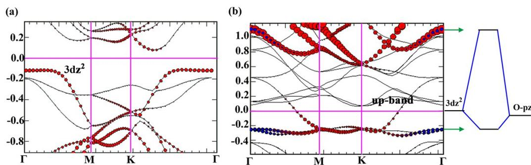
**Fig. S2** The orbital energy level diagram of (a)Ti<sub>2</sub>C monolayer, (b) the spin-up channel of Ti<sub>2</sub>C-O monolayer, where the red circle represents the contribution of  $3d_{z^2}$  orbitals of Ti atoms and the blue circle represents the contribution from  $p_z$  orbitals of O atoms.
