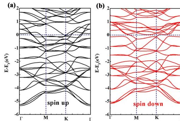
**Fig. S4** The band-structure of  $\text{Ti}_2\text{C-P}$  monolayer. (a) spin up; (b) spin down.
