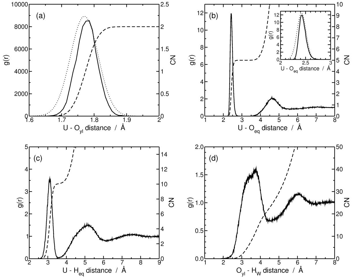
**Fig. S2** Radial distribution functions (solid line) and corresponding coordination numbers (dashed line) calculated for (a)  $U - O_{\text{eq}}$ , (b)  $U - H_{\text{eq}}$ , (c)  $U - O_{\text{yl}}$ , and (d)  $O_{\text{yl}} - H_{\text{w}}$ . Theoretical radial distribution functions calculated from the experimental metrical parameters are also plotted (dashed dotted line).
