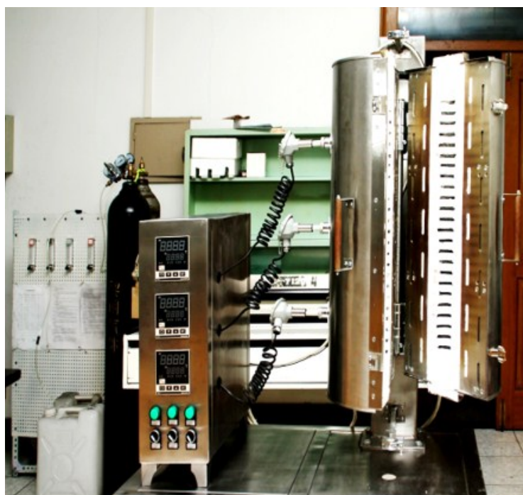
Fig. S5 The picture of self-made fixed bed adsorption system.
