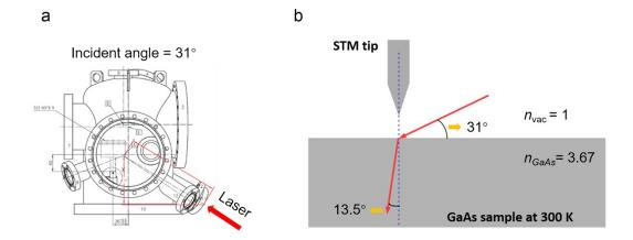
**Fig S4**. (a) Experimental setup. Both OPP-STM and OPPR measurements were conducted using an STM UHV chamber, at a fixed laser incident angle of ~31°. (b) Schematic illustration of the geometry of the oblique incidence light and the refracted light that penetrates into the sample, which determines the optical penetration depth.
