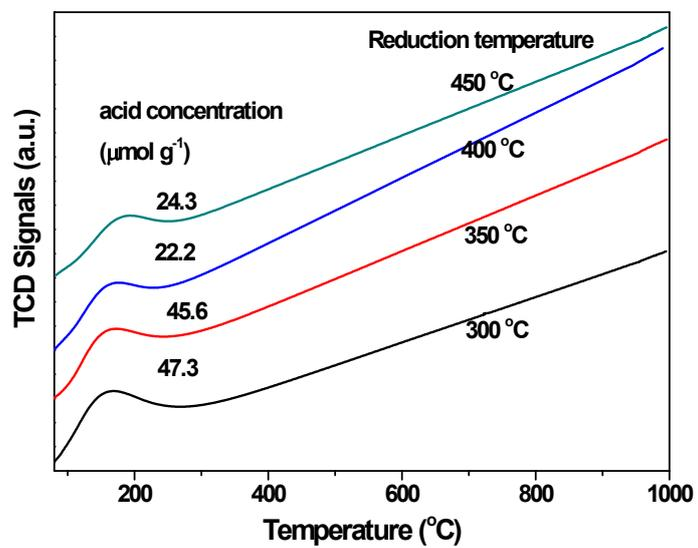
**Fig. S6.** NH<sub>3</sub>-TPD curves of Cu<sub>8</sub>-Mg<sub>1</sub>-Zr<sub>0.47</sub>/SiO<sub>2</sub> catalyst after reduced at different temperatures.
