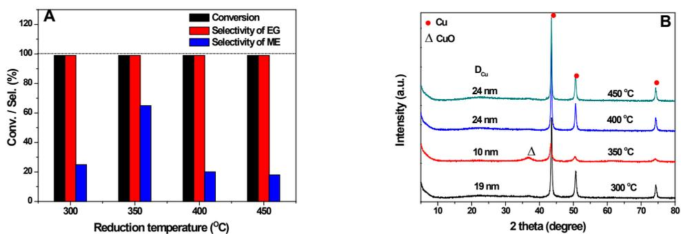
**Fig. S5.** (A) The conversion of EC, the selectivity to EG and ME versus Cu<sub>8</sub>-Mg<sub>1</sub>-Zr<sub>0.47</sub>/SiO<sub>2</sub> catalyst reduction temperature. The reaction parameters are identical with those for Fig. S2 except that the catalyst precursor was reduced at different temperatures. (B) XRD patterns of Cu<sub>8</sub>-Mg<sub>1</sub>-Zr<sub>0.47</sub>/SiO<sub>2</sub> catalysts after reduced at different temperatures.
