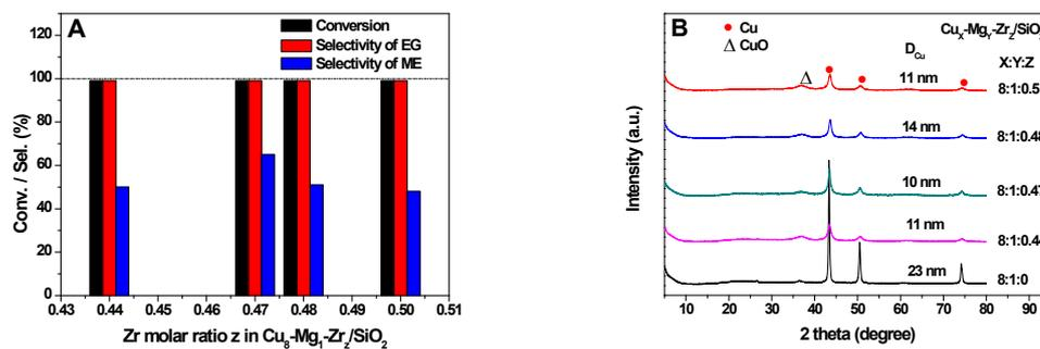
**Fig. S3.** (A) The conversion of EC, the selectivity to EG and ME with  $\text{Cu}_8\text{-Mg}_1\text{-Zr}_z\text{/SiO}_2$  catalysts, the reaction conditions are identical with those for Fig. S2. (B) The XRD patterns of the  $\text{Cu}_8\text{-Mg}_1\text{-Zr}_z\text{/SiO}_2$  catalysts.
