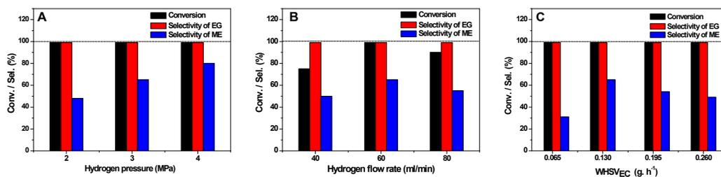
**Fig. S8.** (A) The conversion of EC, the selectivity to EG and ME versus hydrogen pressure; (B) effect of hydrogen flow rate on the conversion of EC, the selectivity to ME and EG; (C) The conversion of EC, the selectivity to ME and EG versus  $WHSV_{EC}$ . Other reaction parameters are identical with those for Fig. S2.
