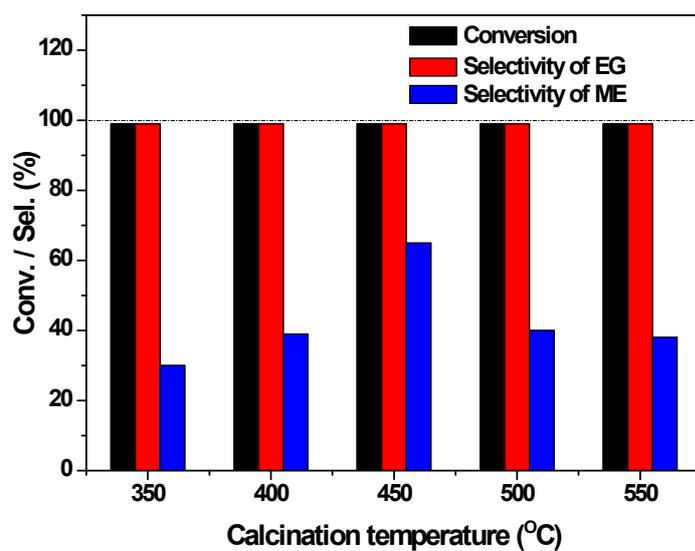
**Fig. S4.** The conversion of EC, the selectivity to EG and ME versus  $\text{Cu}_8\text{-Mg}_1\text{-Zr}_{0.47}/\text{SiO}_2$  catalyst precursor calcination temperature. The reaction parameters are identical with those for Fig. S2 except that the catalyst precursor was calcined at different temperatures.
