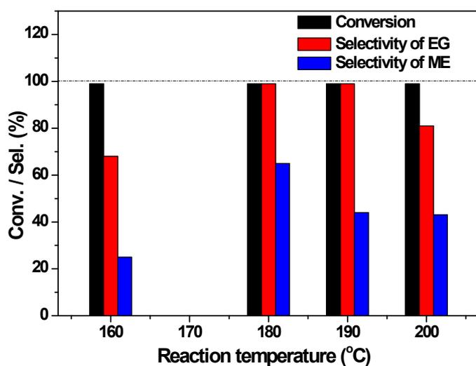
**Fig. S7.** The conversion of EC, the selectivity to EG and ME versus reaction temperature with  $\text{Cu}_8\text{-Mg}_1\text{-Zr}_{0.47}/\text{SiO}_2$  catalyst. The reaction parameters are identical with those for Fig. S2 except that the reaction was conducted at different temperatures.
