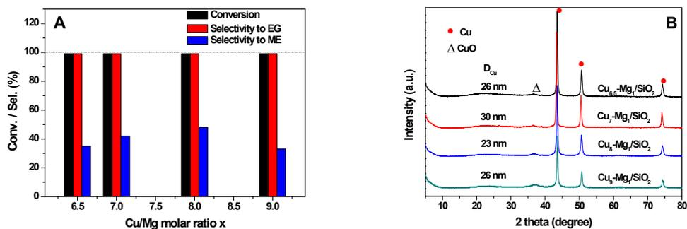
**Fig. S2.** (A) The conversion of EC, the selectivity to EG and ME with  $Cu_x$ - $Mg_1/SiO_2$  catalysts. Reaction conditions: the reaction conditions are identical with those for Fig. S1 except that 3 MPa of  $H_2$  was adopted. (B) The XRD patterns of the  $Cu_x$ - $Mg_1/SiO_2$  catalysts.
