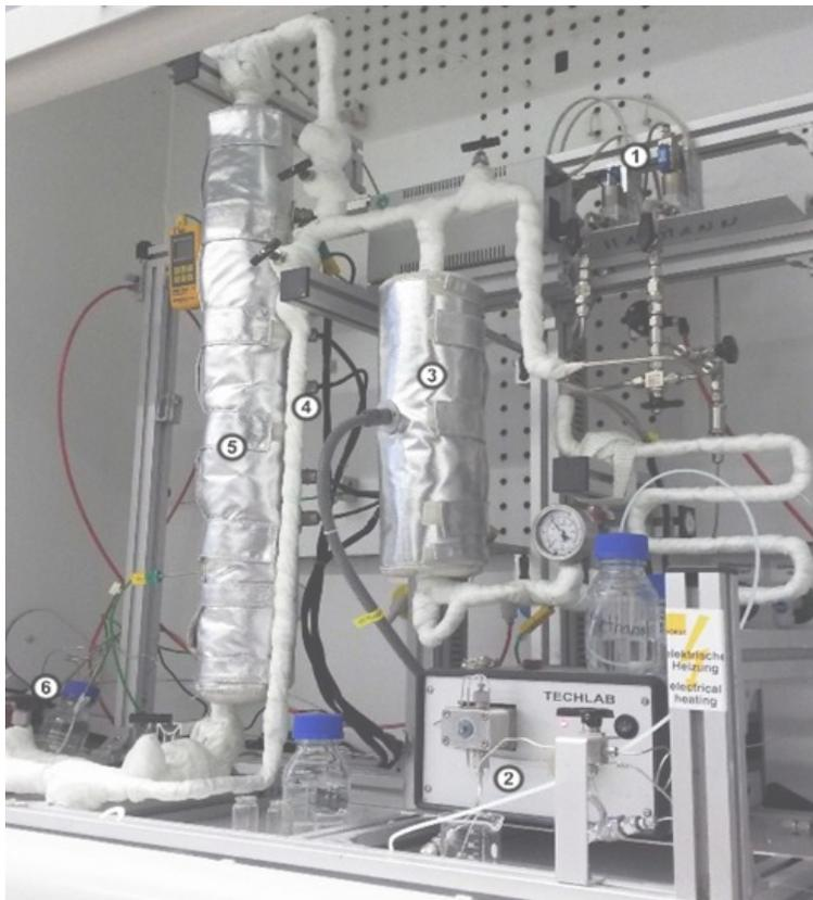
Figure S1. Picture of the continuous gas-phase reactor for e-SILP catalyzed transesterification. (1) Carrier gas dosing, (2) liquid dosing, (3) saturator, (4) bypass, (5) reactor, (6) back-pressure
