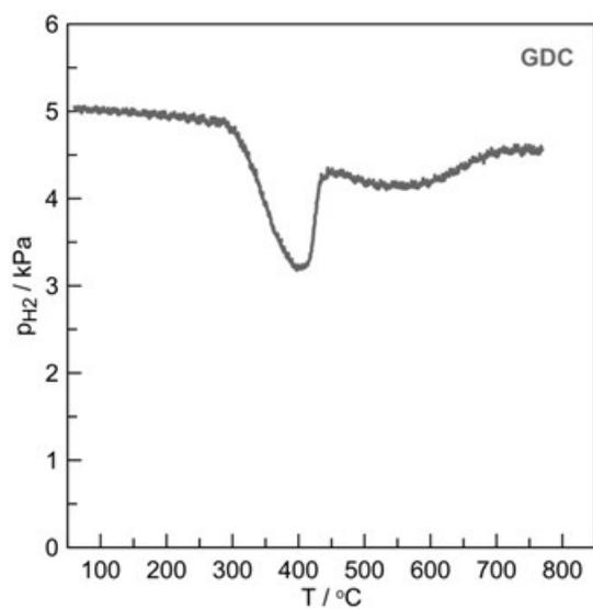
**Figure 1S.** Hydrogen concentration profile as a function of temperature during TPR experiment on GDC.
