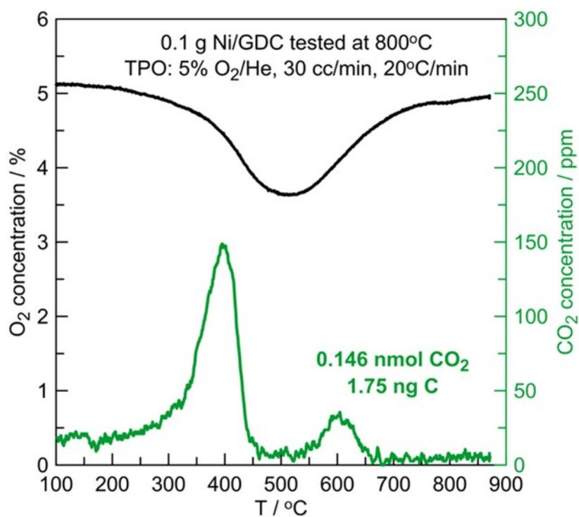
**Figure 2S.** Consumption of oxygen and production of CO<sub>2</sub> as a function of temperature during TPO experiment on Ni/GDC previously tested for methane steam reforming at 800°C.
