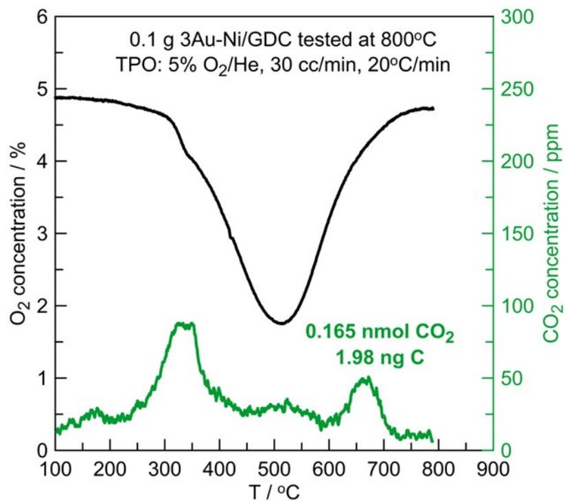
**Figure 3S.** Consumption of oxygen and production of CO<sub>2</sub> as a function of temperature during TPO experiment on Ni-Au/GDC previously tested for methane steam reforming at 800°C.
