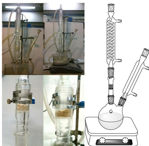
**Figure S1** Schematic representation of the reactive vapor adsorption system (RVA) with the selective adsorption of methanol inside molecular sieves.
