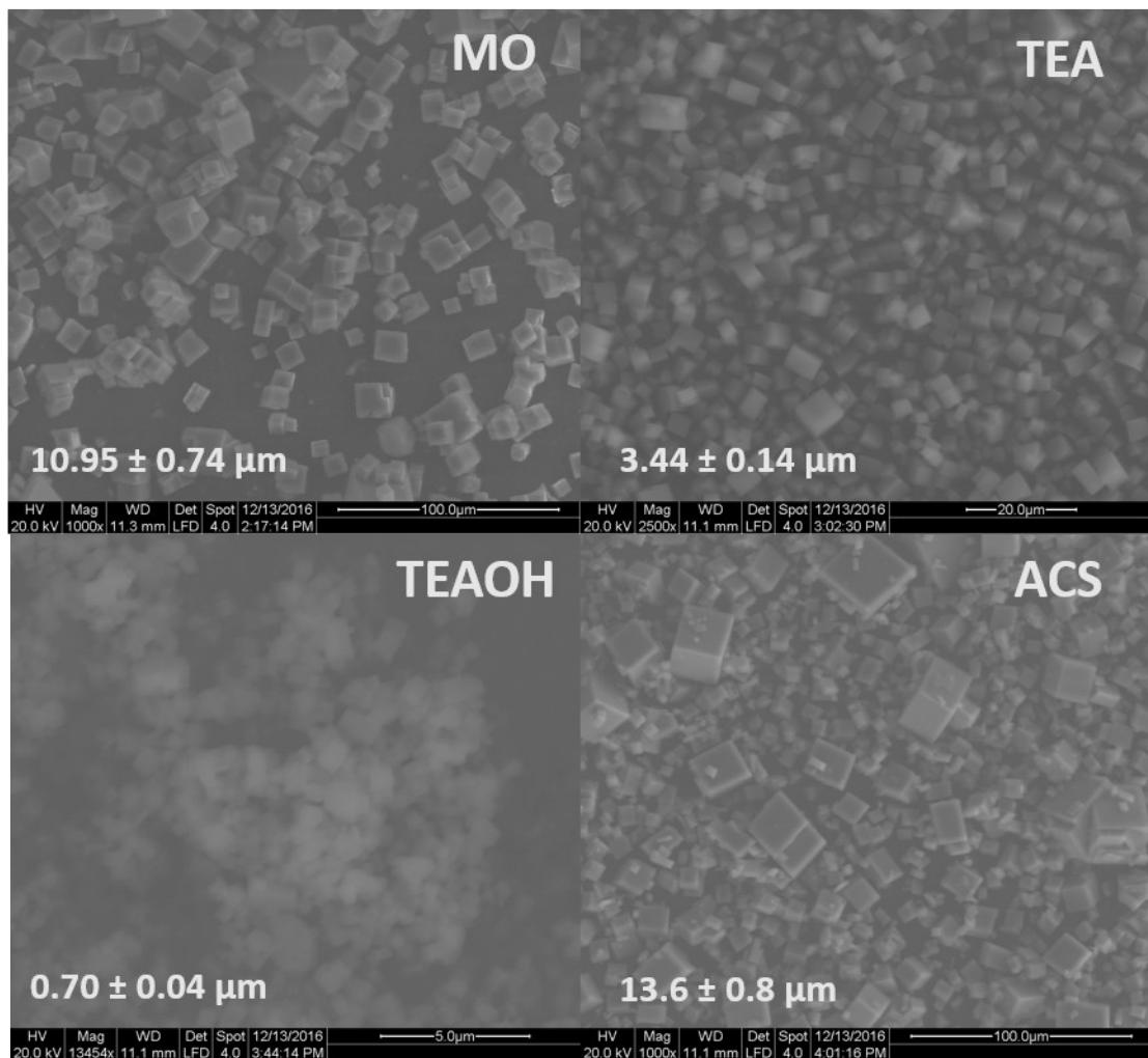
**Figure S1.** SEM image of SAPO-34(MO, TEA, TEAOH, and ACS) and their \*average particle size. \*Size of representative 100 particles were measured, and 95 % confidence interval was calculated.
