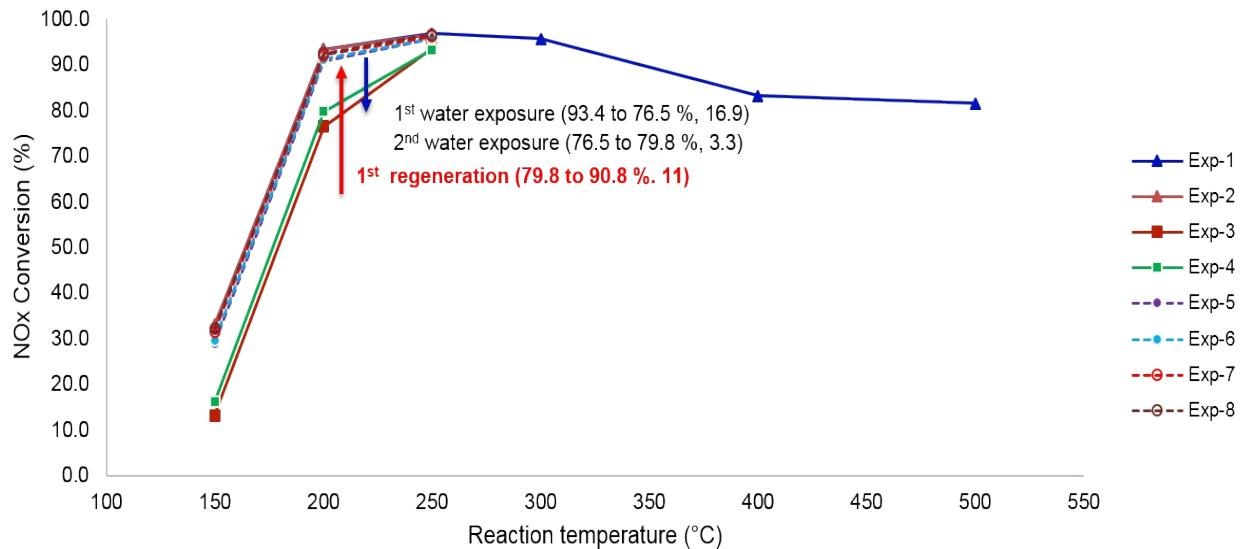
**Figure S2.** NO<sub>x</sub> conversion as a function of temperature on Cu/SAPO-34(TEAOH); reaction conditions: 400 ppm NH<sub>3</sub>, 400 ppm NO, 8% O<sub>2</sub>, 5% H<sub>2</sub>O; GHSV ~24264 h<sup>-1</sup>
