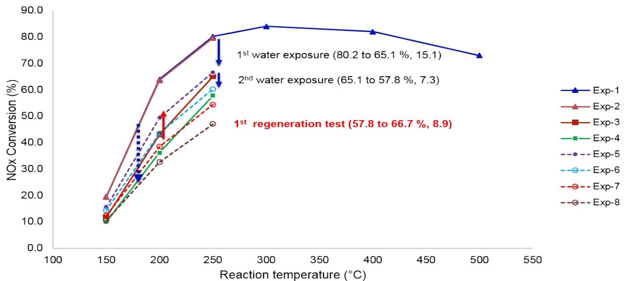
**Figure S3.** NO<sub>x</sub> conversion as a function of temperature on Cu/SAPO-34(ACS); reaction conditions: 400 ppm NH<sub>3</sub>, 400 ppm NO, 8% O<sub>2</sub>, 5% H<sub>2</sub>O; GHSV ~24264 h<sup>-1</sup>
