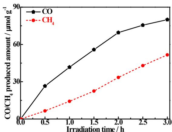
**Fig. S4** Time courses of CO/CH<sub>4</sub> production over 0.25wt% Ru(N'NN')(ONO)-TiO<sub>2</sub> during 3 h full spectrum irradiation of Xe-lamp.
