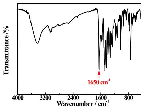
Fig. S1 FTIR spectra of the Ru(II) pincer complex [Ru(N'NN')(ONO)].
