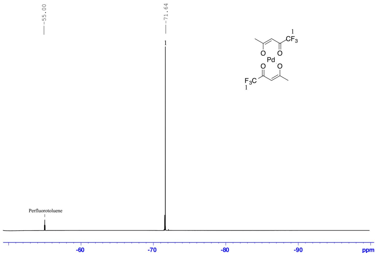
**Figure S10.** <sup>19</sup>F NMR spectrum of Pd(tfpd)<sub>2</sub> in C<sub>6</sub>D<sub>6</sub>.
