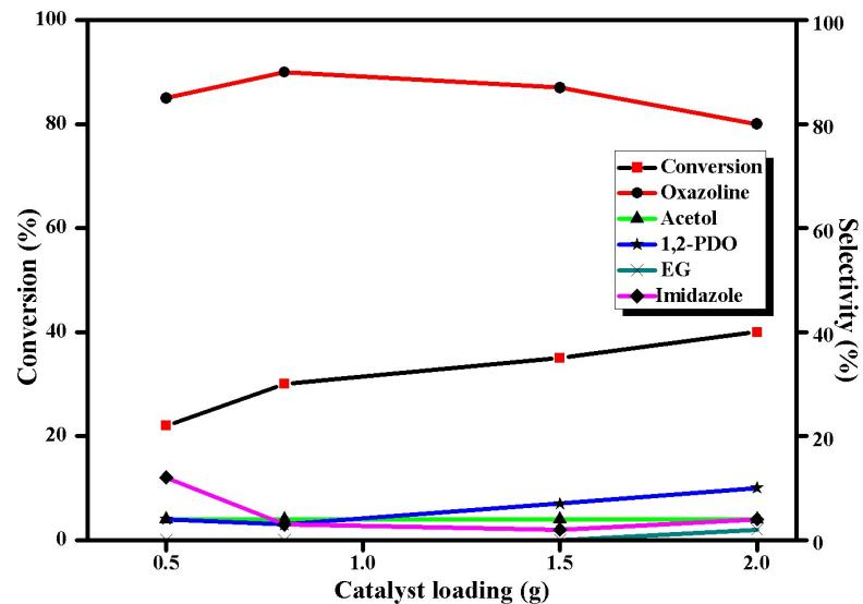
Reaction conditions: 20 wt% glycerol aqueous solution, 220 °C, 15 mL 30% aq. NH<sub>3</sub>, 5 h.
