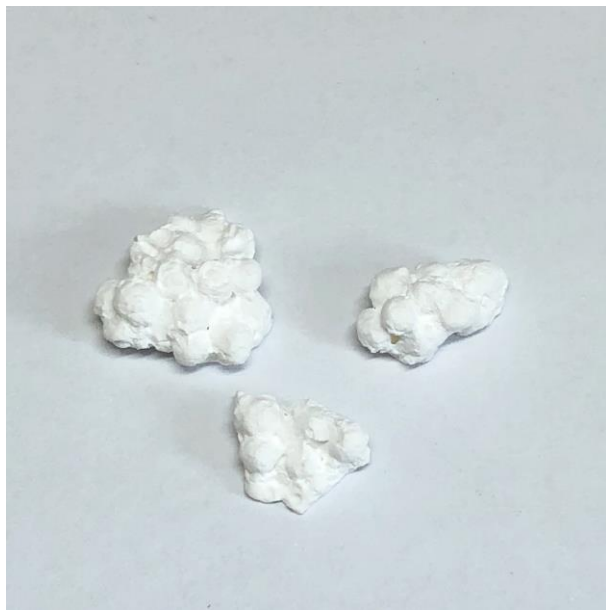
Fig. S1 Photographs of the products synthesized following the procedure of alumina@SAPO-11 without adding CTAB.
