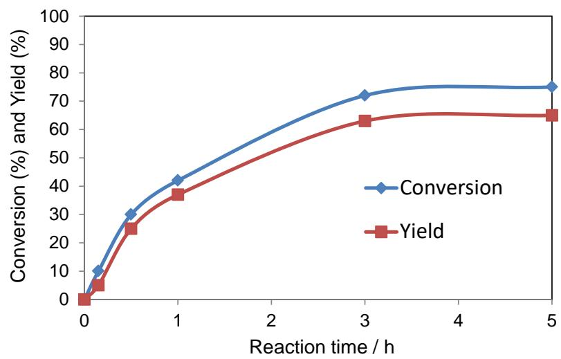
Fig. S1. Time course reaction profile of etherification of **1** and **3** using  $\text{MoO}_3\text{-TiO}_2$  catalyst without calcination (a second cycle).
