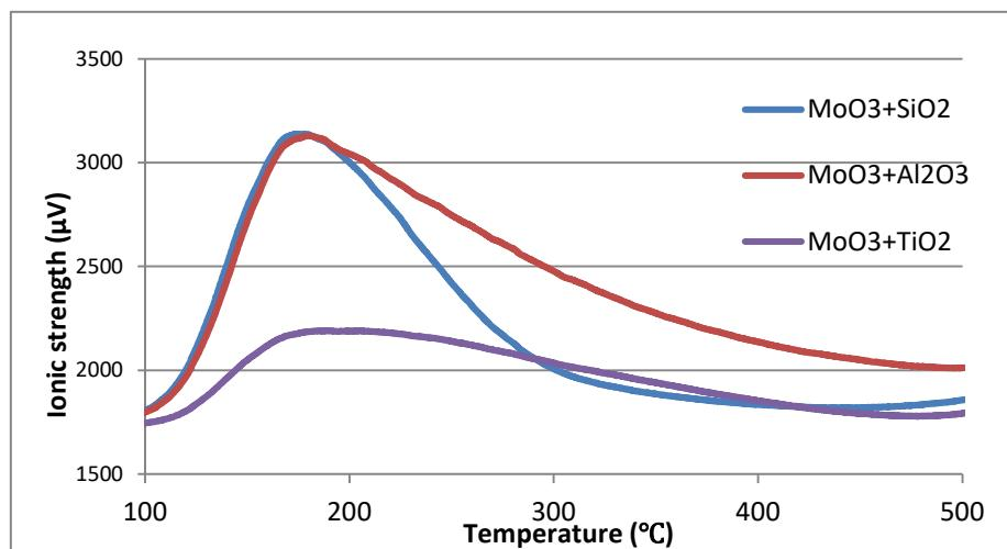
Fig. S2. NH<sub>3</sub>-TPD analyses of MoO<sub>3</sub>-TiO<sub>2</sub>, MoO<sub>3</sub>-SiO<sub>2</sub>, and MoO<sub>3</sub>-Al<sub>2</sub>O<sub>3</sub>.
