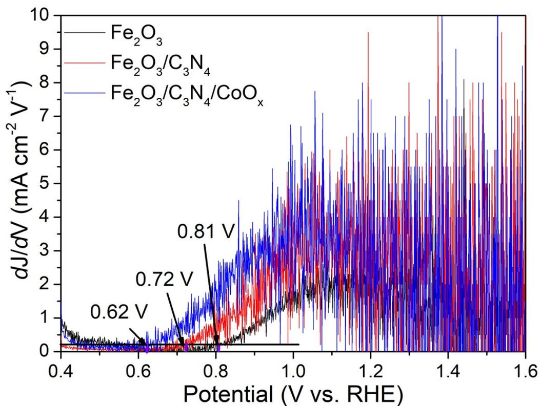
**Fig. S4** First-order derivative curves of the photocurrent densities as a function of the voltage ( $dJ/dV$  curves) for  $\text{Fe}_2\text{O}_3$ ,  $\text{Fe}_2\text{O}_3/\text{C}_3\text{N}_4$ , and  $\text{Fe}_2\text{O}_3/\text{C}_3\text{N}_4/\text{CoO}_x$ .
