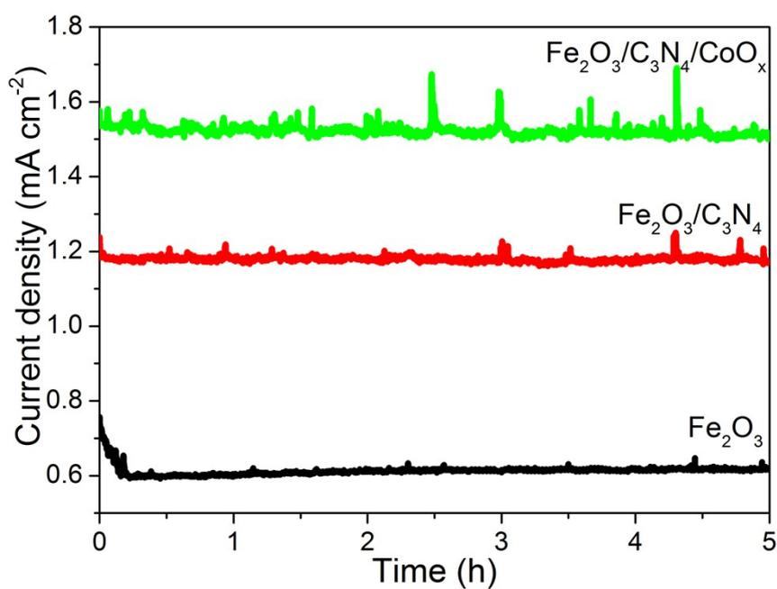
**Fig. S6** Photoelectrochemical stability of Fe<sub>2</sub>O<sub>3</sub>, Fe<sub>2</sub>O<sub>3</sub>/C<sub>3</sub>N<sub>4</sub>, and Fe<sub>2</sub>O<sub>3</sub>/C<sub>3</sub>N<sub>4</sub>/CoO<sub>x</sub> photoanodes at 1.23 V<sub>RHE</sub>. Electrolyte: 1 M of NaOH (pH = 13.6), Light source: AM 1.5 G (100 mW cm<sup>-2</sup>).
