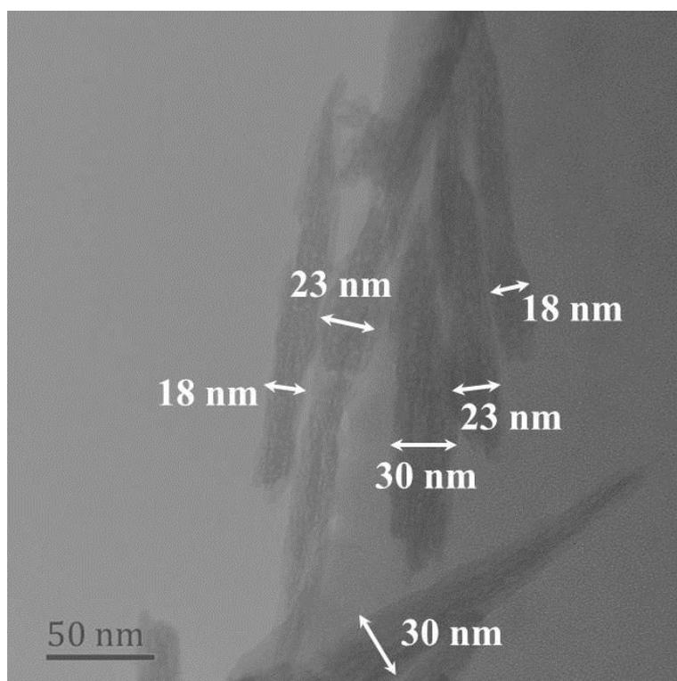
**Fig. S1** Typical TEM image of the as-synthesized FeOOH on a FTO substrate.
