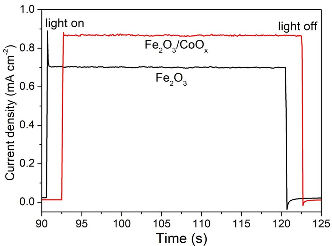
**Fig. S8** Photocurrent density-potential curves as a function of time of Fe<sub>2</sub>O<sub>3</sub> and Fe<sub>2</sub>O<sub>3</sub>/CoO<sub>x</sub> photoanodes at 1.23 V<sub>RHE</sub> under chopped illumination. Electrolyte: 1 M of NaOH (pH = 13.6), Light source: AM 1.5 G (100 mW cm<sup>-2</sup>), Scan rate: 10 mV/s.
