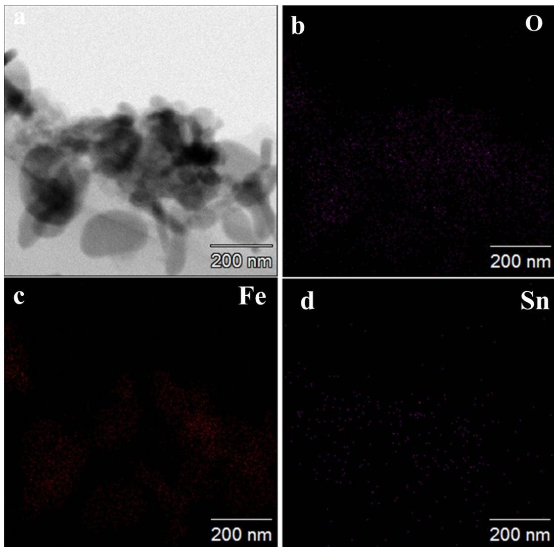
**Fig. S3** a) the scanning transmission electron microscopy (STEM) image, and b) O, c) Fe, and Sn elements mapping.
