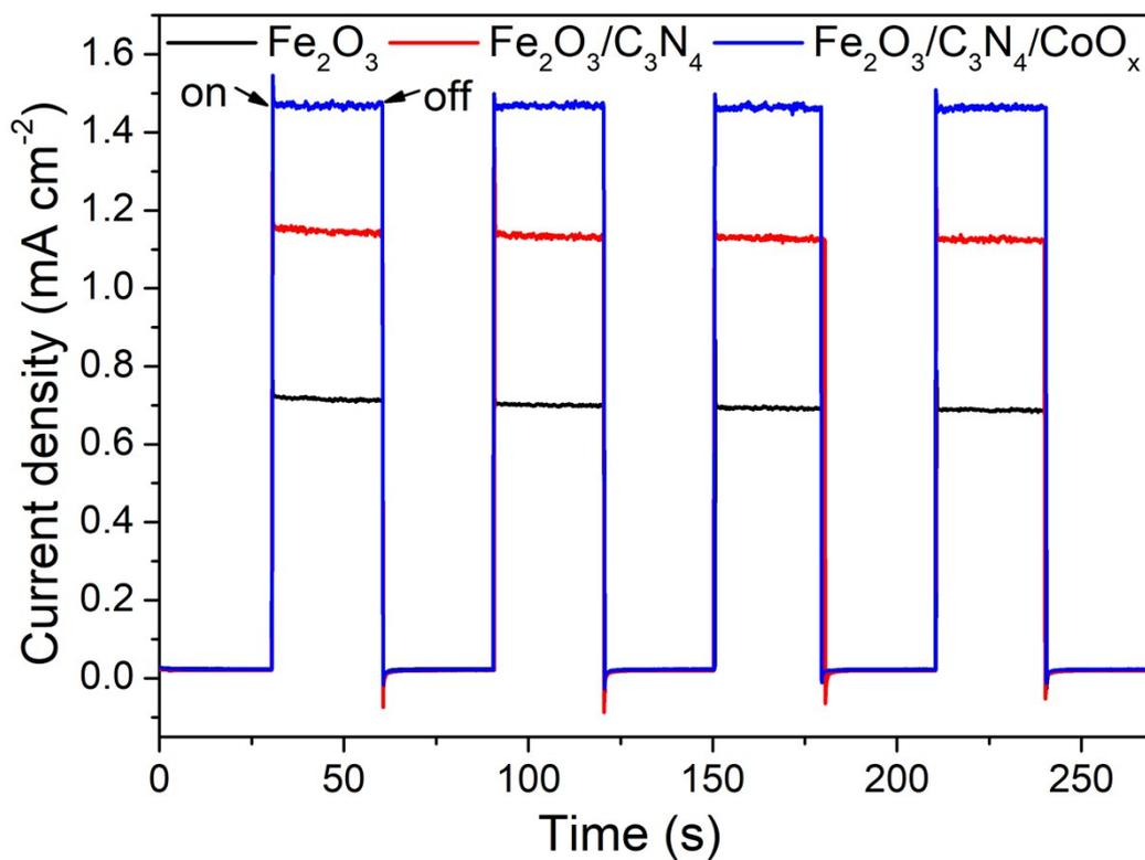
**Fig. S7** Photocurrent density-potential curves as a function of time of Fe<sub>2</sub>O<sub>3</sub>, Fe<sub>2</sub>O<sub>3</sub>/C<sub>3</sub>N<sub>4</sub>, and Fe<sub>2</sub>O<sub>3</sub>/C<sub>3</sub>N<sub>4</sub>/CoO<sub>x</sub> photoanodes at 1.23 V<sub>RHE</sub> under chopped illumination. Electrolyte: 1 M of NaOH (pH = 13.6), Light source: AM 1.5 G (100 mW cm<sup>-2</sup>).
