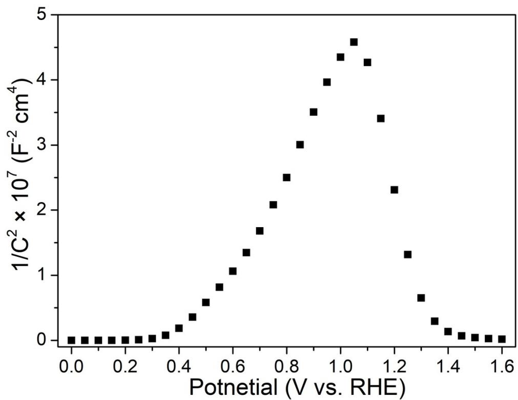
**Fig. S9** Mott-Schottky plots of Fe<sub>2</sub>O<sub>3</sub>/CoO<sub>x</sub> photoanode. Frequency: 1 kHz;
