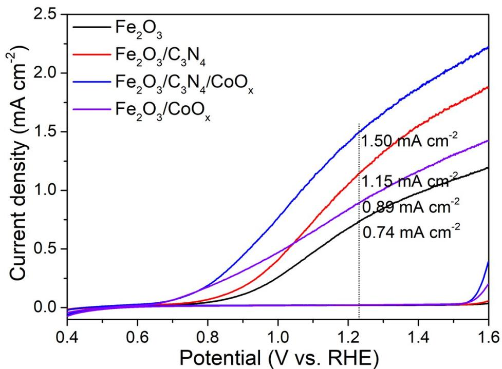
**Fig. S5** Linear sweep voltammograms of Fe<sub>2</sub>O<sub>3</sub>, Fe<sub>2</sub>O<sub>3</sub>/C<sub>3</sub>N<sub>4</sub>, Fe<sub>2</sub>O<sub>3</sub>/C<sub>3</sub>N<sub>4</sub>/CoO<sub>x</sub>, and Fe<sub>2</sub>O<sub>3</sub>/CoO<sub>x</sub>. Electrolyte: 1 M of NaOH (pH = 13.6), Light source: AM 1.5 G (100 mW cm<sup>-2</sup>), Scan rate: 10 mV s<sup>-1</sup>.
