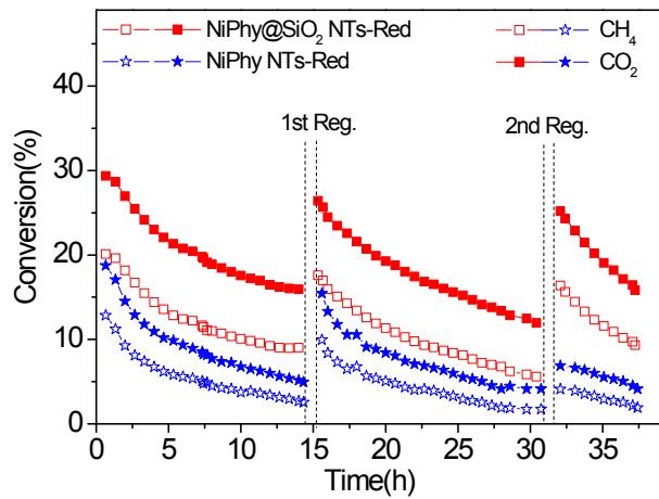
**Fig. S5** Regeneration study of catalysts. Reaction conditions: GHSV of  $1880 \text{ L}\cdot\text{g}^{-1}\text{cat}\cdot\text{h}^{-1}$ ,  $700^\circ\text{C}$ , 1 atm. 1st and 2nd Reg. stands for the first and second times of catalyst regeneration using synthetic air to remove carbon at  $700^\circ\text{C}$ .
