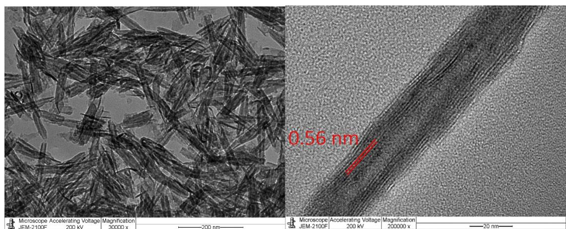
**Fig. S3** TEM images of NiPhy NTs after calcination at 700 °C for 4 h with a ramping rate of 2 °C/min.
