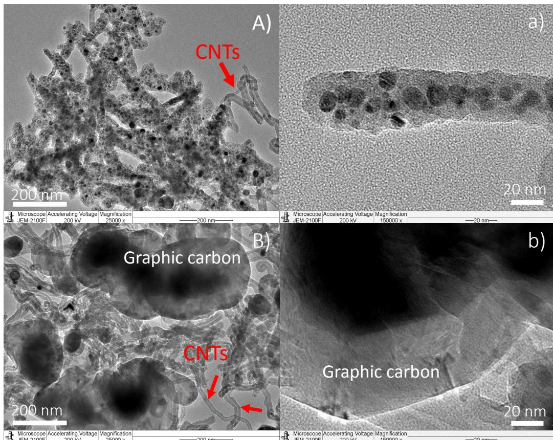
**Fig. S6** TEM images of NiPhy@SiO<sub>2</sub> NTs-Red (A and a) and Ni/SiO<sub>2</sub> catalysts (B and b) after regeneration test.
