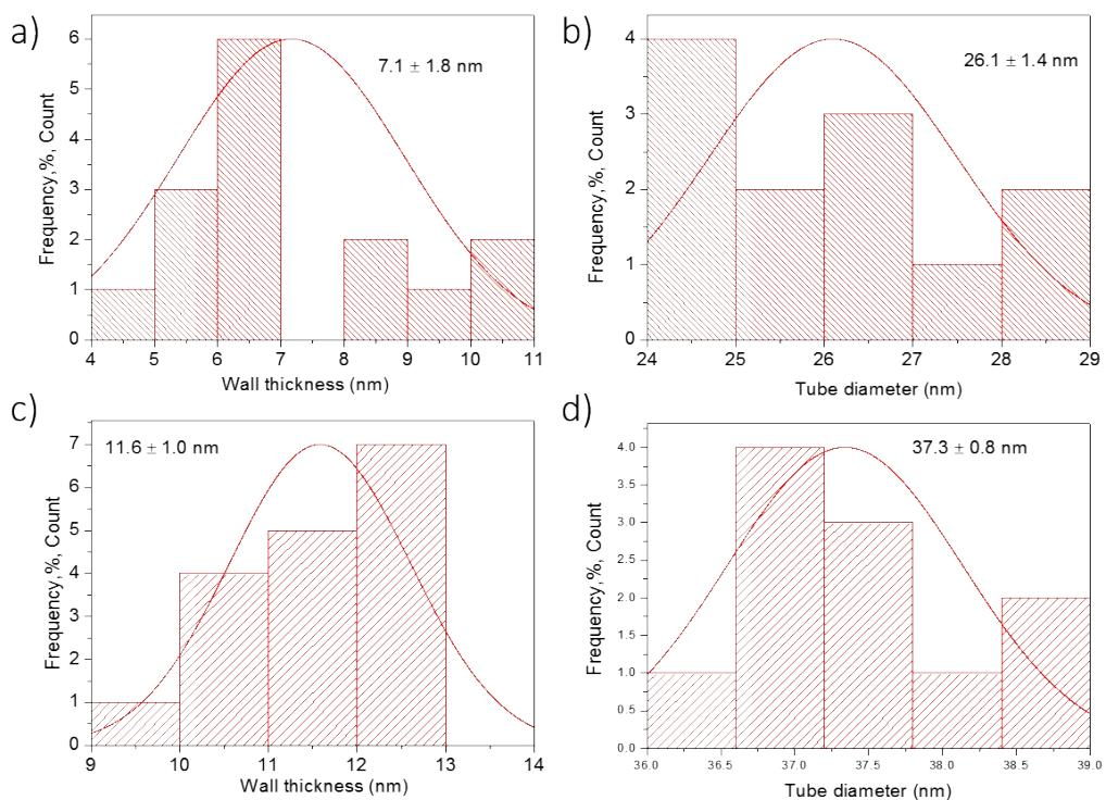
**Fig. S1** Wall thickness and tube diameter for NiPhy NTs (a, b) and SiO<sub>2</sub> NTs (c, d).
