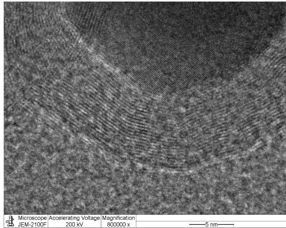
**Fig. S4** HRTEM image of Ni/SiO<sub>2</sub> catalysts after 70 h DRM reaction.
