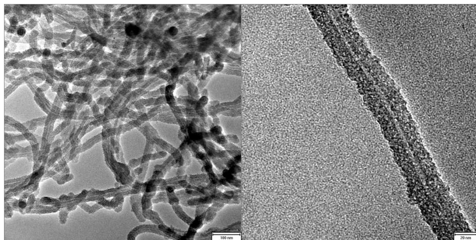
**Fig. S2** TEM images of CNT@SiO<sub>2</sub> nanocomposites
