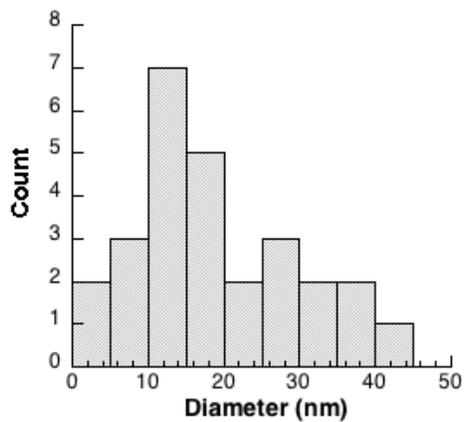
**Figure S3.** Particle distribution of photochemically (I-2959) synthesized AuNP@KNb<sub>3</sub>O<sub>8</sub>. Average diameter: 17.9 ± 10.1 nm.
