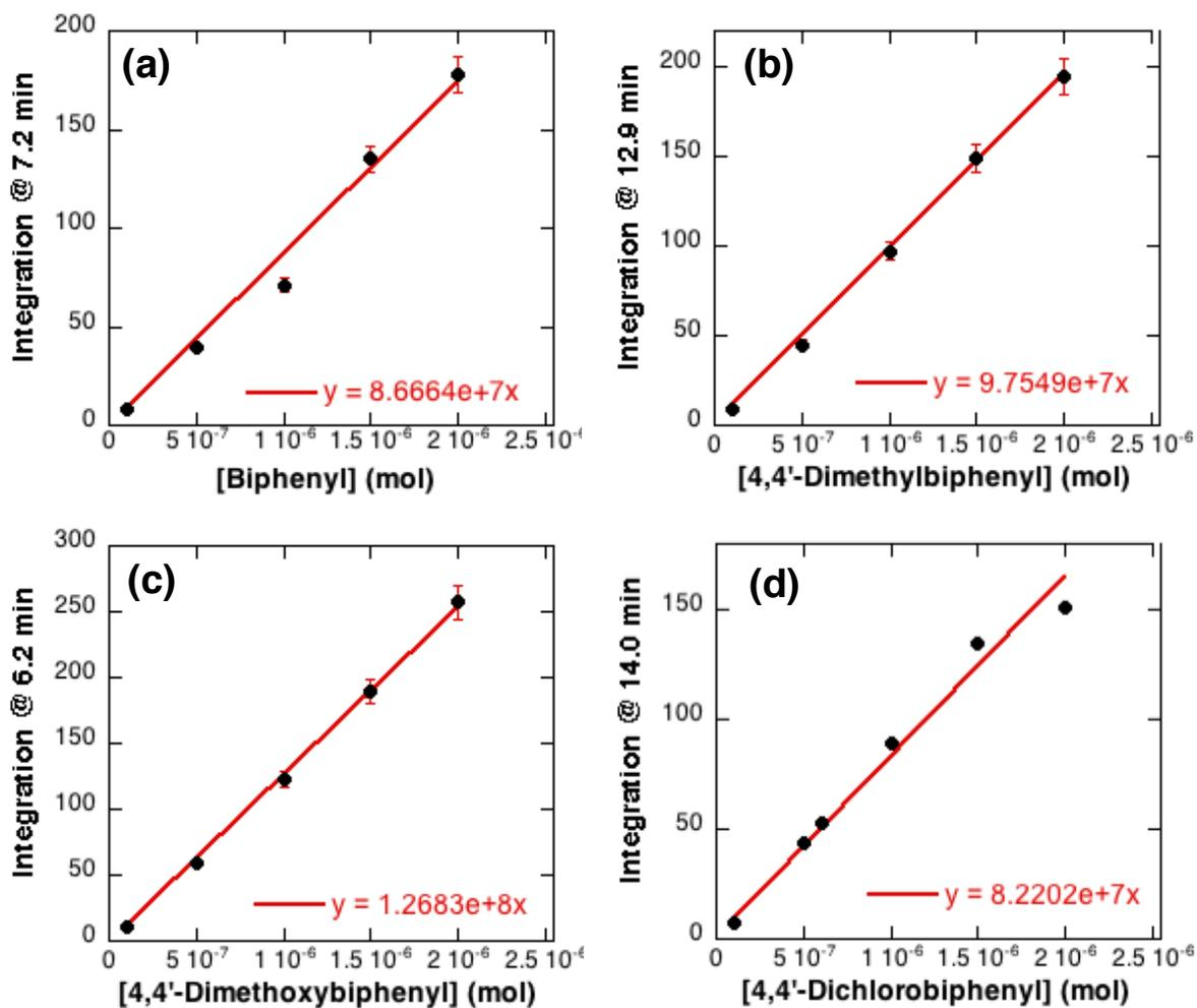
**Figure S2.** Calibration curves for (a) biphenyl, (b) 4,4'-dimethylbiphenyl, (c) 4,4'-dimethoxybiphenyl and (d) 4,4'-dichlorobiphenyl generated using authentic commercial standards and HPLC chromatogram integrations.
