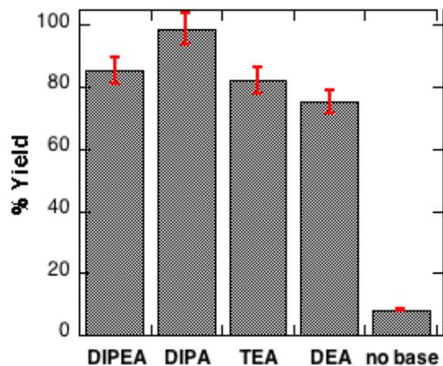
**Figure S4.** Percent biphenyl yield obtained in the presence of various amine sacrificial oxidants. Reaction conditions: 30 mg AuNP/KNb<sub>3</sub>O<sub>8</sub>, 3 μmol iodobenzene, 3 μmol aliphatic amine, 3 mL of CH<sub>3</sub>OH, 2 hours UVA irradiation.
