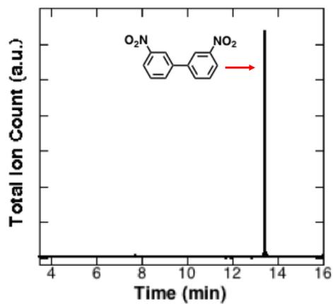
**Figure S6.** Representative GC-MS of AuNP/ $\text{KNb}_3\text{O}_8$ -catalyzed Ullmann homocoupling to form 3,3'-dinitrobiphenyl (Table 2, entry 6). Reaction conditions: aryl halide (3  $\mu\text{mol}$ ), AuNP/ $\text{KNb}_3\text{O}_8$  (30 mg), DIPA (3  $\mu\text{mol}$ ), 3 mL  $\text{CH}_3\text{OH}$ , ambient temperature,  $\text{N}_2$  atmosphere, 1 hr UVA irradiation.
