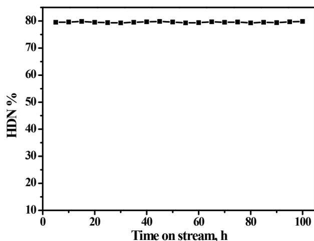
**Figure S8.** Quinoline HDN result with time on stream over NiMo/Zk-3(400 °C, 4.0 MPa, 400 ml/ml and 10 h<sup>-1</sup>)
