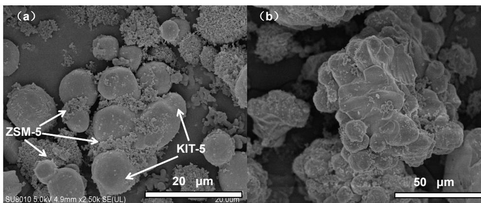
**Figure S3.** SEM images of: (a) PZK, (b) Zk-3.
