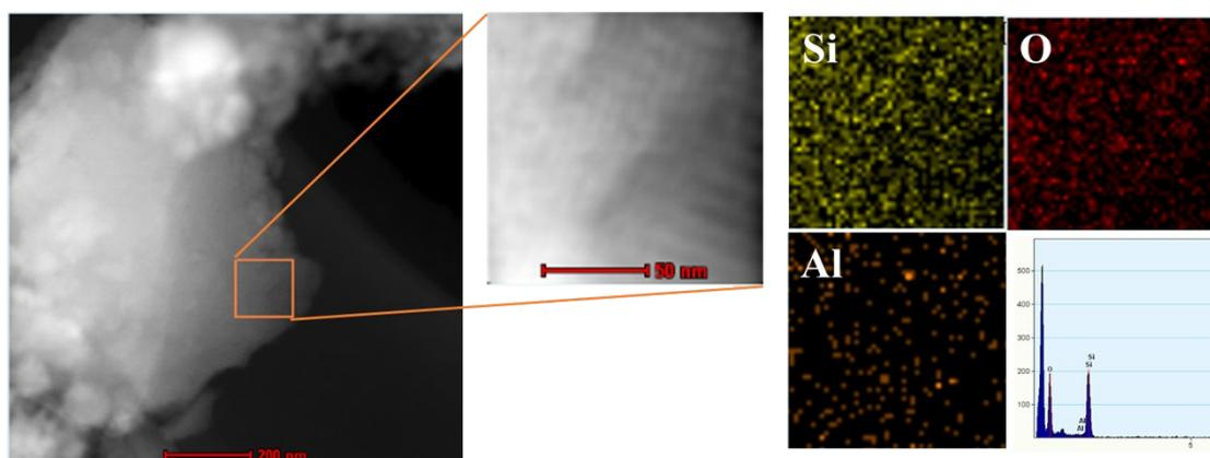
**Figure S2.** HAADF-STEM and EDX elemental mapping images of Zk-3.
