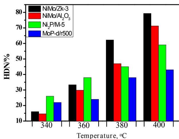
**Figure S9.** Quinoline HDN performance over various catalysts at different temperatures
