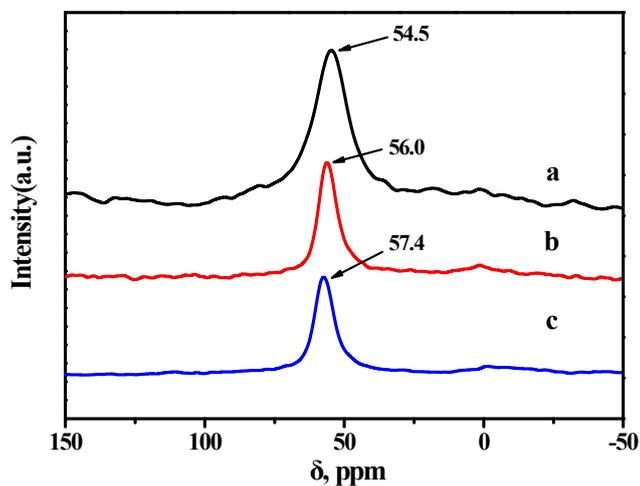
**Figure S4.**  $^{27}\text{Al}$  NMR spectra of the series materials: (a) Al-KIT-5. (b) Zk-3, (c) PZK
