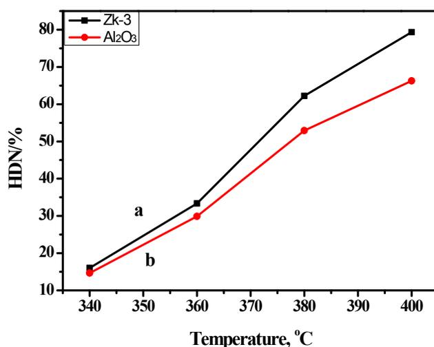
**Figure S7.** Quinoline HDN results at different temperatures (10 h<sup>-1</sup>, 4 MPa, 400 ml/ml).
