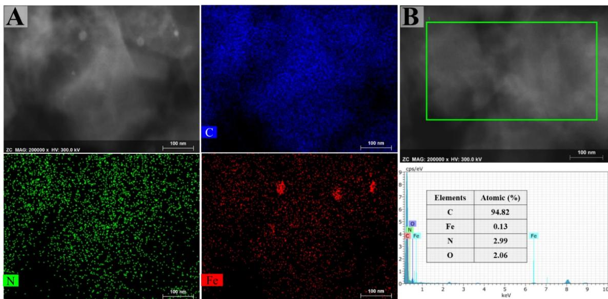
**Fig. S12** A) STEM images with elemental mapping for C, N, and Fe, and B) a selected area EDS spectrum with a table of elemental atomic percentages (inset) of  $\text{Fe}_{0.06}\text{-N/C-900}$  sample after 5000 potential cycles.
