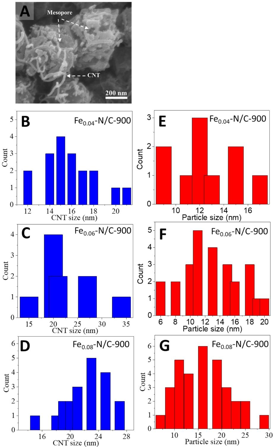
**Fig. S3** A) SEM image of  $\text{Fe}_{0.06}\text{-N/C-900}$  showing the development of pores and N-doped CNTs. B-D) size distribution histograms of CNTs from SEM images in Fig. 3B-D and E-G) particle size distribution from TEM images in Fig. 3F-H for  $\text{Fe}_{0.04}\text{-N/C-900}$ ,  $\text{Fe}_{0.06}\text{-N/C-900}$ , and  $\text{Fe}_{0.08}\text{-N/C-900}$ , respectively.
