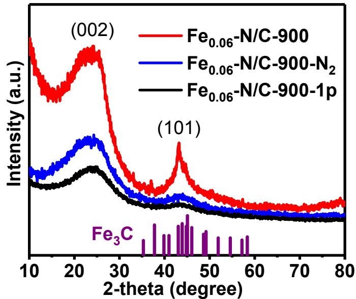
**Fig. S2** XRD spectra of  $\text{Fe}_{0.06}\text{-N/C-900-1p}$ ,  $\text{Fe}_{0.06}\text{-N/C-900-N}_2$ , and  $\text{Fe}_{0.06}\text{-N/C-900}$ .
