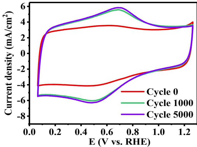
**Fig. S11** Cyclic voltammograms of  $\text{Fe}_{0.06}\text{-N/C-900}$  electrode in  $\text{N}_2$ -saturated 0.1 M  $\text{HClO}_4$  solution at different potential cycles of  $N = 0, 1000, 5000$ .
