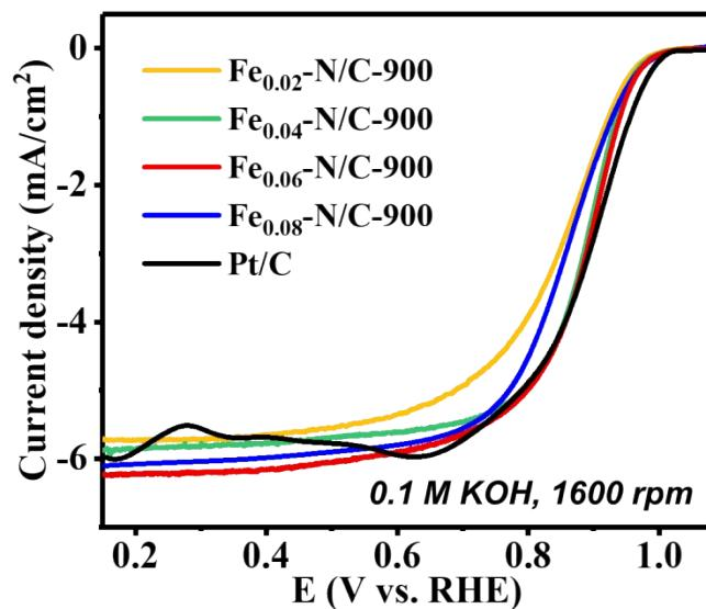
**Fig. S8** LSV curves of as-prepared catalysts  $\text{Fe}_x\text{-N/C-900}$  and Pt/C-TKK in  $\text{O}_2$ -saturated 0.1 M KOH.
