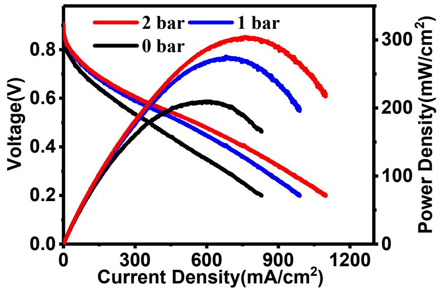
**Fig. S9** H<sub>2</sub>/air fuel cell polarization curves and corresponding power density at 80 °C with various backpressure from 0 to 2 bar (the cathode catalyst loading is 3.5 mg/cm<sup>2</sup>, and membrane of MEA is nafion 212) of Fe<sub>0.06</sub>-N/C-900.
