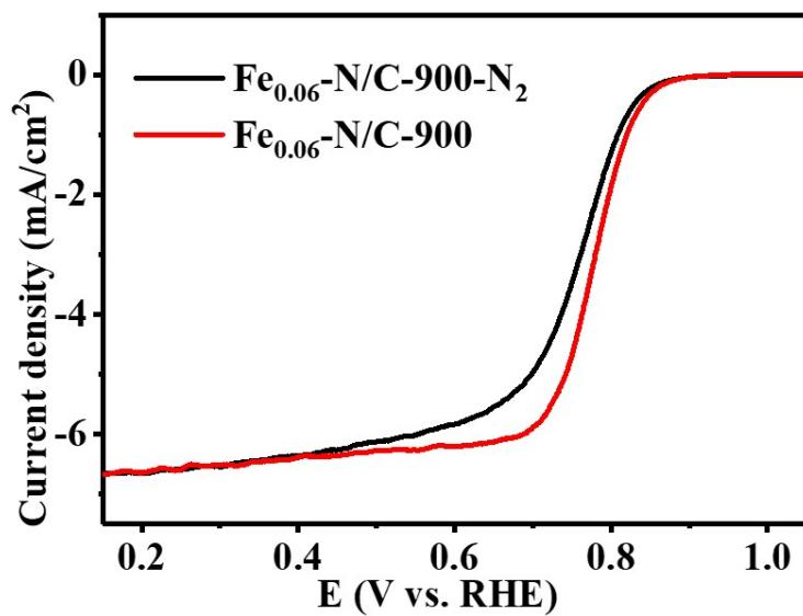
**Fig. S6** LSV curves of  $\text{Fe}_{0.06}\text{-N/C-900}$  and  $\text{Fe}_{0.06}\text{-N/C-900-N}_2$  with rotation speed 1600 rpm at scan rate of 10 mV/s in  $\text{O}_2$ -saturated 0.1 M  $\text{HClO}_4$ .
