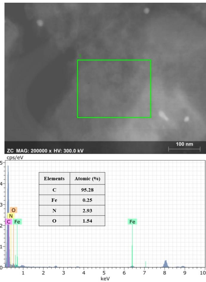
**Fig. S5** STEM image and EDS spectrum of a selected area along with a table of elemental atomic percentage (inset) of  $\text{Fe}_{0.06}\text{-N/C-900}$  catalyst.
