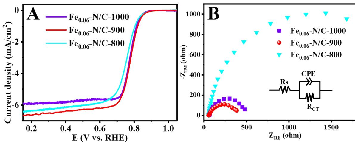
**Fig. S7** A) LSV curves, and B) Nyquist plots (inset: equivalent circuits) of the  $\text{Fe}_{0.06}\text{-N/C-800}$ ,  $\text{Fe}_{0.06}\text{-N/C-900}$ , and  $\text{Fe}_{0.06}\text{-N/C-1000}$  prepared at different pyrolysis temperatures in  $\text{O}_2$ -saturated 0.1 M  $\text{HClO}_4$ .
