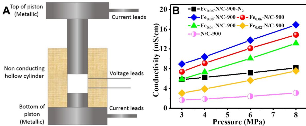
**Fig. S4** A) Electrical conductivity cell with four-probe configuration, and B) electrical conductivity vs pressure profiles of  $\text{Fe}_x\text{-N/C-900}$  and  $\text{Fe}_{0.06}\text{-N/C-900-N}_2$ .
