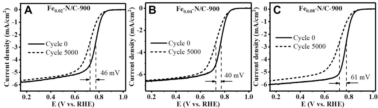
**Fig. S10** LSV curves at before (cycles 0) and after 5000 potential cycles (Cycle 5000) in O<sub>2</sub>-saturated HClO<sub>4</sub> of Fe<sub>0.02</sub>-N/C-900, Fe<sub>0.04</sub>-N/C-900 and Fe<sub>0.08</sub>-N/C-900.
