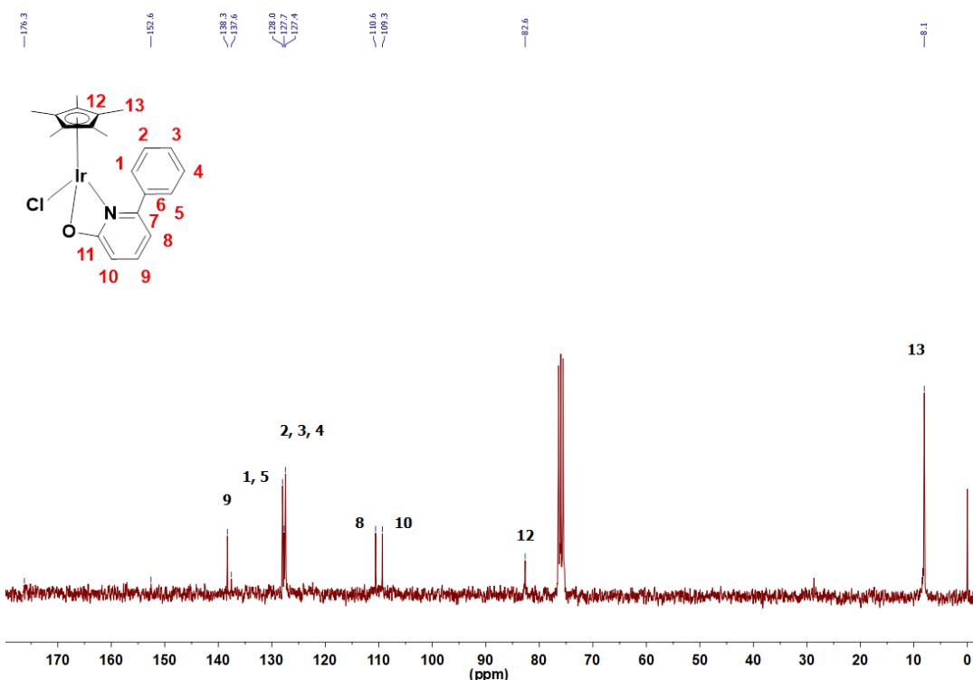
**Fig S59.** <sup>13</sup>C NMR spectra of compound **4** in CDCl<sub>3</sub> (300 MHz).
