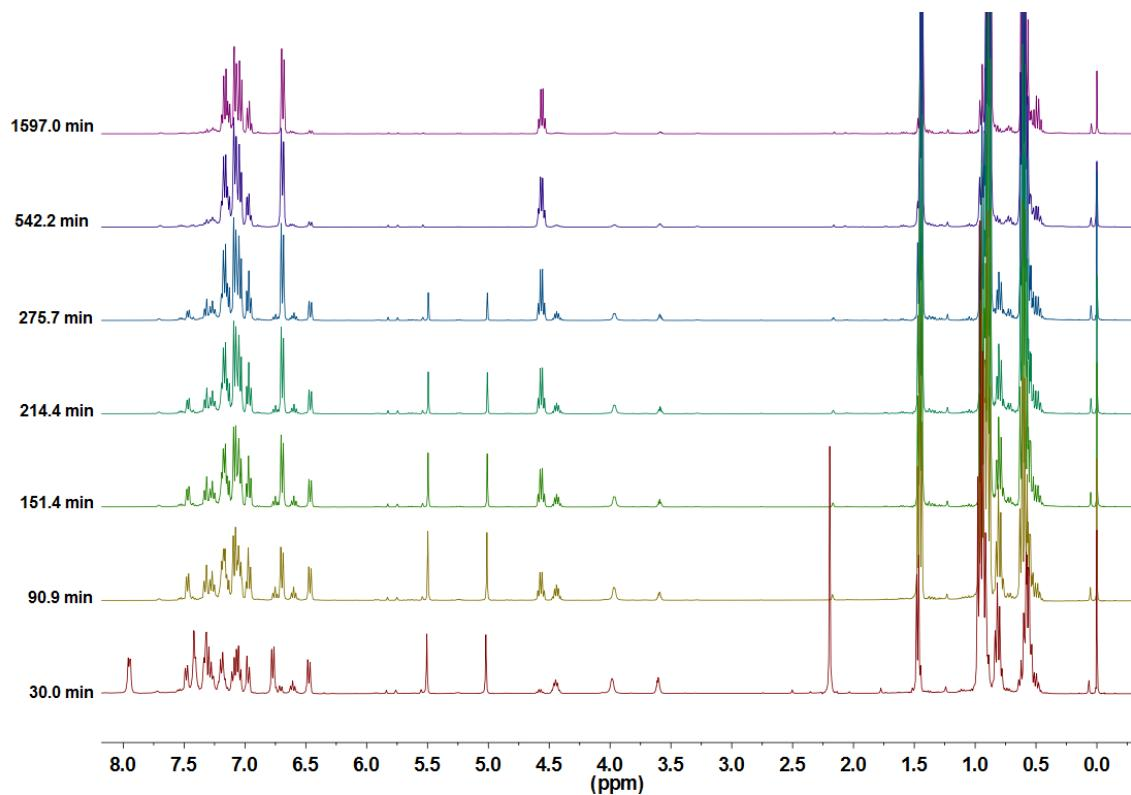
**Fig S47.** Time-resolved  $^1\text{H}$  NMR study of the hydrosilylation of N-(1-phenylethylidene)aniline using precatalyst **5** (300 MHz). Reaction conditions: precatalyst **5** (0.12 mg, 0.0002 mmol), NaBArF<sub>24</sub> (0.34 mg, 0.0004 mmol), N-(1-phenylethylidene)aniline (38.0 mg, 0.1946 mmol), Et<sub>3</sub>SiH (37.3  $\mu\text{L}$ , 0.2335 mmol), 0.5 mL CDCl<sub>3</sub>, internal capillary TMS (10% v/v in CDCl<sub>3</sub>).
