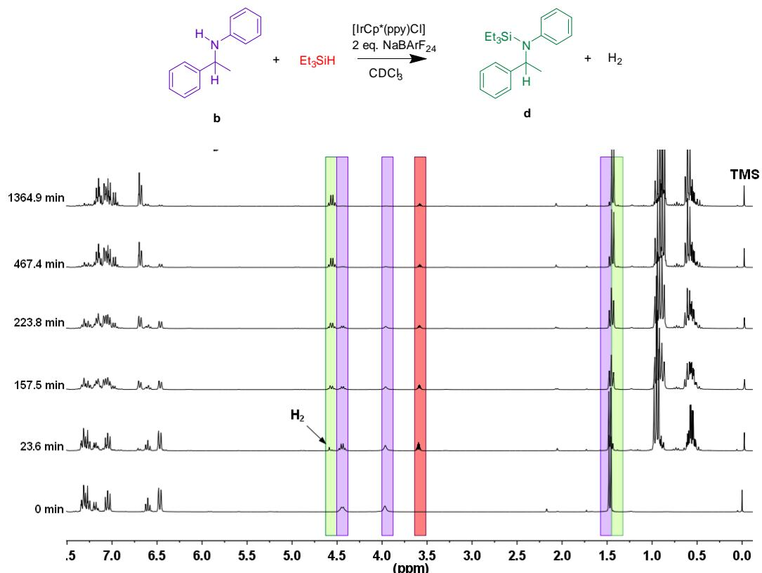
**Fig S20.** Time-resolved <sup>1</sup>H NMR study of the hydrosilylation of N-(1-phenylethyl)aniline (**b**) using precatalyst **1** (CDCl<sub>3</sub>, 300 MHz). Reaction conditions: precatalyst **1** (0.50 mg, 0.0010 mmol), NaBArF<sub>24</sub> (1.70 mg, 0.0019 mmol), N-(1-phenylethyl)aniline (**b**) (38.40 mg, 0.1946 mmol), Et<sub>3</sub>SiH (37.3 µL, 0.2335 mmol), 0.5 mL CDCl<sub>3</sub>, internal capillary TMS (10% v/v in CDCl<sub>3</sub>).
