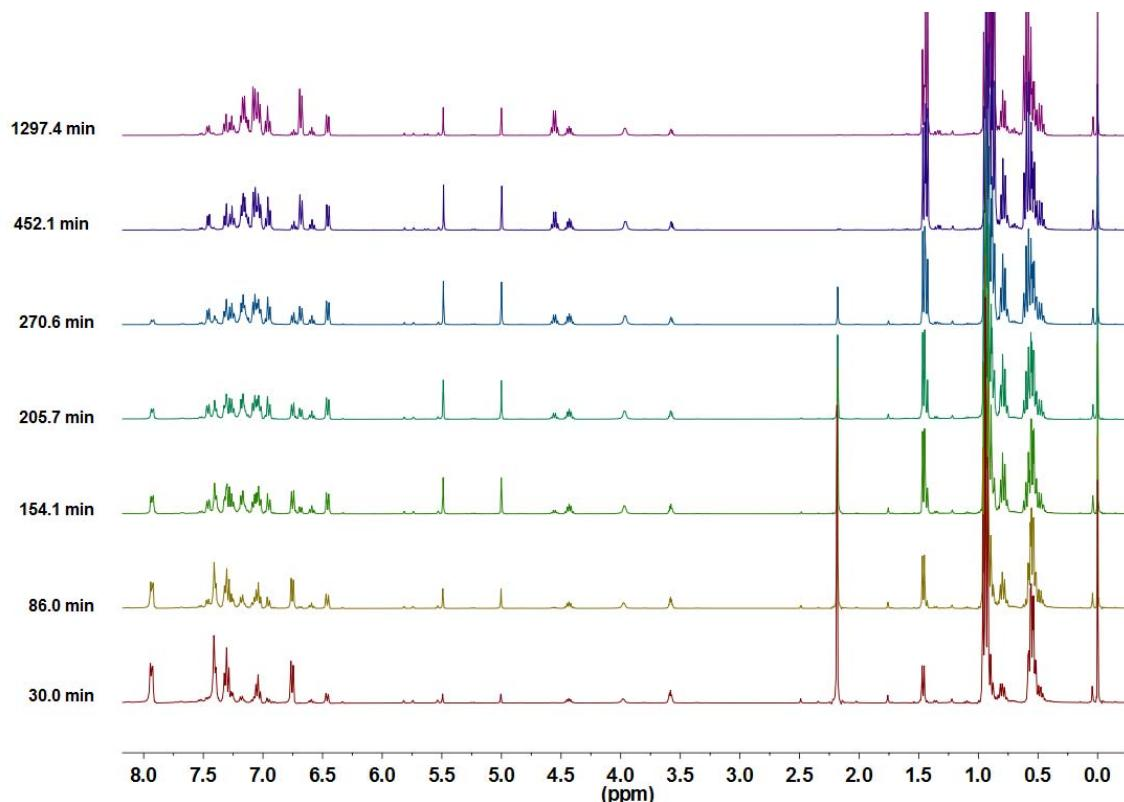
**Fig S49.** Time-resolved  $^1\text{H}$  NMR study of the hydrosilylation of N-(1-phenylethylidene)aniline using precatalyst **6** (300 MHz). Reaction conditions: precatalyst **6** (0.11 mg, 0.0002 mmol), NaBArF<sub>24</sub> (0.34 mg, 0.0004 mmol), N-(1-phenylethylidene)aniline (38.0 mg, 0.1946 mmol), Et<sub>3</sub>SiH (37.3  $\mu\text{L}$ , 0.2335 mmol), 0.5 mL CDCl<sub>3</sub>, internal capillary TMS (10% v/v in CDCl<sub>3</sub>).
