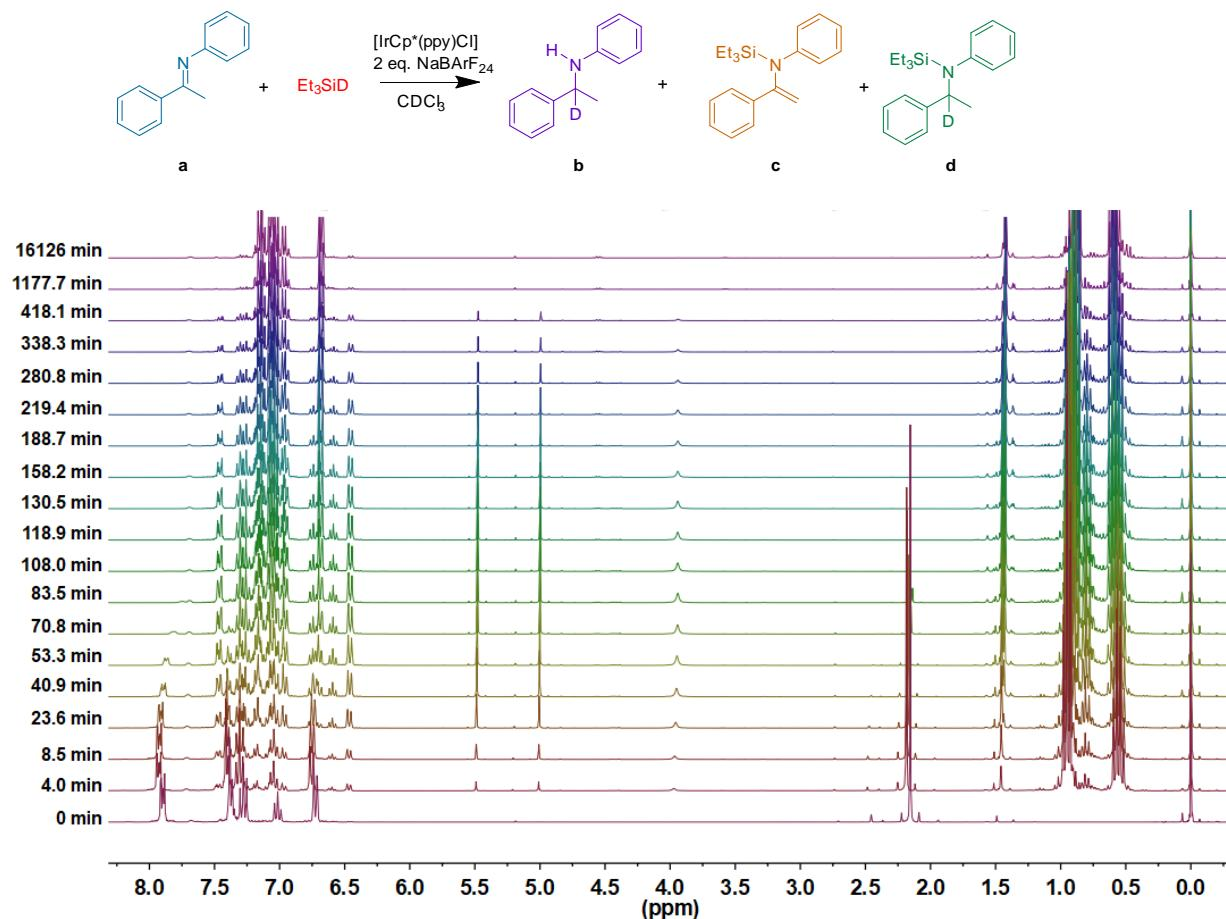
**Fig S22.** Time-resolved <sup>1</sup>H NMR study of the hydrosilylation of N-(1-phenylethylidene)aniline using precatalyst **1** (CDCl<sub>3</sub>, 300 MHz). Reaction conditions: precatalyst **1** (0.50 mg, 0.0010 mmol), NaBARF<sub>24</sub> (1.70 mg, 0.0019 mmol), N-(1-phenylethylidene)aniline (38.00 mg, 0.1946 mmol), Et<sub>3</sub>SiD (37.3 μL, 0.2335 mmol), 0.5 mL CDCl<sub>3</sub>, internal capillary TMS (10% v/v in CDCl<sub>3</sub>).
