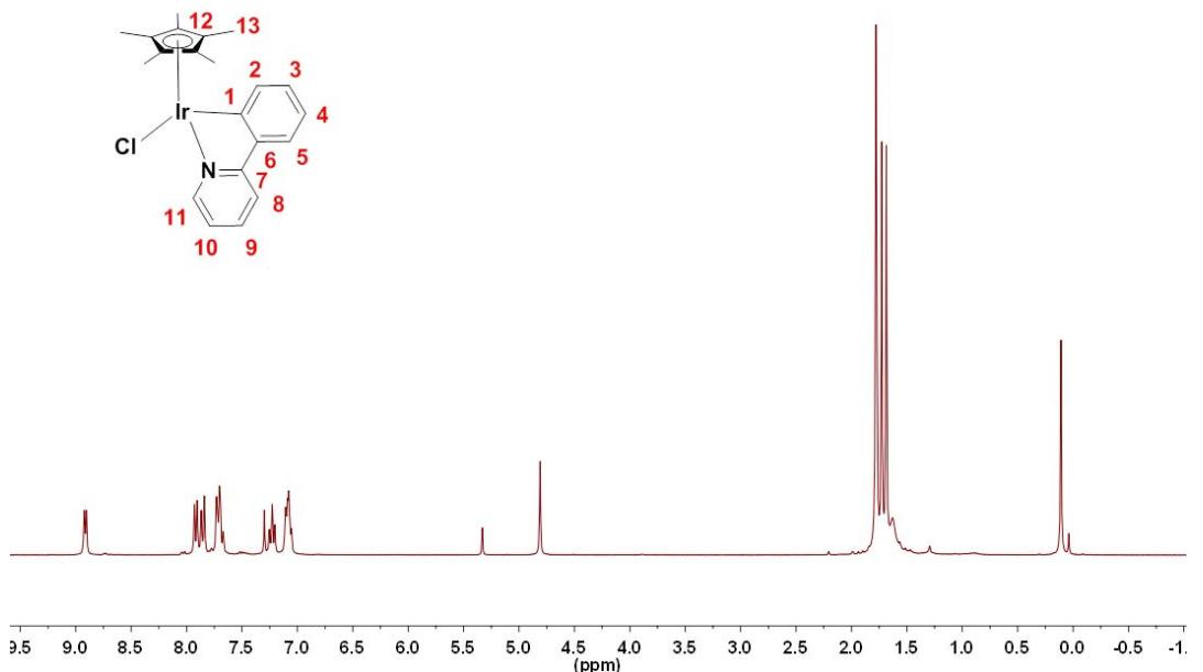
**Fig S51.**  $^1\text{H}$  NMR spectra of compound **1** in  $\text{CDCl}_3$  (300 MHz).
