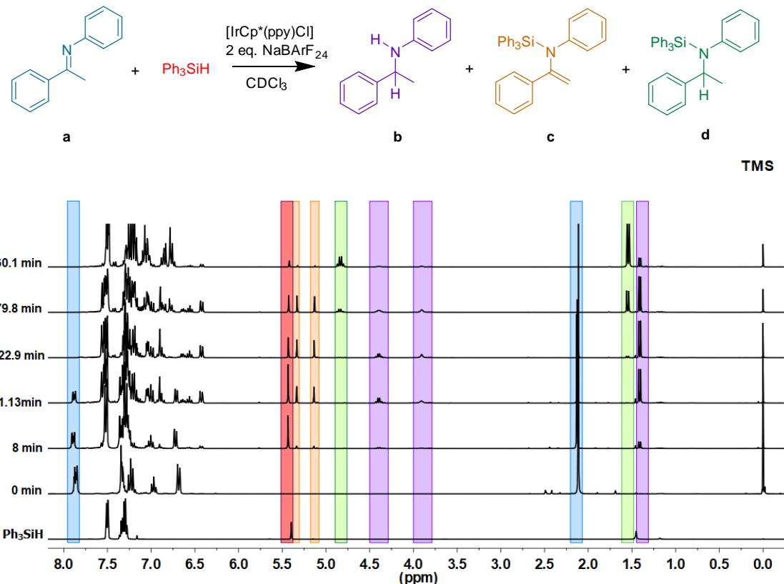
**Fig S26.** Time-resolved <sup>1</sup>H NMR study of the hydrosilylation of N-(1-phenylethylidene)aniline using precatalyst **1** (CDCl<sub>3</sub>, 300 MHz). Reaction conditions: precatalyst **1** (0.5 mg, 0.0010 mmol), NaBArF<sub>24</sub> (1.70 mg, 0.0019 mmol), N-(1-phenylethylidene)aniline (38.00 mg, 0.1946 mmol), Ph<sub>3</sub>SiH (60.93 mg, 0.2335 mmol), 0.5 mL CDCl<sub>3</sub>, internal capillary TMS (10% v/v in CDCl<sub>3</sub>).
