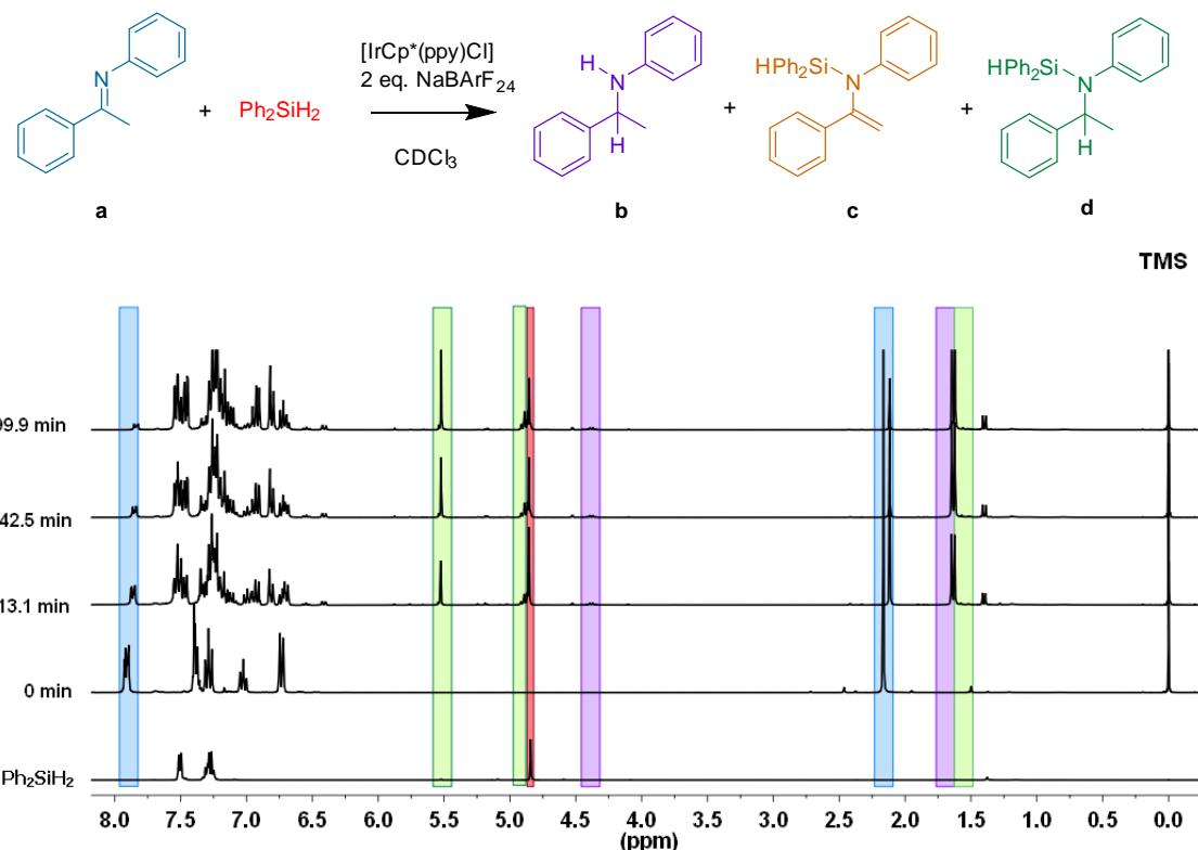
**Fig. S38.** Time-resolved <sup>1</sup>H NMR study of the hydrosilylation of N-(1-phenylethylidene)aniline using precatalyst **1** (CDCl<sub>3</sub>, 300 MHz). Reaction conditions: precatalyst **1** (0.50 mg, 0.0010 mmol), NaBArF<sub>24</sub> (1.70 mg, 0.0019 mmol), N-(1-phenylethylidene)aniline (38.00 mg, 0.1946 mmol), Ph<sub>2</sub>SiH<sub>2</sub> (43.3 μL, 0.2335 mmol), 0.5 mL CDCl<sub>3</sub>, internal capillary TMS (10% v/v in CDCl<sub>3</sub>).
