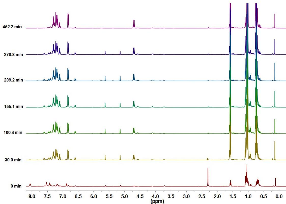
**Fig S43.** Time-resolved  $^1\text{H}$  NMR study of the hydrosilylation of N-(1-phenylethylidene)aniline using precatalyst **3** (300 MHz). Reaction conditions: precatalyst **3** (0.11 mg, 0.0002 mmol), NaBArF<sub>24</sub> (0.34 mg, 0.0004 mmol), N-(1-phenylethylidene)aniline (38.0 mg, 0.1946 mmol), Et<sub>3</sub>SiH (37.3  $\mu\text{L}$ , 0.2335 mmol), 0.5 mL CDCl<sub>3</sub>, internal capillary TMS (10% v/v in CDCl<sub>3</sub>).
