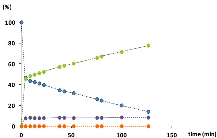
**Fig S39.** Reaction profile of imine-derived products according to *in situ* <sup>1</sup>H NMR spectroscopy. CDCl<sub>3</sub>, 300 MHz. Reaction conditions: precatalyst **1** (0.50 mg, 0.0010 mmol), NaBArF<sub>24</sub> (1.70 mg, 0.0019 mmol), N-(1-phenylethylidene)aniline (38.00 mg, 0.1946 mmol), Ph<sub>2</sub>SiH<sub>2</sub> (43.3 μL, 0.2335 mmol), 0.5 mL CDCl<sub>3</sub>.
