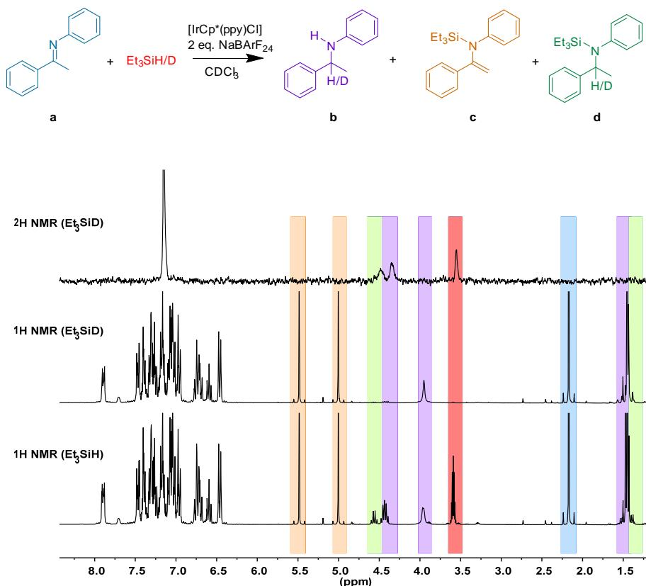
**Fig S23.** <sup>1</sup>H NMR spectra of hydrosilylation reactions at 40 min using Et<sub>3</sub>SiH (bottom) and <sup>1</sup>H and <sup>2</sup>H NMR spectra using Et<sub>3</sub>SiD (top). Reaction conditions: precatalyst **1** (0.50 mg, 0.0010 mmol), NaBArF<sub>24</sub> (1.70 mg, 0.0019 mmol), imine (38.00 mg, 0.1946 mmol), Et<sub>3</sub>SiH or Et<sub>3</sub>SiD (37.3  $\mu$ L, 0.2335 mmol), 0.5 mL CDCl<sub>3</sub> or CHCl<sub>3</sub>, internal capillary TMS (10% v/v in CDCl<sub>3</sub>).
