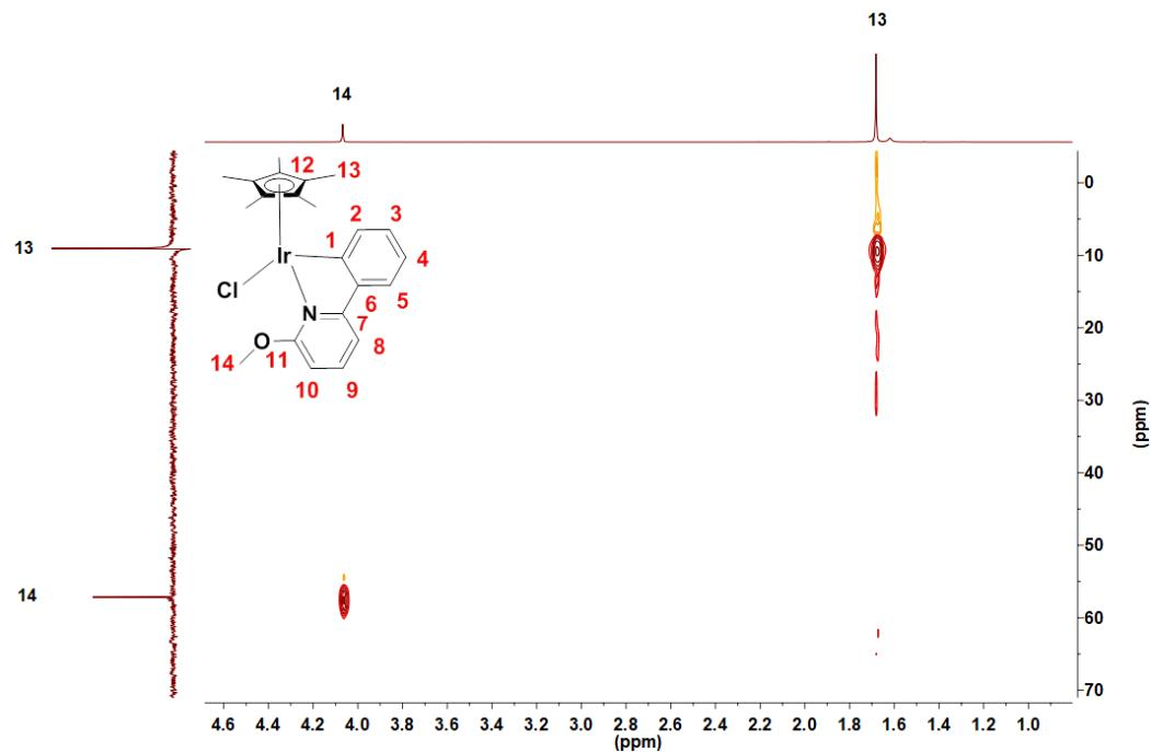
**Fig S57.** Aliphatic region of the HSQC NMR spectra of compound **3** in  $\text{CDCl}_3$ .
