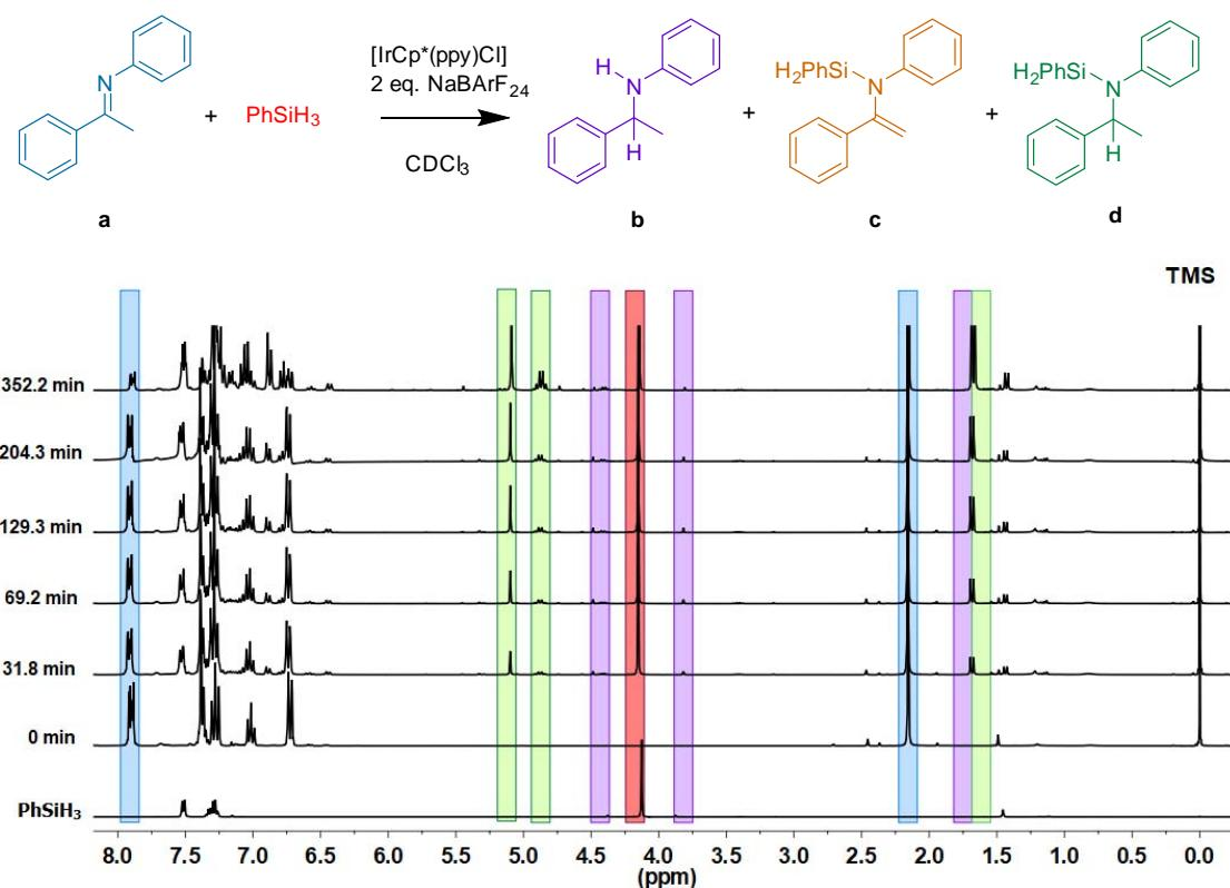
**Fig S36.** Time-resolved  $^1\text{H}$  NMR study of the hydrosilylation of N-(1-phenylethylidene)aniline using precatalyst **1** (CDCl<sub>3</sub>, 300 MHz). Reaction conditions: precatalyst **1** (0.50 mg, 0.0010 mmol), NaBArF<sub>24</sub> (1.70 mg, 0.0019 mmol), N-(1-phenylethylidene)aniline (38.00 mg, 0.1946 mmol), PhSiH<sub>3</sub> (28.8  $\mu\text{L}$ , 0.2335 mmol), 0.5 mL CDCl<sub>3</sub>, internal capillary TMS (10% v/v in CDCl<sub>3</sub>).
