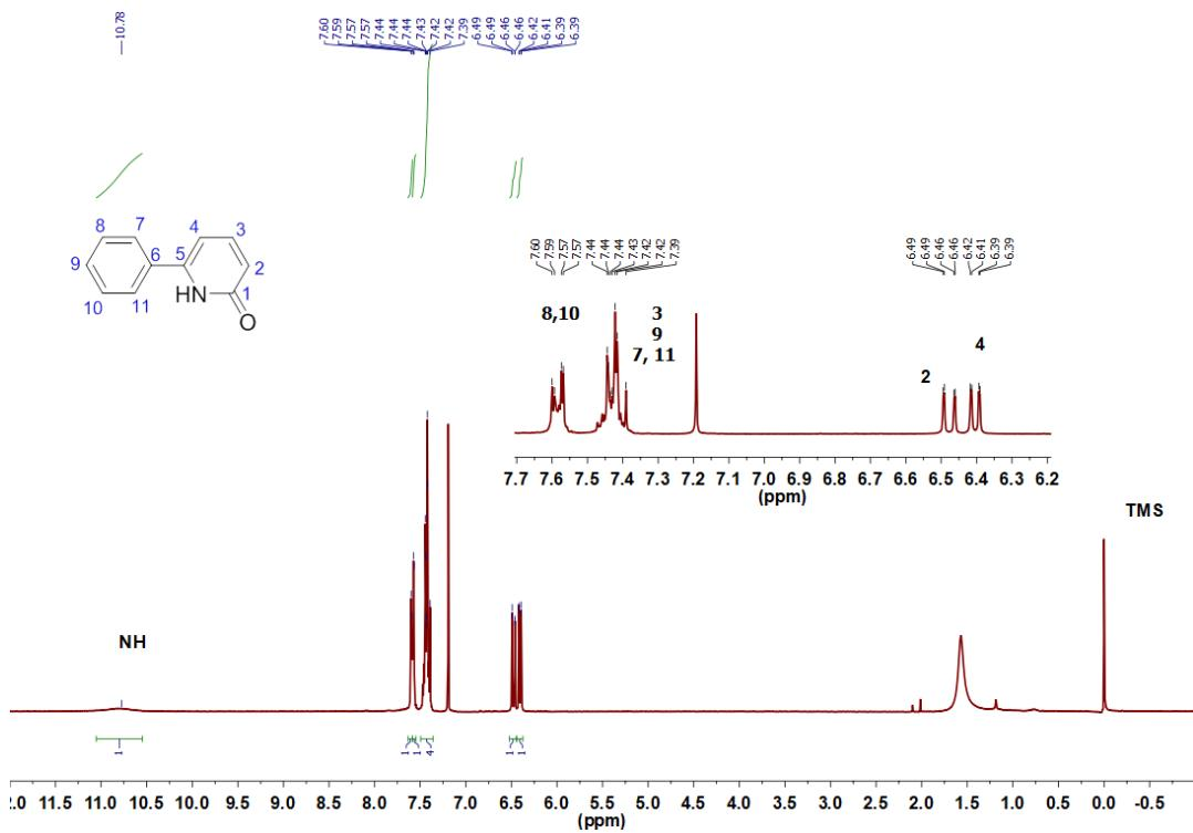
**Fig S68.**  $^1\text{H}$  NMR spectra of 6-phenyl-2-pyridone in  $\text{CDCl}_3$  (300 MHz).
