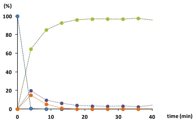
**Fig S29.** Reaction profile of imine-derived products according to *in situ* <sup>1</sup>H NMR spectroscopy.  $\text{CDCl}_3$ , 300 MHz. Reaction conditions: precatalyst **1** (0.50 mg, 0.0010 mmol),  $\text{NaBArF}_{24}$  (1.70 mg, 0.0019 mmol), N-(1-phenylethylidene)aniline (38.00 mg, 0.1946 mmol),  $\text{MePh}_2\text{SiH}$  (46.3  $\mu\text{L}$ , 0.2335 mmol), 0.5 mL  $\text{CDCl}_3$ .
