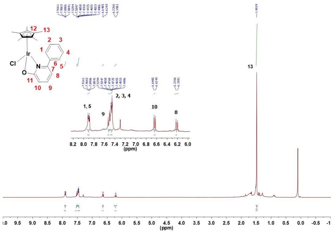
**Fig S58.**  $^1\text{H}$  NMR spectra of compound **4** in  $\text{CDCl}_3$  (300 MHz).
