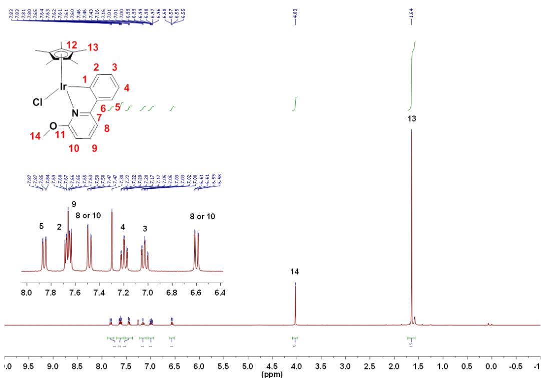
**Fig S53.**  $^1\text{H}$  NMR spectra of compound 3 in  $\text{CDCl}_3$  (300 MHz).
