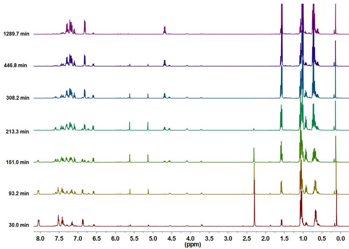
**Fig S41.** Time-resolved  $^1\text{H}$  NMR study of the hydrosilylation of N-(1-phenylethylidene)aniline using precatalyst **2** (300 MHz). Reaction conditions: precatalyst **2** (0.11 mg, 0.0002 mmol), NaBArF<sub>24</sub> (0.34 mg, 0.0004 mmol), N-(1-phenylethylidene)aniline (38.0 mg, 0.1946 mmol), Et<sub>3</sub>SiH (37.3  $\mu\text{L}$ , 0.2335 mmol), 0.5 mL CDCl<sub>3</sub>, internal capillary TMS (10% v/v in CDCl<sub>3</sub>).
