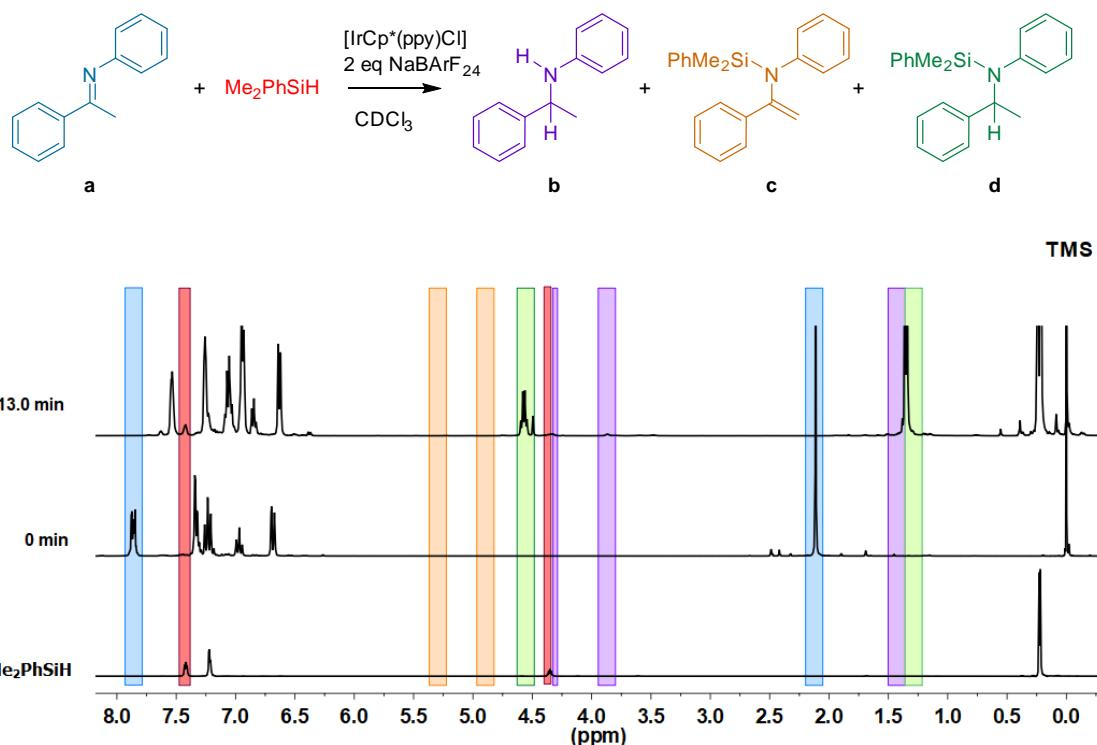
**Fig S30.** Time-resolved <sup>1</sup>H NMR study of the hydrosilylation of N-(1-phenylethylidene)aniline using precatalyst **1** ( $\text{CDCl}_3$ , 300 MHz). Reaction conditions: precatalyst **1** (0.50 mg, 0.0010 mmol),  $\text{NaBArF}_{24}$  (1.70 mg, 0.0019 mmol), N-(1-phenylethylidene)aniline (38.00 mg, 0.1946 mmol),  $\text{Me}_2\text{PhSiH}$  (36.2  $\mu\text{L}$ , 0.2335 mmol), 0.5 mL  $\text{CDCl}_3$ , internal capillary TMS (10% v/v in  $\text{CDCl}_3$ ).
