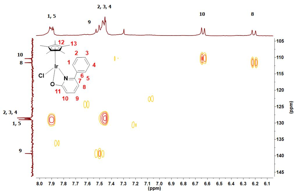
**Fig S61.** Aliphatic region of the HSQC NMR spectra of compound **4** in CDCl<sub>3</sub>.
