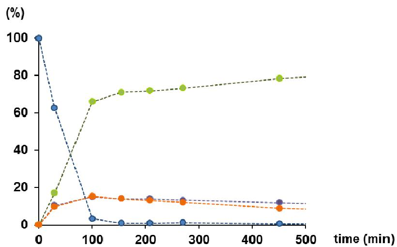
**Fig S44.** Reaction profile of A) imine-derived and B) silane-containing products, according to *in situ*  $^1\text{H}$  NMR spectroscopy. Reaction conditions: precatalyst **3** (0.11 mg, 0.0002 mmol), NaBArF<sub>24</sub> (0.34 mg, 0.0004 mmol), N-(1-phenylethylidene)aniline (38.0 mg, 0.1946 mmol), Et<sub>3</sub>SiH (37.3  $\mu\text{L}$ , 0.2335 mmol), 0.5 mL CDCl<sub>3</sub>, internal capillary TMS (10% v/v in CDCl<sub>3</sub>).
