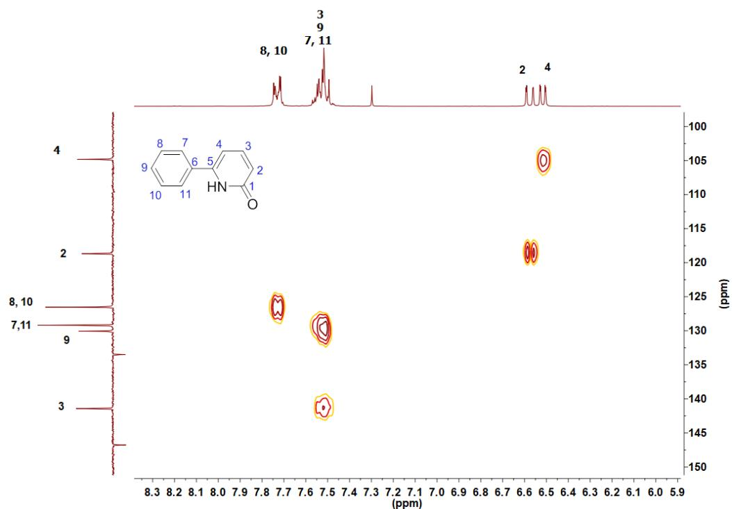
**Fig S71.** Aromatic region of the HSQC NMR spectra of 6-phenyl-2-pyridone in  $\text{CDCl}_3$ .
