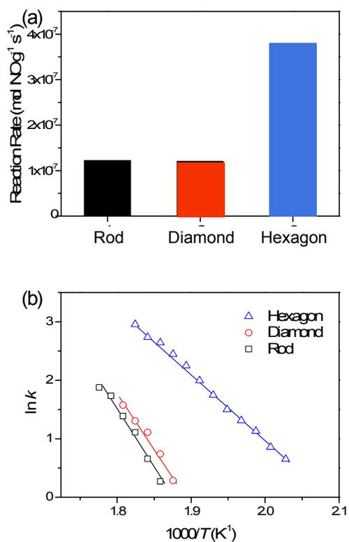
Figure S1. (a) Catalytic activities (at 300 °C) and (b) Arrhenius-type plots for selective catalytic reduction of NO<sub>x</sub> over Fe<sub>2</sub>O<sub>3</sub>-hexagon, Fe<sub>2</sub>O<sub>3</sub>-diamond, and Fe<sub>2</sub>O<sub>3</sub>-rods.
