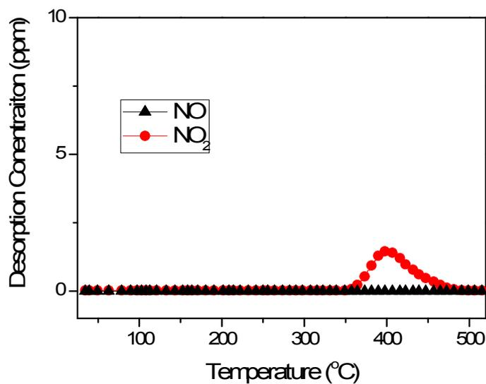
Figure S3. TPD spectra of  $NO$  and  $NO_2$  taken after exposing the  $Fe_2O_3$ -hexagon sample to a saturation dose of  $NO/3\%O_2/N_2$ .
