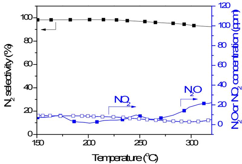
Figure S2.  $N_2$  selectivity, outlet  $N_2O$ , and  $N_2O$  concentration as a function of temperature over  $Fe_2O_3$ -hexagon. Reactant feed contains 600 ppm of  $NO$ , 600 ppm of  $NH_3$ , 3 vol%  $O_2$ , balanced with  $N_2$ .
