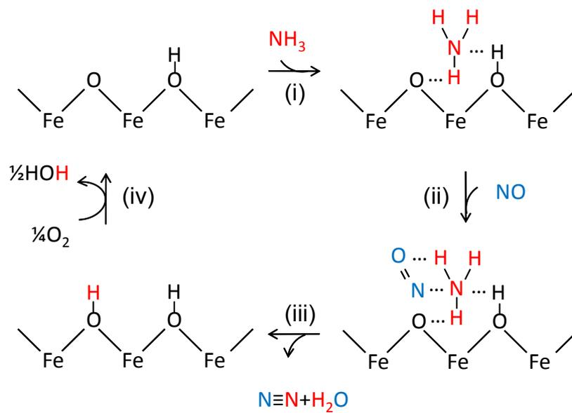
Figure S4. A plausible reaction mechanism of  $\text{NH}_3$ -SCR on  $\text{Fe}_2\text{O}_3$ -hexagon.
