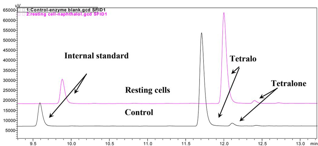
Fig. S7 *E. coli* cells containing empty plasmids to perform the catalytic reaction for tetralol. The resting cells of containing empty plasmids (red line) and control without enzyme (black line) were used to perform the oxidation reaction. The control was set as the substrate without any protein.
