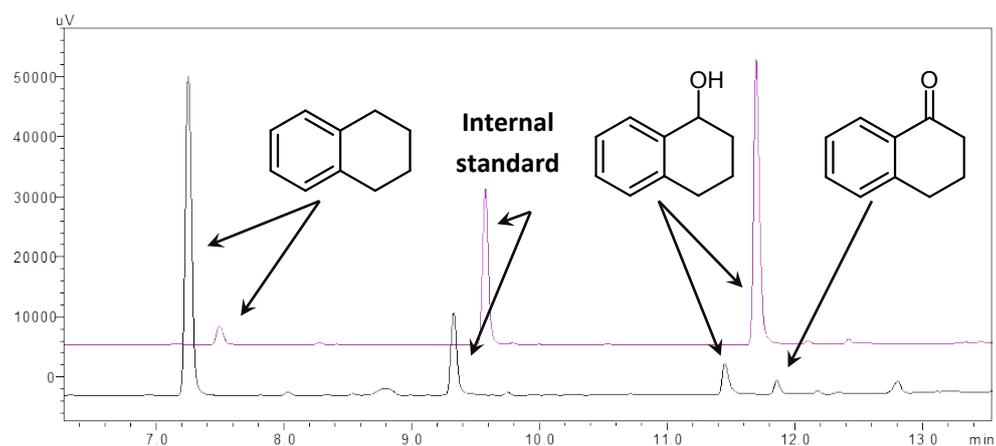
Fig. S3 Product selectivity analyzed by GC, Rsi-MS column. The black line represents wild type (WT) for the biotransformation of tetralin. The red line was RJ3 for the transformation.
