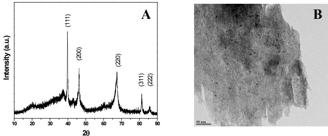
**Fig. S4** PXRD pattern (A) and TEM (B) image of 3.5 wt% Pt loaded  $\text{Al}_2\text{O}_3$  catalyst
