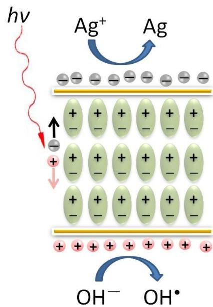
**Figure S11.** A schematic illustrating the photoinduced Ag deposition on the surface of ferroelectric materials.
