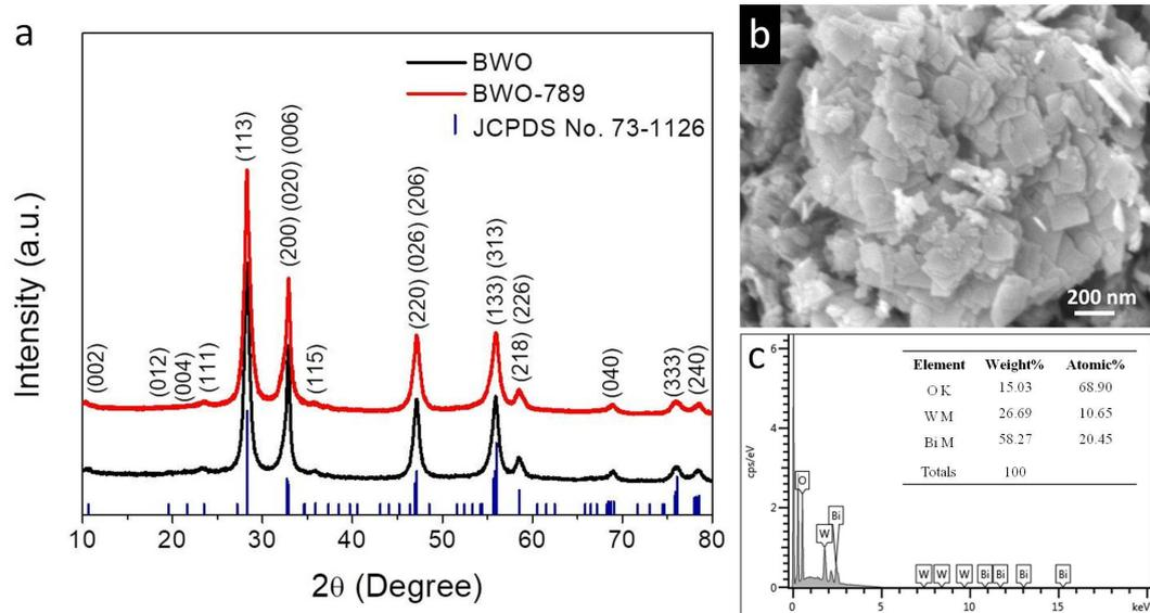
**Figure S9.** XRD (a), SEM (b) and EDS (c) results of poled BWO-789 after the cycling experiment.
