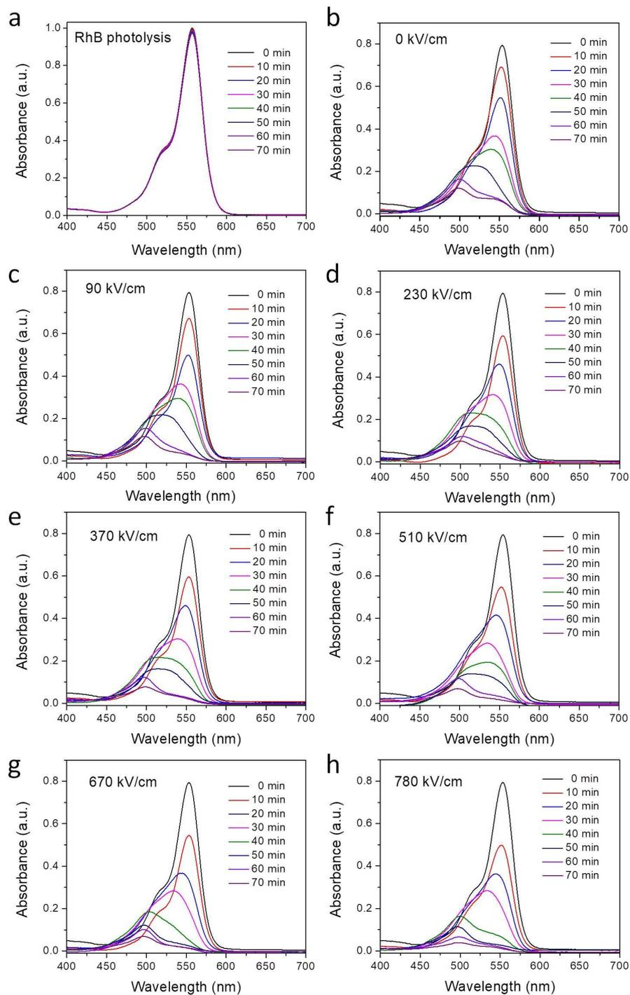
**Figure S5.** The temporal evolutions of all the absorption spectra of the RhB solution ( $10^{-5}$  mol/L) degraded by unpoled and poled  $\text{Bi}_2\text{WO}_6$  under Xe lamp light irradiation.
