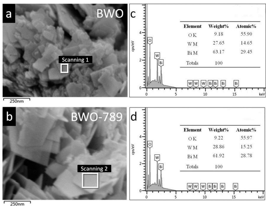
**Figure S2.** SEM and EDS results of pristine  $\text{Bi}_2\text{WO}_6$  (a, c) and poled BWO-789 (b, d).
