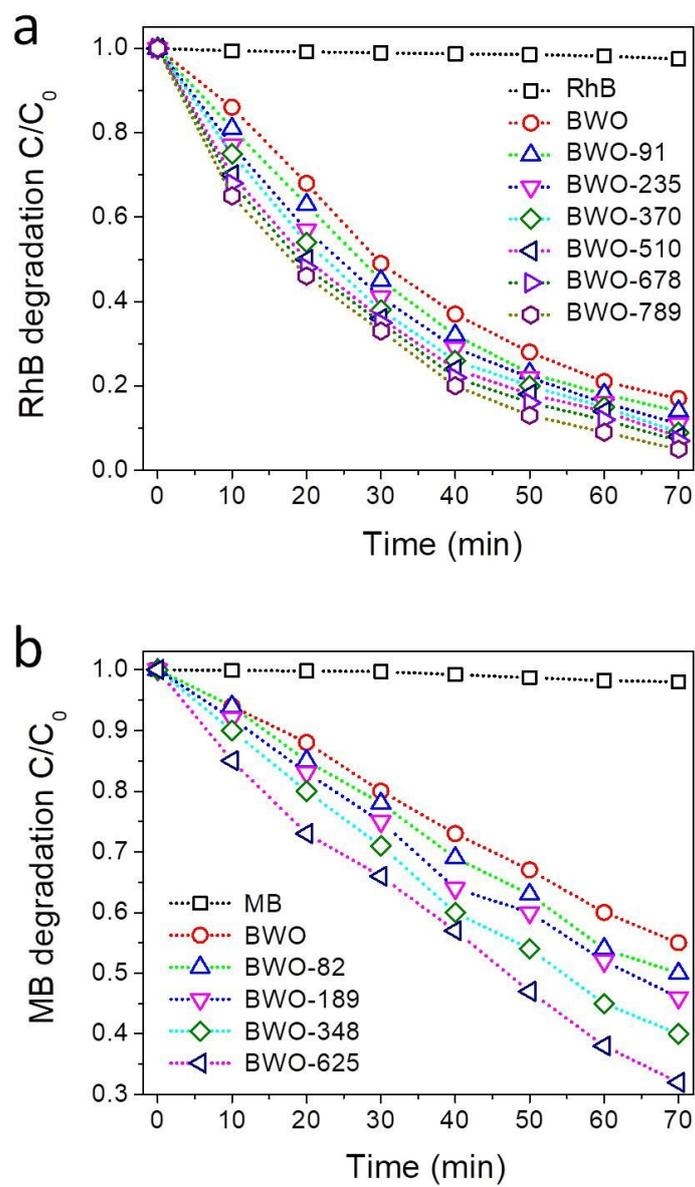
**Figure S10.** Photocatalytic decomposition of RhB (a) and MB (b) with the pristine Bi<sub>2</sub>WO<sub>6</sub> and poled Bi<sub>2</sub>WO<sub>6</sub> after exposing to air for two weeks.
