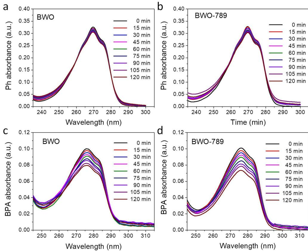
**Figure S7.** The temporal evolutions of all the absorption spectra of the Ph (a,b) and BPA (c,d) solutions (20 ppm) degraded by unpoled and poled  $\text{Bi}_2\text{WO}_6$  under Xe lamp light irradiation.
