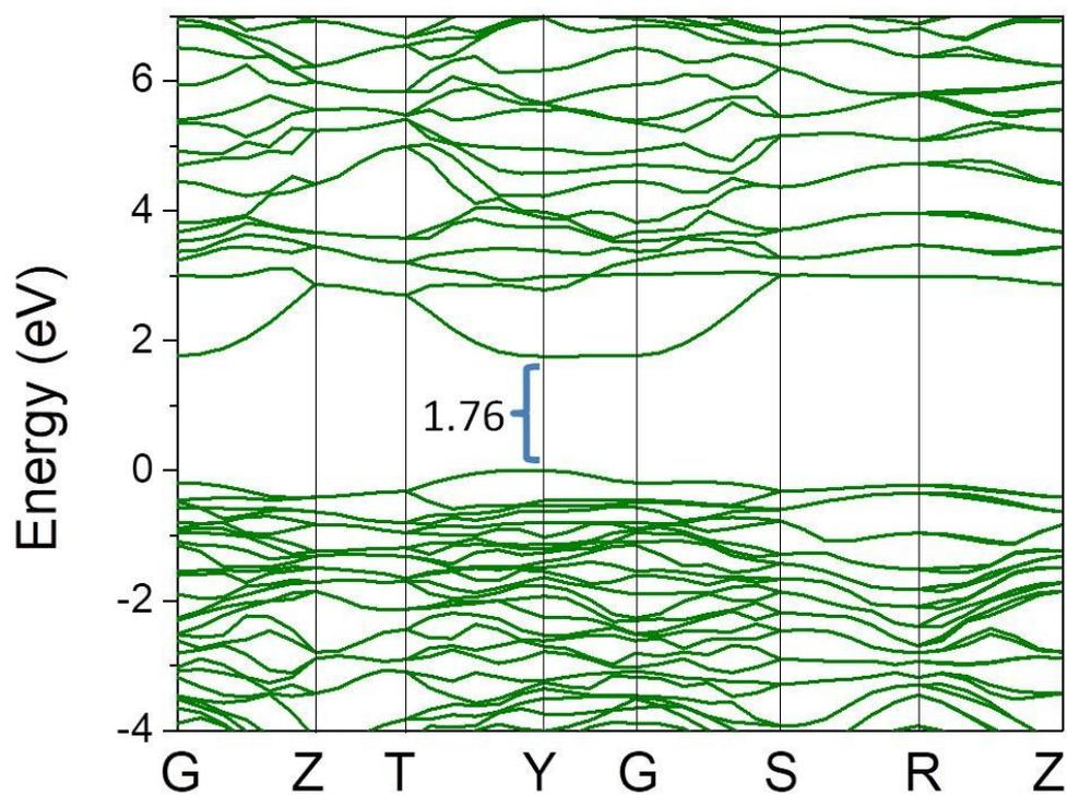
**Figure S13.** Band structure of Bi<sub>2</sub>WO<sub>6</sub> calculated by the DFT method.
