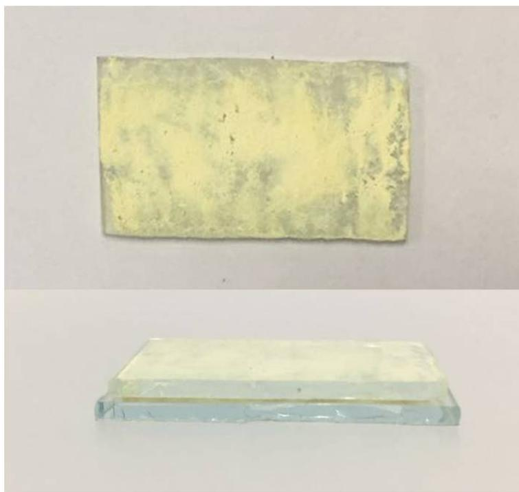
**Figure S1.** The optical photographs of Bi<sub>2</sub>WO<sub>6</sub>/PMMA composite film on the FTO substrate.
