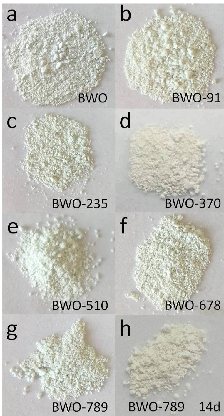
**Figure S3.** The optical photographs of as-grown  $\text{Bi}_2\text{WO}_6$  (a), poled  $\text{Bi}_2\text{WO}_6$  under various electric fields (b-g) and BWO-789 after exposing to air for two weeks (h).
