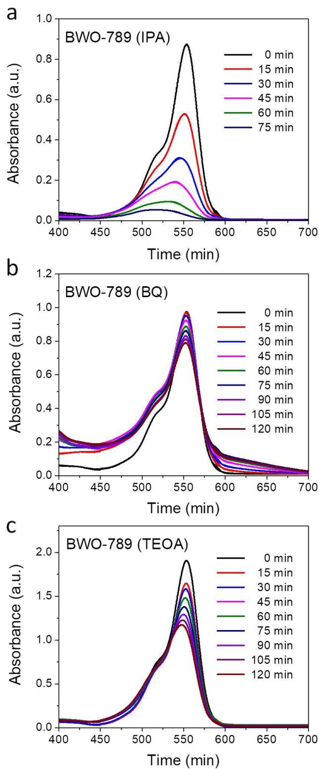
**Figure S12.** The temporal evolutions of all the absorption spectra of the RhB degraded by poled BWO-789 with IPA (a), BQ (b) and TEOA (c) under Xe lamp light irradiation.
