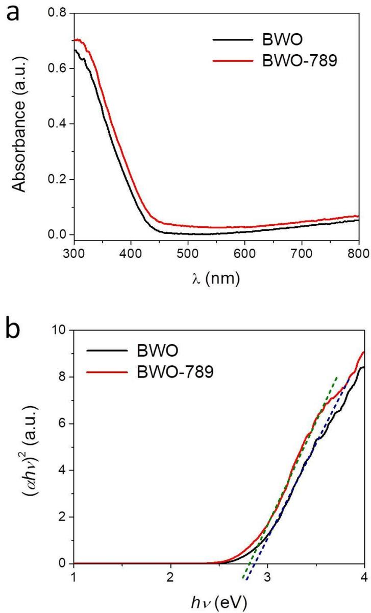
**Figure S4.** UV-vis diffuse reflection spectra (a) and  $(\alpha h\nu)^2$  vs.  $h\nu$  plots (b) of pristine  $\text{Bi}_2\text{WO}_6$  and poled BWO-789.
