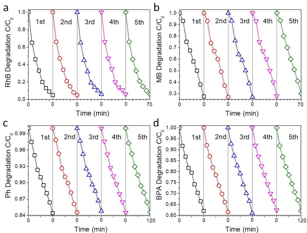
**Figure S8.** Cycling tests of visible-light driven photocatalytic activity of BWO-789 for RhB (a), MB (b), Ph (c) and BPA (d) photodegradations.
