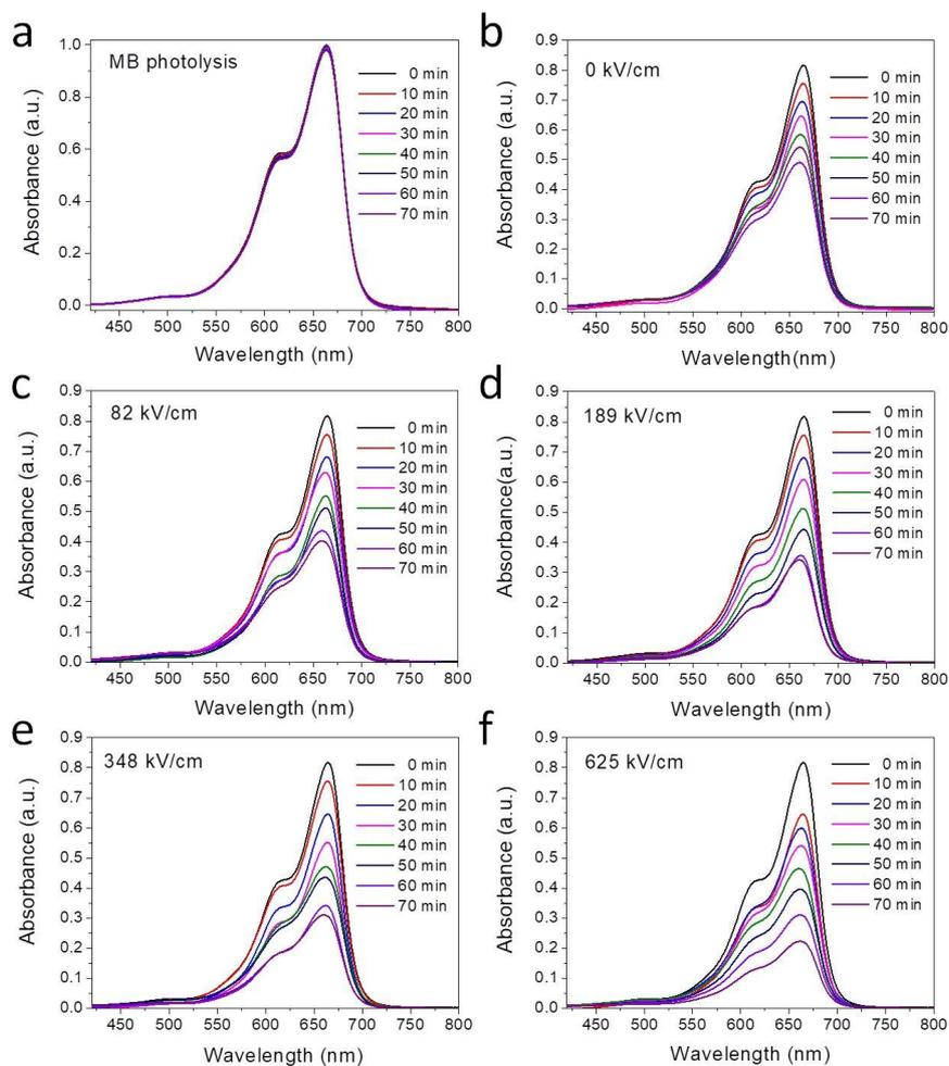
**Figure S6.** The temporal evolutions of all the absorption spectra of the MB solutions ( $10^{-5}$  mol/L) degraded by unpoled and poled  $\text{Bi}_2\text{WO}_6$  under Xe lamp light irradiation.
