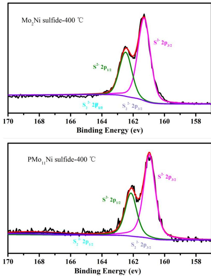
**Fig. S6** Deconvolution of S 2p XPS spectra of  $\text{Mo}_2\text{Ni}$  and  $\text{PMo}_{11}\text{Ni}$  sulfides.
