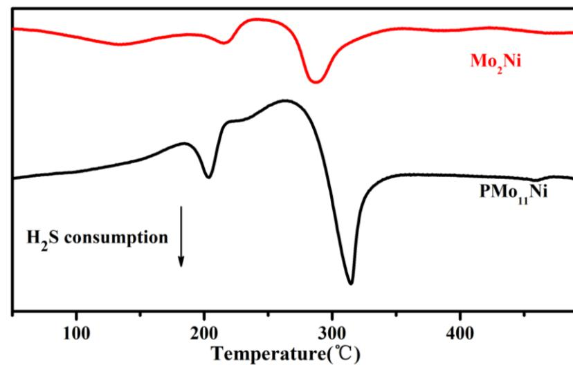
**Fig. S2** TPS profiles of bulk  $Mo_2Ni$  and  $PMo_{11}Ni$ .
