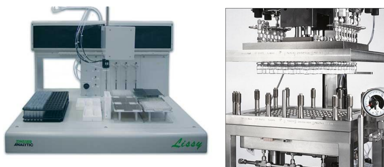
Figure S1: Hardware available at InnoSyn for high throughput screening: a) Liquid handling robot (Zinsser Lissy) and b) Premex 96-Multi Reactor. [1]
