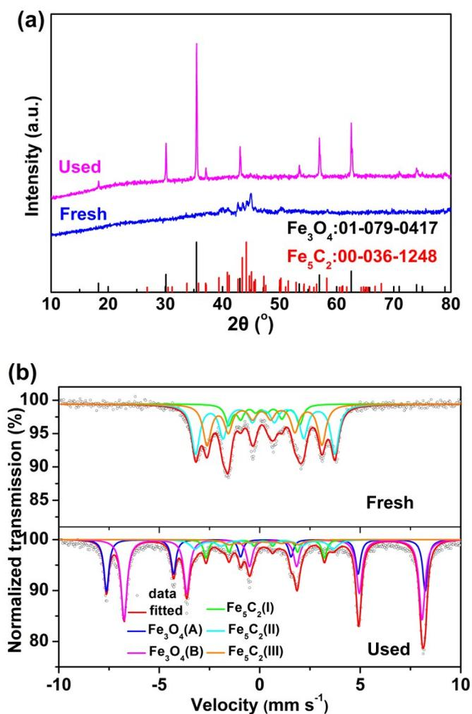
**Fig. S1** XRD patterns (a) and Mössbauer spectra (b) of the fresh and used 1Na/Fe<sub>5</sub>C<sub>2</sub> catalysts.
