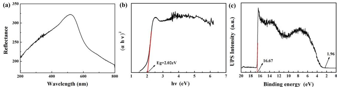
**Fig. S3** (a) UV-vis diffuse reflectance spectrum, (b)  $(\alpha h\nu)^2$  versus  $h\nu$  curve, and (c) UPS spectrum of COP-NT.
