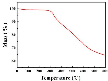
**Fig. S2** TGA curves of COP-NT.
