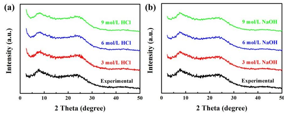
**Fig. S1** The PXRD patterns of COP-NT under different conditions.
