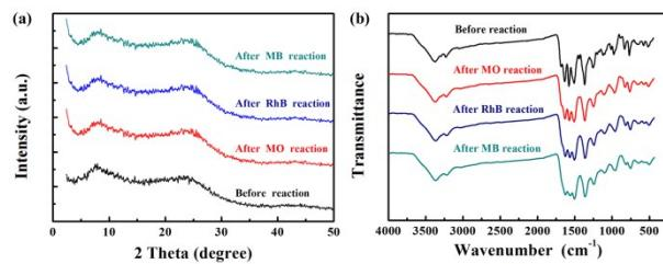
**Fig. S7** (a) PXRD patterns and (b) FT-IR spectra of COP-NT before and after reaction.
