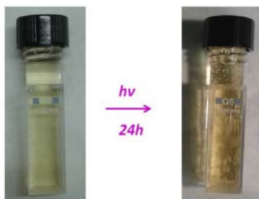
Fig. S1 Crystallization of the trans photodimer, DMAMA, after irradiation at \lambda = 365 nm of a saturated ethanolic solution.
