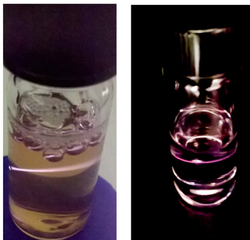
Figure S3. Digital photographs of alendronate-coated \text{NaYF}_4:\text{Nd}^{3+}/\text{Yb}^{3+}/\text{Er}^{3+} (1/20/2%)@ \text{NaYF}_4:\text{Nd}^{3+} (25%) core-shell UCNPs in fetal bovine serum (left) and in PBS buffer (right) after laser excitation at \lambda = 793 nm (cw diode laser, power output 100 mW).
