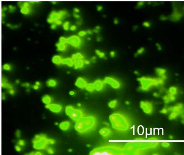
**Figure S6** A typical fluorescence image of CsPbBr<sub>3</sub> particles.
