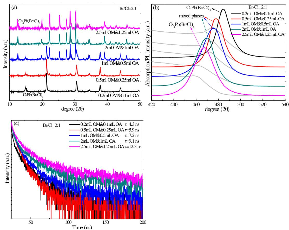
**Figure S4** (a) XRD patterns, (b) PL/Absorption spectra and (c) time-resolved fluorescence decay curves of the synthesized products obtained by using different amounts of OA and OM surfactants, transforming from 3D perovskite  $\text{CsPb}(\text{Br/Cl})_3$  to 0D perovskite-related  $\text{Cs}_4\text{Pb}(\text{Br/Cl})_6$  with Br/Cl ratio of 2:1.
