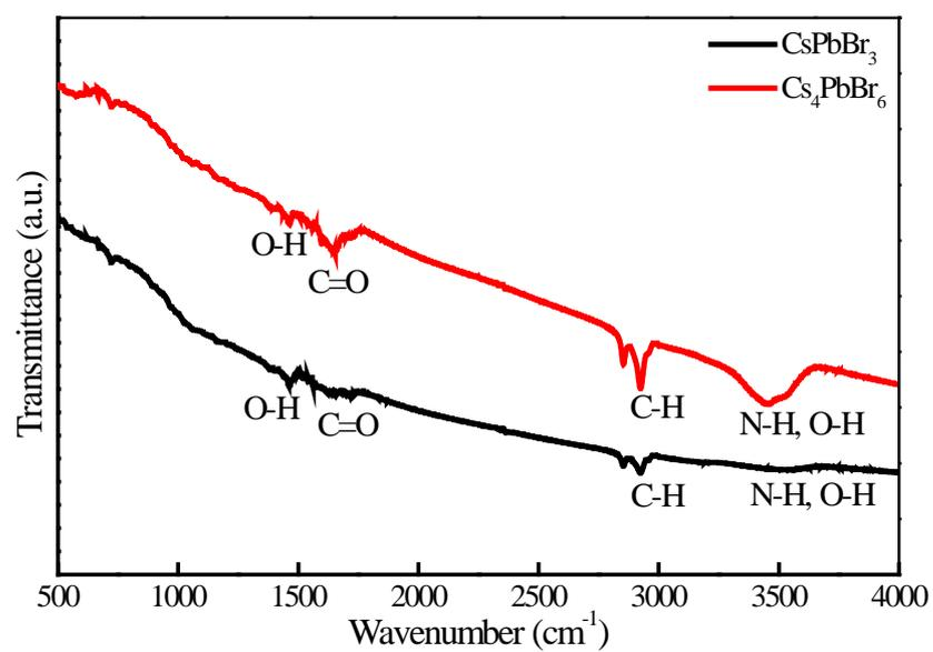
**Figure S5** FTIR spectra of the as-prepared CsPbBr<sub>3</sub> and Cs<sub>4</sub>PbBr<sub>6</sub> samples, showing the presence of COOH and NH<sub>2</sub> groups on the surfaces of CsPbBr<sub>3</sub> and Cs<sub>4</sub>PbBr<sub>6</sub> particles.
