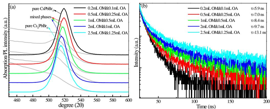
**Figure S2** (a) PL/Absorption spectra and (b) time-resolved fluorescence decay curves of the synthesized products obtained by using different amounts of OA and OM surfactants, transforming from 3D perovskite CsPbBr<sub>3</sub> to 0D perovskite-related Cs<sub>4</sub>PbBr<sub>6</sub>.
