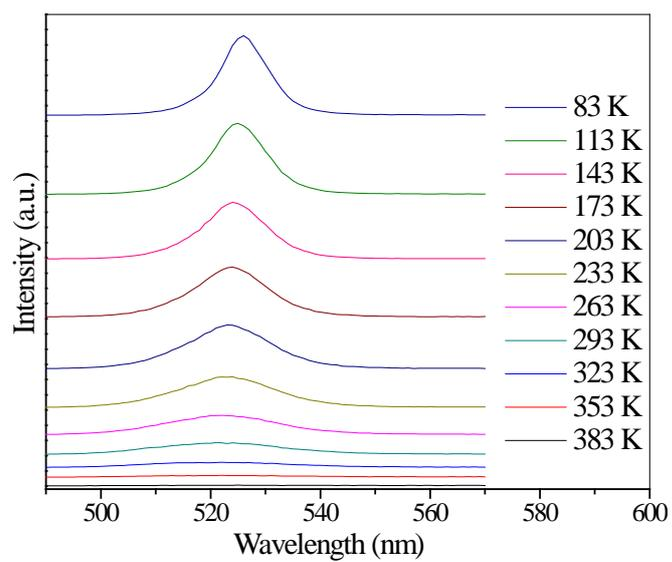
**Figure S3** Temperature-dependent emission spectra of Cs<sub>4</sub>PbBr<sub>6</sub> product.
