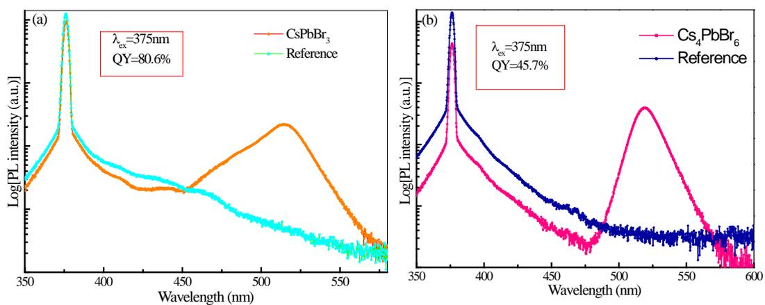
**Figure S1** Quantitative excitation and emission spectra ( $\lambda_{ex}=375\text{ nm}$ ) of (a) CsPbBr<sub>3</sub> sample and (b) Cs<sub>4</sub>PbBr<sub>6</sub> one recorded by a spectrofluorometer equipped with an integrating sphere for quantum yield (QY) measurement.
