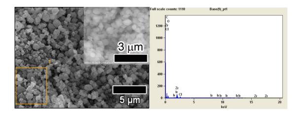
Figure S1. SEM image and EDX analysis of Ir in bpy-UiO $_{30}$ -Ir $_{10}$ .
