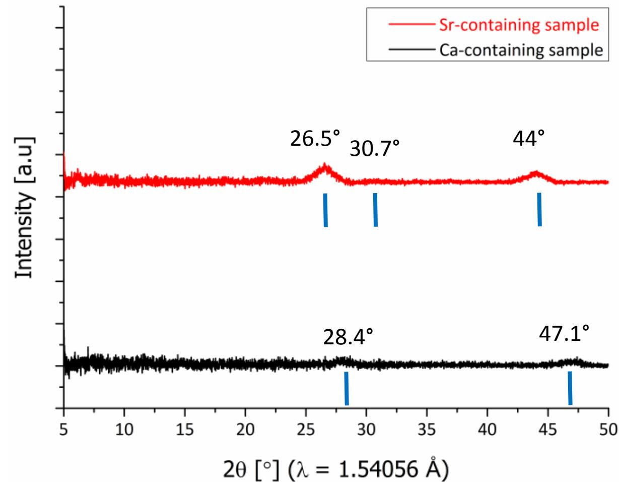
**Figure S3.** PXRD patterns of [Ca(*o*BDC-F<sub>4</sub>)(H<sub>2</sub>O)<sub>2</sub>] (**1**) (black PXRD pattern) and [Sr(*o*BDC-F<sub>4</sub>)(H<sub>2</sub>O)<sub>2</sub>] (red PXRD pattern). (a) samples as-synthesized. (b) Samples after decompositions compared to the standard X-ray lines for CaF<sub>2</sub> from the 00-075-0097 card and SrF<sub>2</sub> from the 00-001-0644 card (blue vertical lines).
