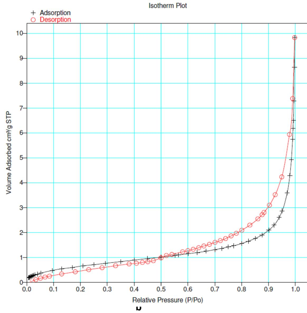
**Figure S8.** Isotherm curves of the compound 2. Adsorption (crosses) and desorption pore volume (circles) isotherm for nitrogen at room temperature (a), at 200 °C (b), 240 (c), 290 °C (d).
