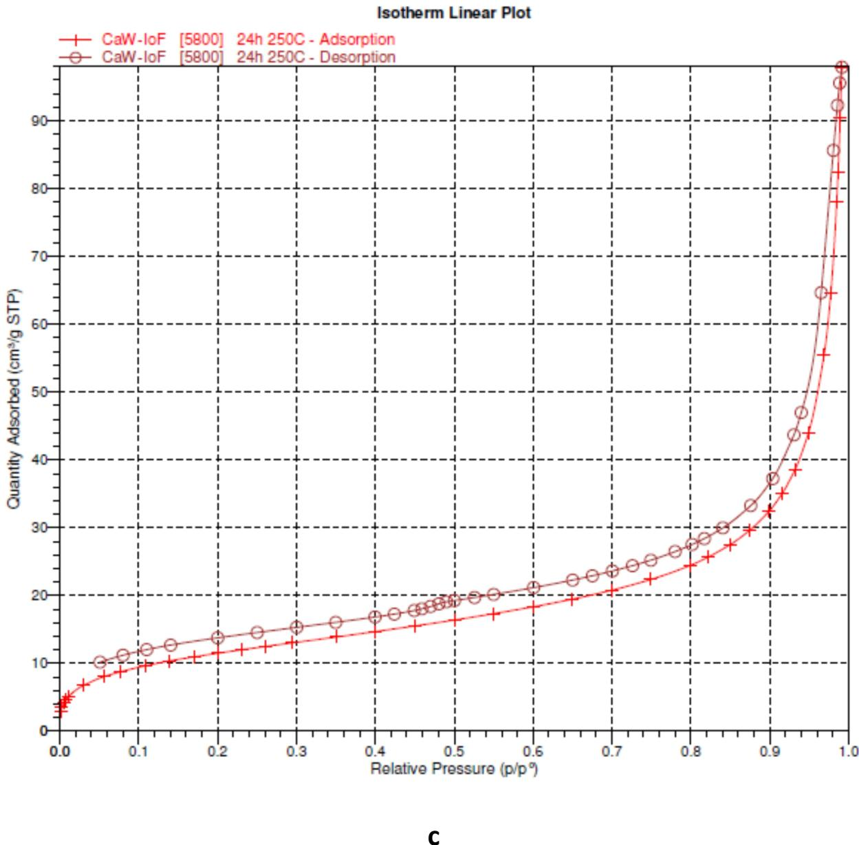
**Figure S7.** Isotherm curves of the compound **1**. Adsorption (crosses) and desorption pore volume (circles) isotherm for nitrogen at room temperature (a), at 200 °C (b), 250 (c).
