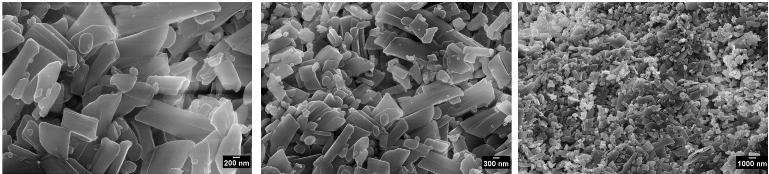
**Figure S9.** SEM images for  $[\text{Ca}(o\text{BDC-F}_4)(\text{H}_2\text{O})_2]$  (**1**).
