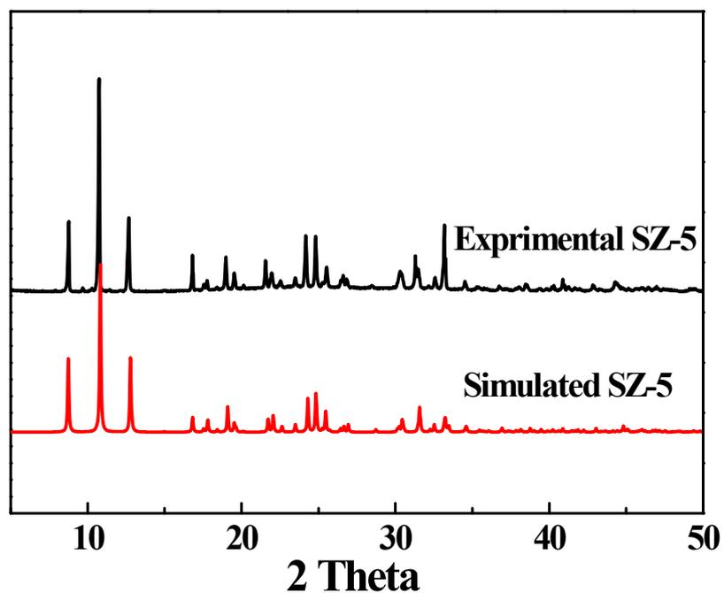
Figure S1. The powder X-ray diffraction (PXRD) for SZ-5
