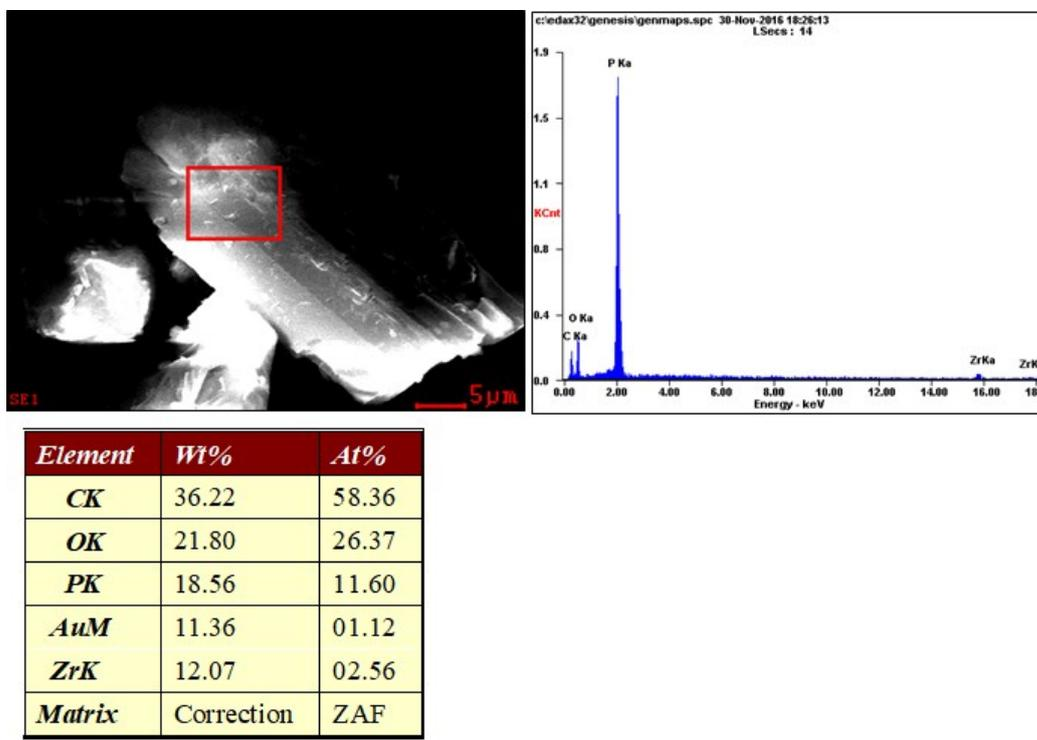
Figure S3. SEM images and EDS data of **SZ-5** before ion-exchange.
