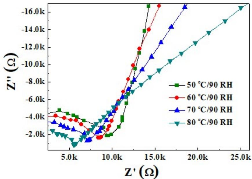
**Figure S6.** Impedance plots of SZ-5 at different temperatures of 40-80 °C under 90% RH.
