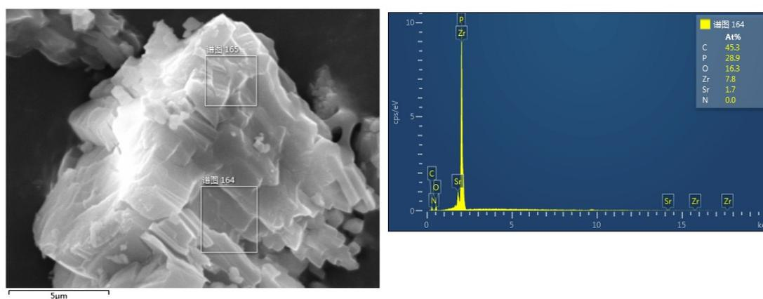
Figure S4. SEM images and EDS data of **SZ-5** after ion-exchange.
