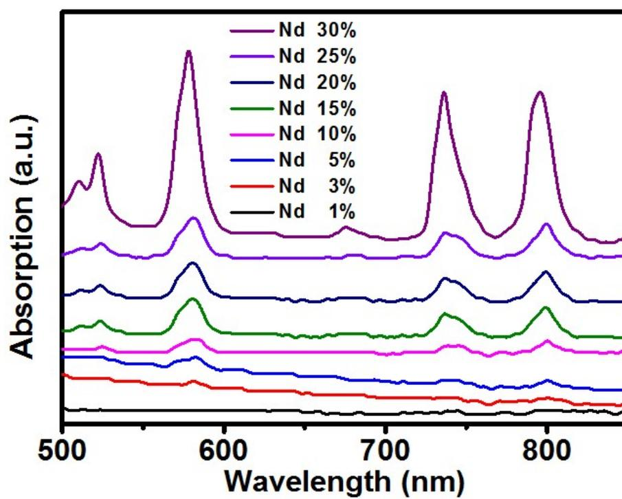
**Figure S6.** Absorption spectra of CaF<sub>2</sub>:Nd samples with different Nd<sup>3+</sup> doping contents.
