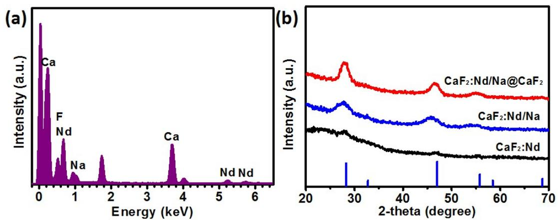
**Figure S2.** (a) EDX pattern of CaF<sub>2</sub>:Nd/Na nanoparticles; (b) XRD patterns of the as-synthesized CaF<sub>2</sub>:Nd, CaF<sub>2</sub>:Nd/Na and CaF<sub>2</sub>:Nd/Na@CaF<sub>2</sub> nanoparticles.
