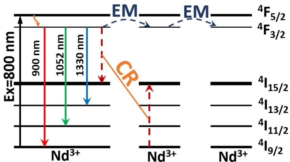
**Figure S5.** Mechanism of generation of the NIR PL emissions upon 800 nm laser irradiation, the cross-relaxation (CR) process and energy migration process (EM) between Nd<sup>3+</sup> ions.
