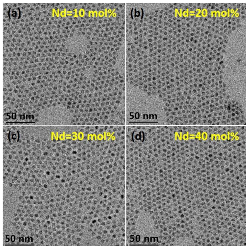
**Figure S1.** TEM images of CaF<sub>2</sub>:Nd/Na nanoparticles with different Nd<sup>3+</sup> doping concentrations.
