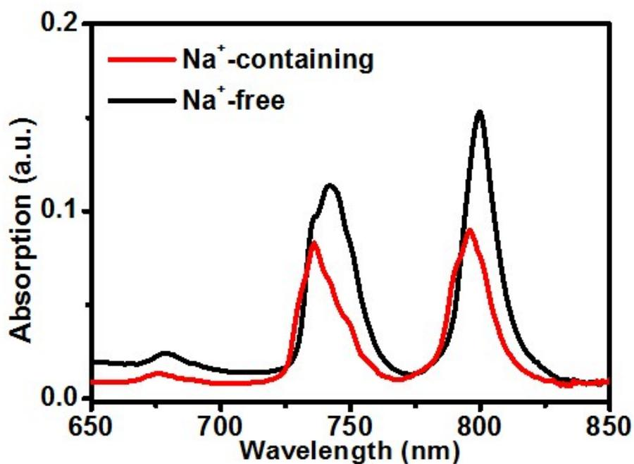
**Figure S3.** Visible - Near-infrared absorption spectra of the  $\text{CaF}_2:\text{Nd}$  samples codoped with and without  $\text{Na}^+$  ions dispersed in cyclohexane ( $0.1 \text{ mmol}\cdot\text{ml}^{-1}$ ). The absorption peak at around 740 nm, 800 nm are the results of the transitions from  $^4\text{I}_{9/2}$  to  $^4\text{F}_{7/2}$ ,  $^4\text{I}_{9/2}$  to  $^4\text{F}_{5/2}$  of  $\text{Nd}^{3+}$  ions, respectively.
