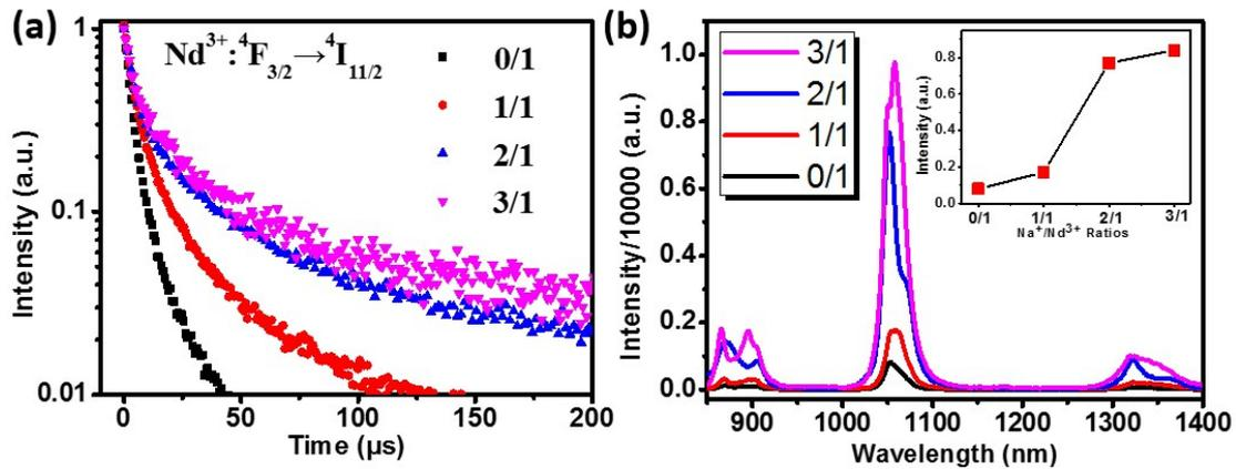
**Figure S4.** (a) Decays of PL emission at 1052 nm in  $\text{CaF}_2:\text{Nd}(10 \text{ mol}\%)/\text{Na}$  nanocrystals doped with different ratios of  $\text{Na}^+/\text{Nd}^{3+}$  under 800 nm laser excitation; (b) NIR PL spectra of  $\text{CaF}_2:\text{Nd}(10 \text{ mol}\%)/\text{Na}$  nanocrystals doped with different ratios of  $\text{Na}^+/\text{Nd}^{3+}$  under 800 nm laser excitation. Inset in (b): PL intensity at 1052 nm as a function of  $\text{Na}^+/\text{Nd}^{3+}$  ratios.
