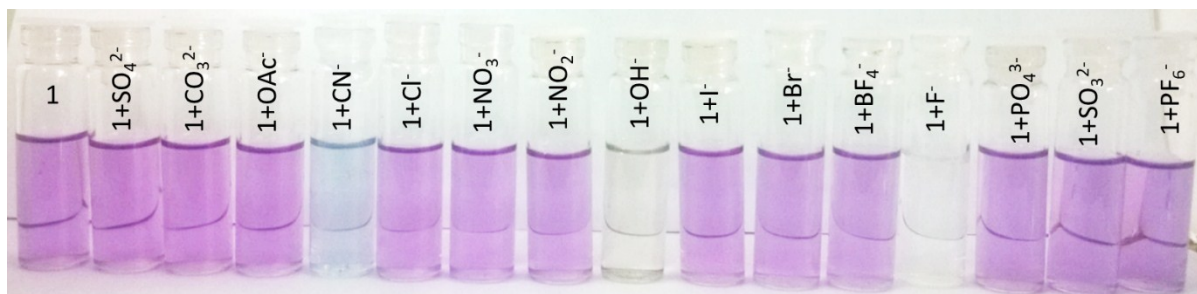
Figure S7. Photograph of 1 ( 10^{-5} M in \text{CH}_3\text{CN} ) and with added analytes. It clearly depicts that only \text{CN}^- , \text{F}^- and \text{OH}^- are able to change the color of 1 while other anions elicited no response.
