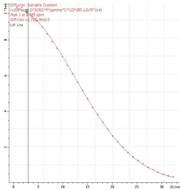
**Figure S10.** *TopSpin* display after fitting with *SimFit* ( $T_1/T_2$  Analysis). The fitting curve for the peak at +6.98 ppm of pure PS in  $CD_2Cl_2$  is shown. The plot is ideal, and the fit is, therefore, reliable.
