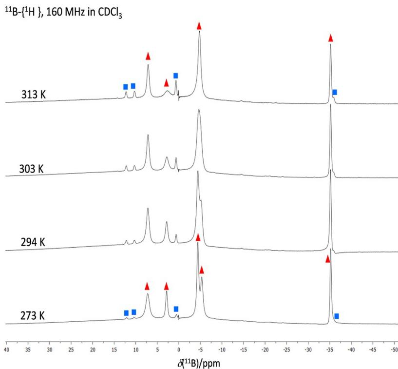
**Figure S4** Variable temperature (VT): 160 MHz  $^{11}\text{B}-\{\text{H}\}$  NMR spectra of salt **1** in  $\text{CDCl}_3$ . The signals of neutral  $\text{B}_{10}\text{H}_{14}$  and anionic  $[\text{B}_{10}\text{H}_{13}]^-$  are highlighted in blue squares and red triangles, respectively.
