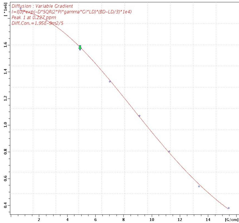
**Figure S12.** *TopSpin* display after fitting with *SimFit* ( $T_1/T_2$  Analysis). The fitting curve for the peak at +0.23 ppm of salt **1** in  $\text{CD}_3\text{CN}$  is shown. The peak corresponds to the polyhedral anion. The plot is not ideal, and the fit is not as reliable as others in this study.
