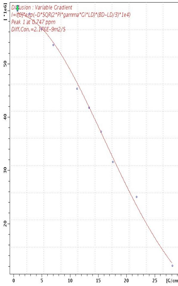
**Figure S15.** *TopSpin* display after fitting with *SimFit* ( $T_1/T_2$  Analysis). The fitting curve for the peak at +0.75 ppm of salt **1** in  $\text{CD}_3\text{CN}$  is shown. This peak corresponds to the polyhedral anion. Plot too short, the fit is not good enough so the value of the diffusion coefficient is not as reliable as the measured for PS in  $\text{CD}_3\text{CN}$ .
