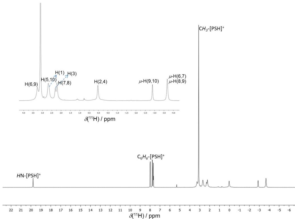
**Figure S2** 500 MHz  $^1\text{H}$ - $\{{}^{11}\text{B}\}$  NMR spectra of salt **1** in  $\text{CD}_2\text{Cl}_2$  at 178 K.
