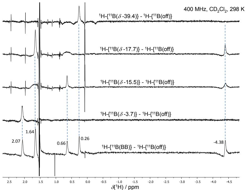
**Figure S7** Subtraction of the off-decoupled spectrum,  $^1\text{H}-\{^{11}\text{B}(\text{off})\}$ , from the Broad Band (BB) decoupled spectrum,  $^1\text{H}-\{^{11}\text{B(BB)}\}$  (bottom trace); and subtractions of the  $^1\text{H}-\{^{11}\text{B}(\text{off})\}$  spectrum from the  $^{11}\text{B}$ -selectively decoupled spectra,  $^1\text{H}-\{^{11}\text{B}(\delta_{\text{B}})\}$  for the pyridine adduct, 6,9-(py)<sub>2</sub>-*arachno*- $\text{B}_{10}\text{H}_{12}$ .
