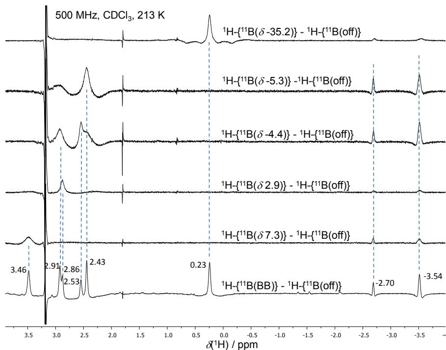
**Figure S5** Subtraction of the off-decoupled spectrum,  $^1\text{H}-\{^{11}\text{B}(\text{off})\}$ , from the Broad Band (BB) decoupled spectrum,  $^1\text{H}-\{^{11}\text{B}(\text{BB})\}$  (bottom trace); and subtractions of the  $^1\text{H}-\{^{11}\text{B}(\text{off})\}$  spectrum from the  $^{11}\text{B}$ -selectively decoupled spectra,  $^1\text{H}-\{^{11}\text{B}(\delta_B)\}$  for compound **1**.
