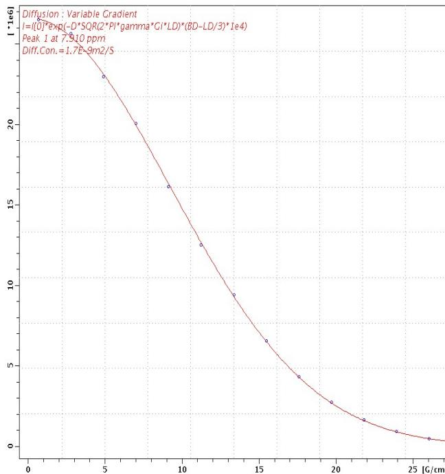
**Figure S13.** *TopSpin* display after fitting with *SimFit* ( $T_1/T_2$  Analysis). The fitting curve for the peak at +7.91 ppm of salt **1** in  $\text{CD}_3\text{CN}$  is shown. The peak corresponds to  $\text{PSH}^+$ . The plot is ideal, and the fit is reliable.
