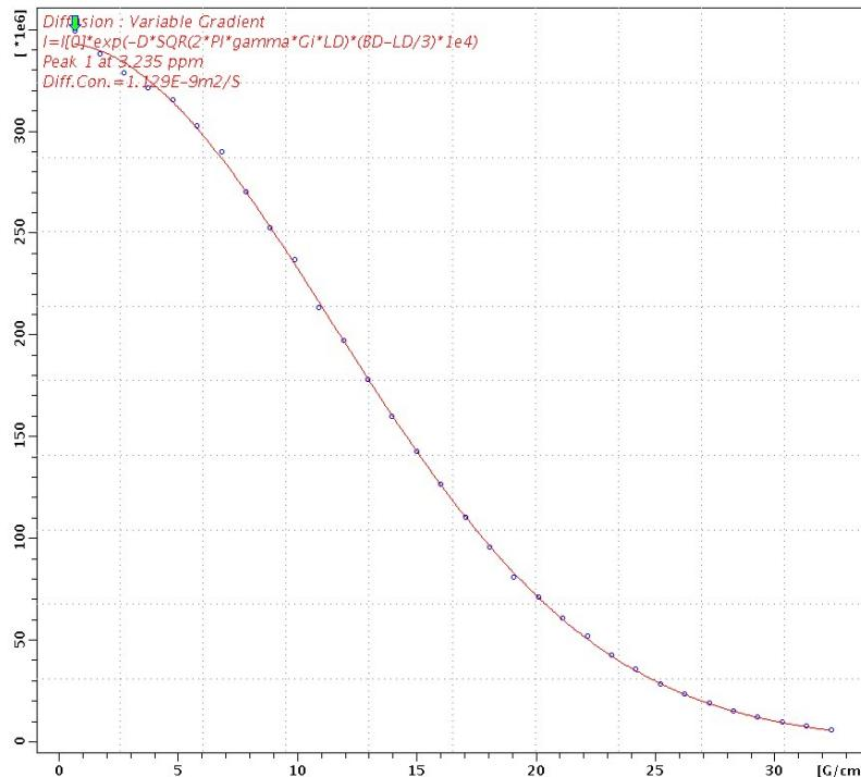
**Figure S8.** *TopSpin* display after fitting with *SimFit* ( $T_1/T_2$  Analysis). The fitting curve for the peak at +3.24 ppm of salt **1** in  $\text{CD}_2\text{Cl}_2$  is shown. The plot is ideal, and the fit is, therefore, reliable. This peak corresponds to the  $[\text{PSH}]^+$  cation.
