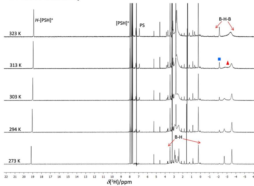
**Figure S3** Variable temperature (VT): 500 MHz  $^1\text{H}$ - $\{{}^{11}\text{B}\}$  NMR spectra of salt **1** in  $\text{CDCl}_3$ . The signals of neutral  $\text{B}_{10}\text{H}_{14}$  and anionic  $[\text{B}_{10}\text{H}_{13}]^-$  are highlighted in blue squares and red triangles, respectively.
