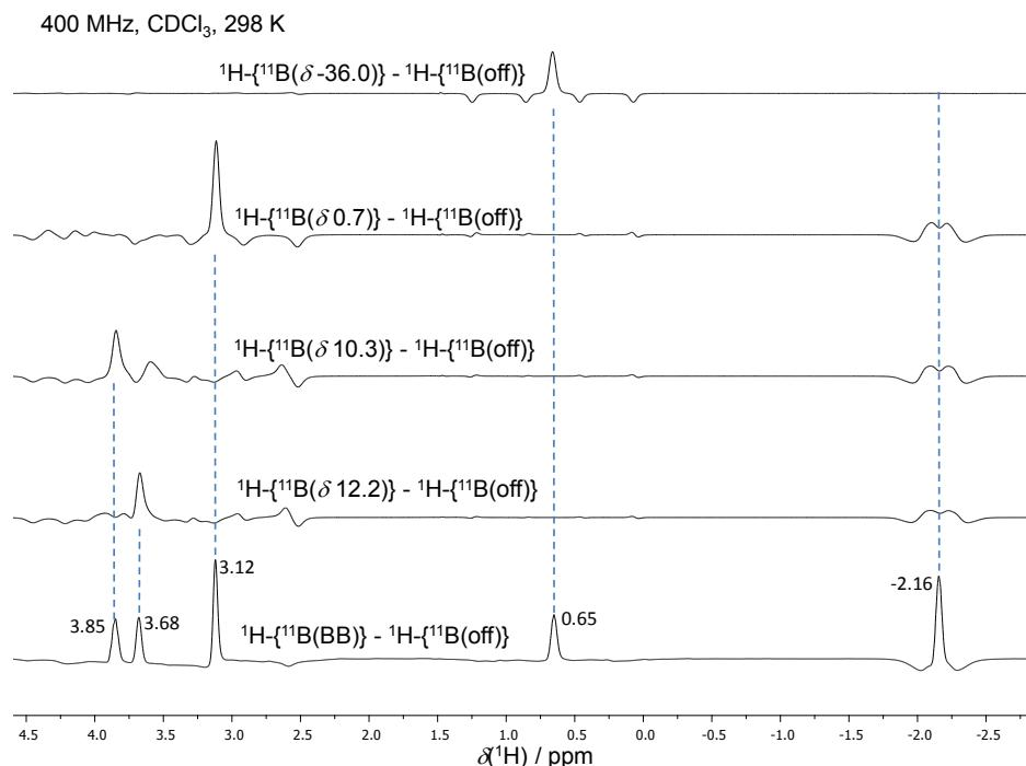
**Figure S6** Subtraction of the off-decoupled spectrum,  $^1\text{H}-\{^{11}\text{B}(\text{off})\}$ , from the Broad Band (BB) decoupled spectrum,  $^1\text{H}-\{^{11}\text{B}(\text{BB})\}$  (bottom trace); and subtractions of the
