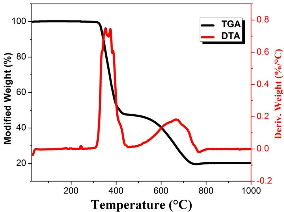
Fig. S4 TG and DTA curve of 2
