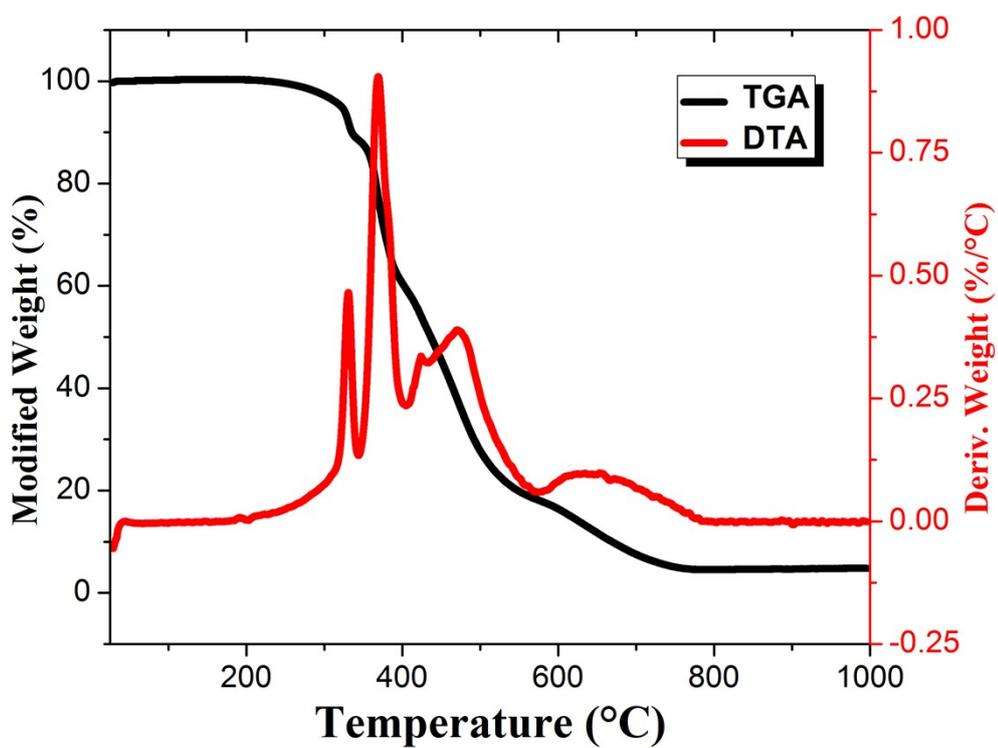
Fig. S3 TG and DTA curve of 1
