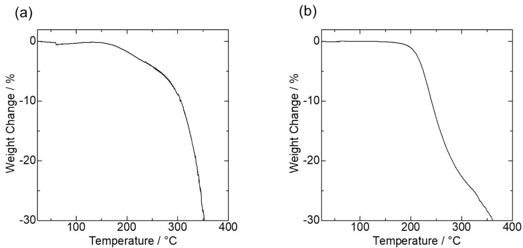
Fig. S1. TG curves of (a) **2** and (b) **3**. (The measurements were carried out under Ar atmosphere with scan rate of  $5^\circ \text{ min}^{-1}$ )
