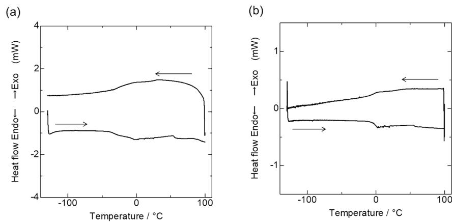
Fig. S2. DSC curves of (a) **2** and (b) **3** (first cooling scan and second heating scan, scan rate =  $5^\circ \text{ min}^{-1}$ ).
