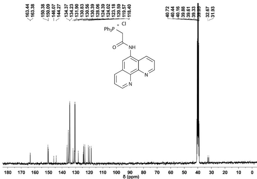
Fig. S2  $^{13}\text{C-NMR}$  spectrum of LPT1 in  $\text{DMSO-d}_6$ , 300 MHz.
