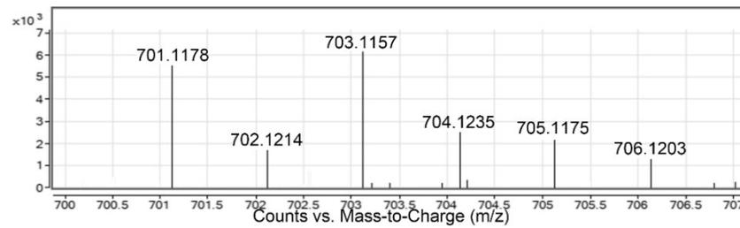
**Fig. S15** High resolution ESI mass spectrum of CPT6.
