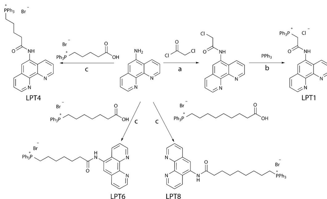
**Scheme S1** Synthetic routes to ligands. (a) Et<sub>3</sub>N, DCM, N<sub>2</sub>, RT; (b) K<sub>2</sub>CO<sub>3</sub>, CH<sub>3</sub>CN, N<sub>2</sub>, 90 °C; (c) EDCI, DMAP, DCM, RT.
