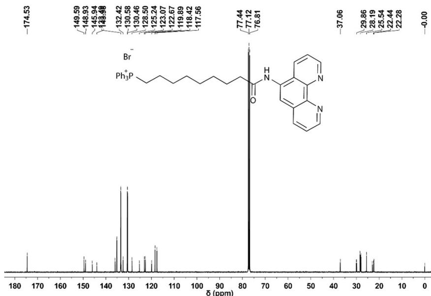
**Fig. S11**  $^{13}\text{C-NMR}$  spectrum of LPT8 in  $\text{CDCl}_3\text{-d}_6$ , 400 MHz.
