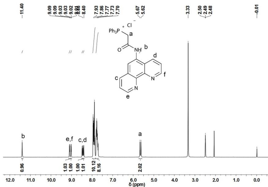
**Fig. S1** <sup>1</sup>H-NMR spectrum of LPT1 in DMSO-d<sub>6</sub>, 300 MHz.
