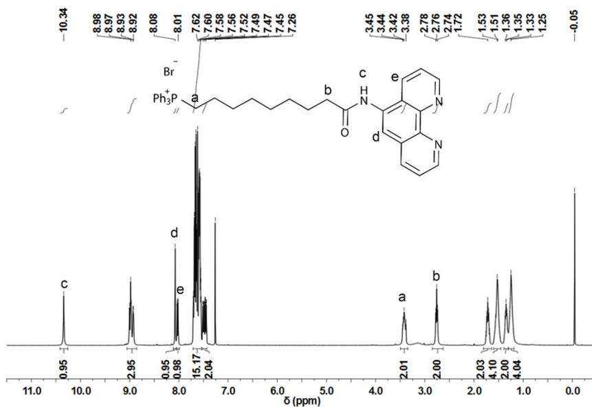
**Fig. S10**  $^1\text{H-NMR}$  spectrum of LPT8 in  $\text{CDCl}_3\text{-d}_6$ , 400 MHz.
