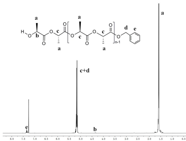
Fig. S4 ^1\text{H} NMR spectrum of PLLA-50 catalyzed by [\text{Mg}(\text{L}^1)_2] (7) in the presence of BnOH.
